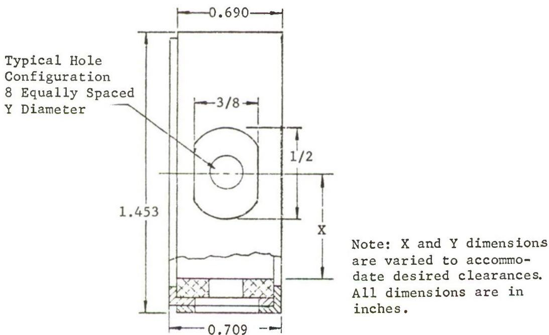
Figure 6. Solid Lubricant Retainer Geometry
