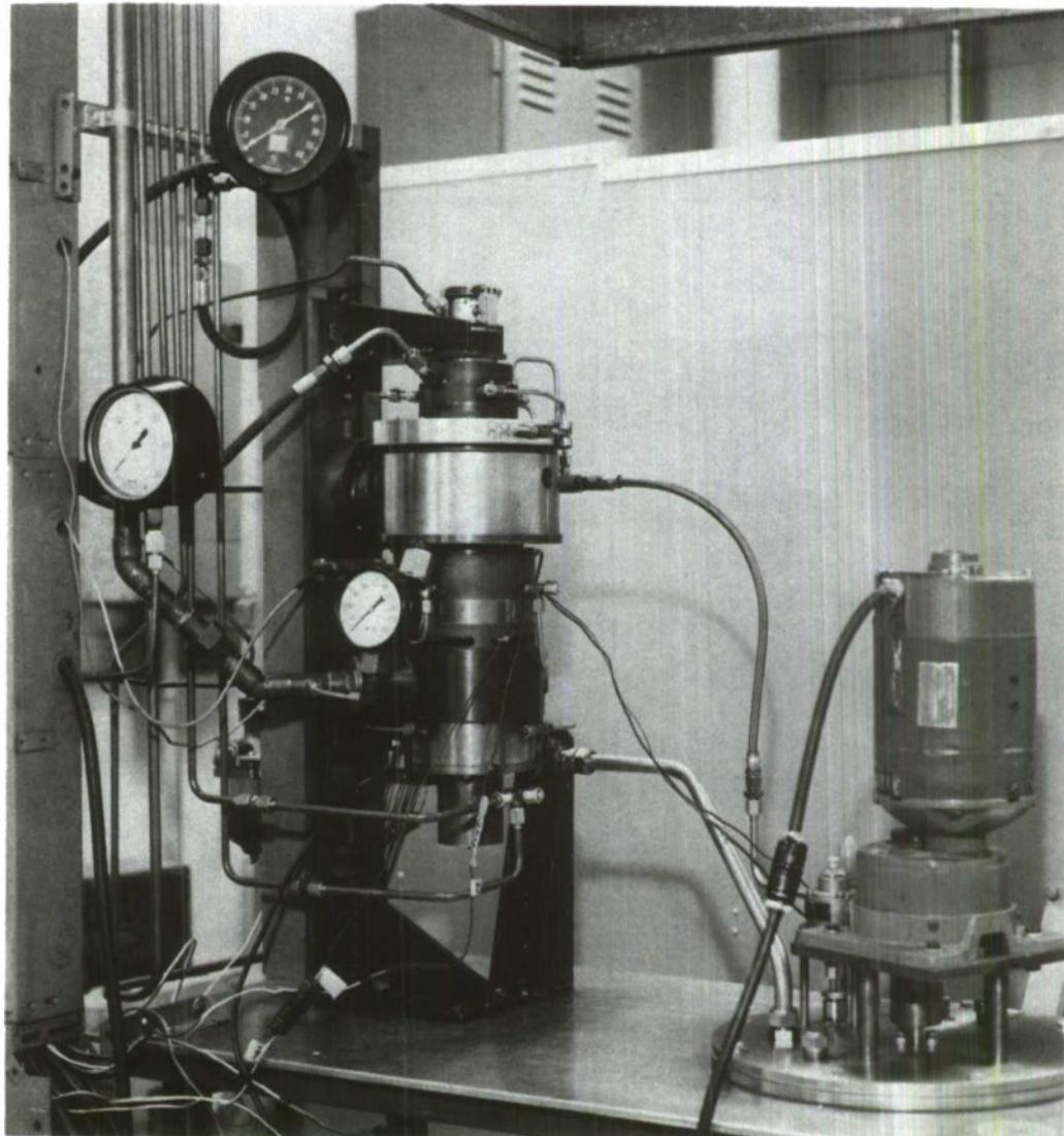
Figure 2. Solid Lube Bearing Test Facility Rig
