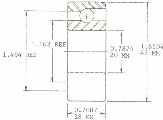
Figure 4. Basic 204 Size Test Bearing Geometry
