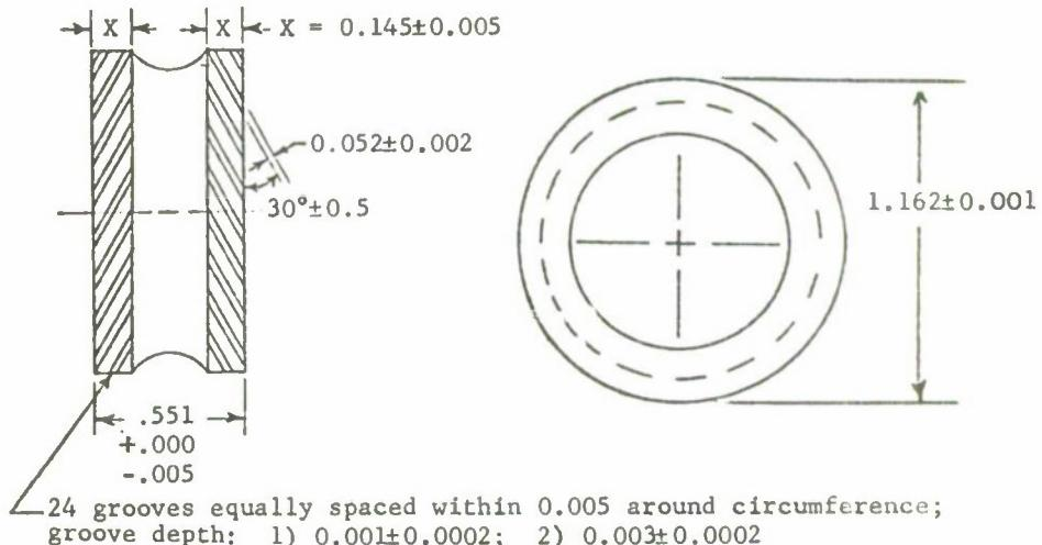
Figure 5. Detailed Drawing of Grooved Bearing
