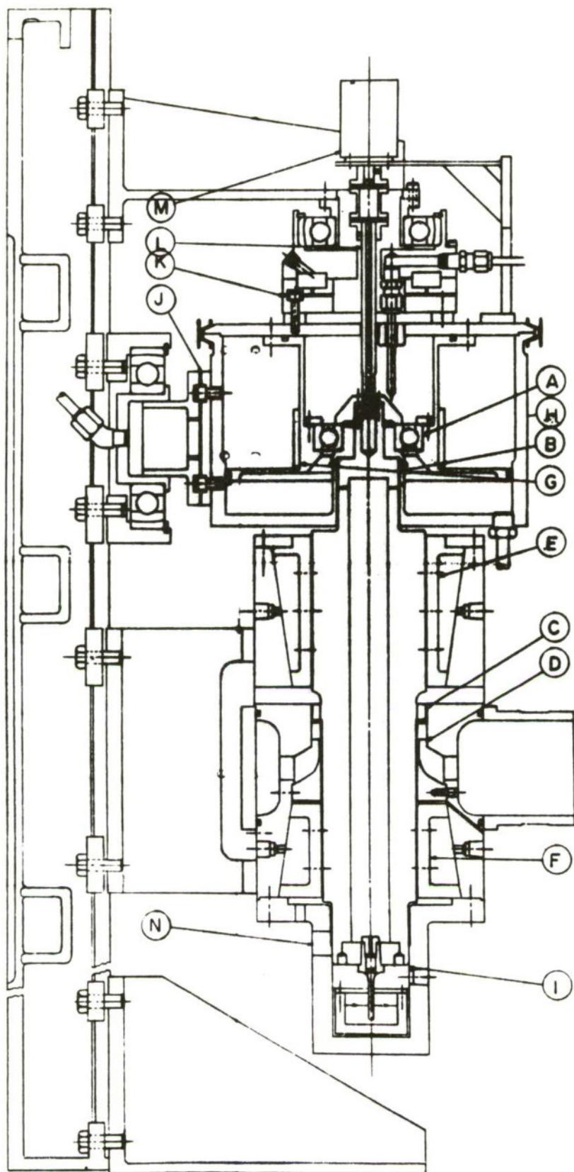
Figure 3. Schematic of Rolling Element Bearing Test Rig
