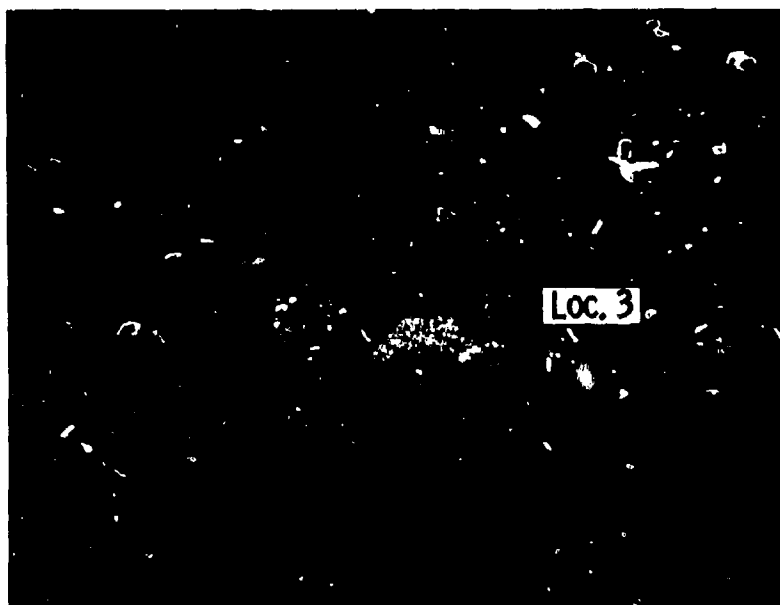
Figure 3-7b Fracture Surface of Cast CaF 2 Sample. SEM 100X
