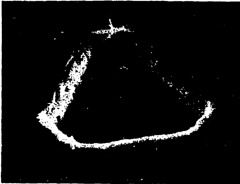
Fig. 3-27d Scattering Center at Surface in Cast \text{CaF}_2 . SEM 5000 \times .
