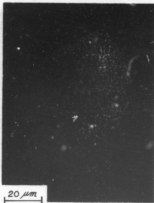
Figure B-11. Photomicrograph taken slightly out of focus to emphasize small subgrains. Pure KBr forged at 21°C and 4660 psi.
