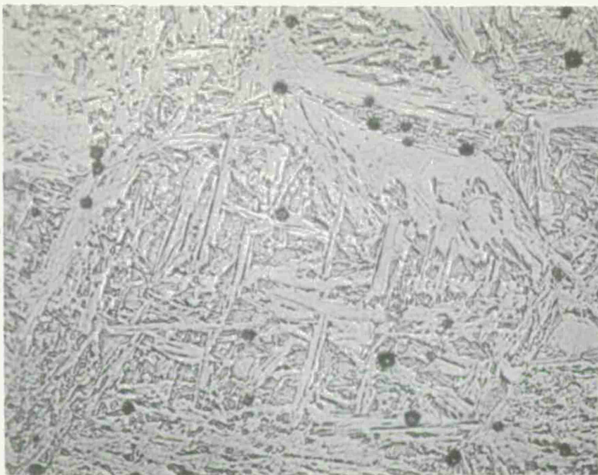
Figure 7. 78 w/o Co-22 w/o Fe Alloy Annealed at 1000°C Air Cooled to 25°C. Etched in 5% Nital. Photomicrograph Shows Structure of BCC Phase (X1000).
