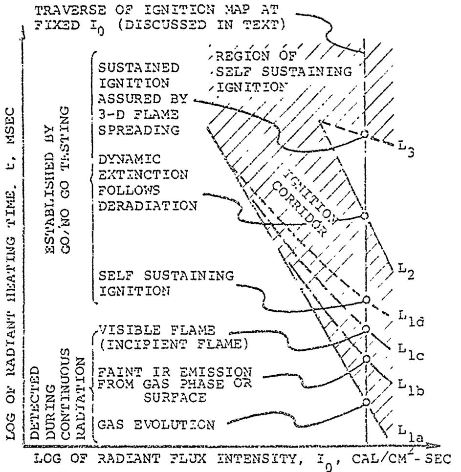
Fig. 1 Generalized ignition map showing event limits or signals that occur during radiant heating of solid propellants.
