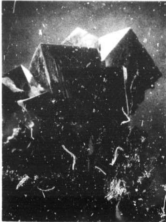
Figure 2.  $\text{PrB}_6$  deposit containing 1 mm cubes, gold wire substrate. ( $\sim 50\times$ )
