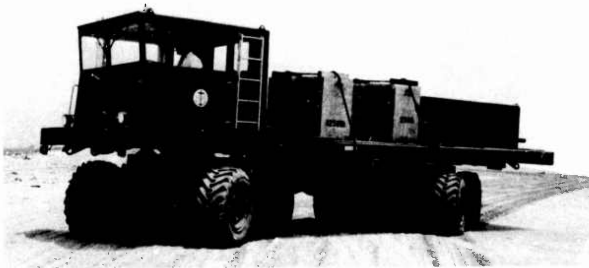
Figure 7. Operating vehicle on beach sand for Terra-Grip tire performance and frame modification tests.
