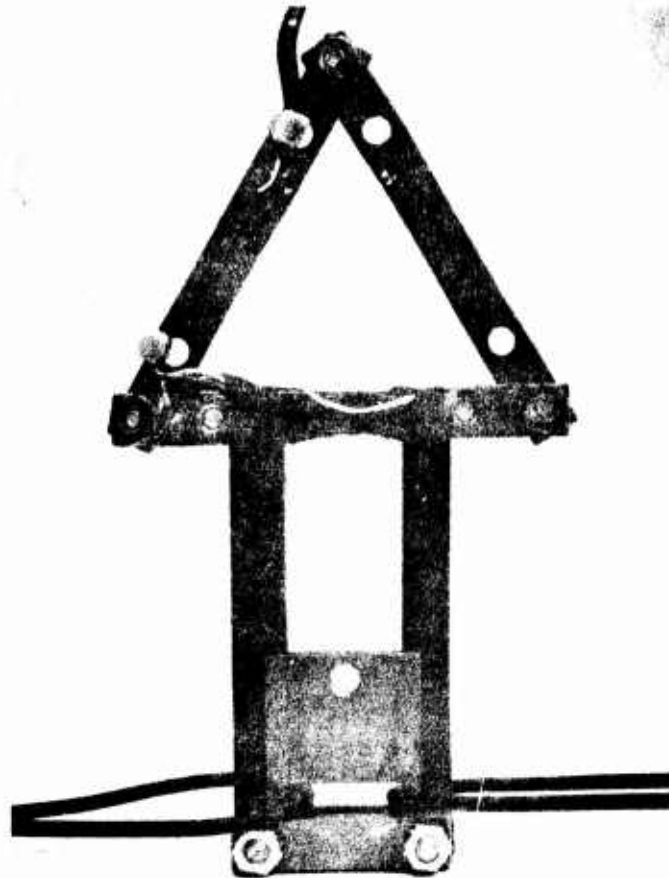
Figure 8. Mechanical gage modified to produce an electrical signal proportional to force.
