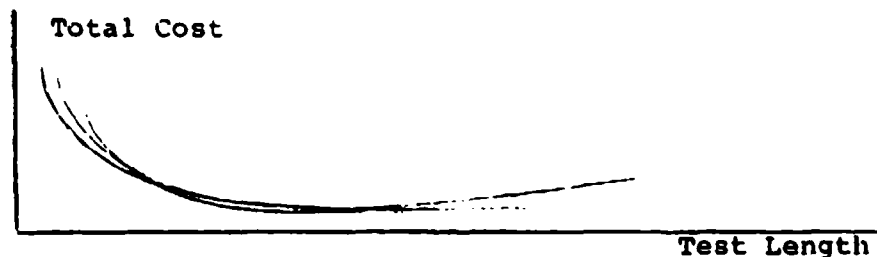
Figure 27. Total Cost by Test Length for Several Assumed Values of True LSC (Hypothetical).
