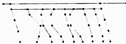
FIGURE 4b MODE SHAPE NO. 2 FREQUENCY 8.640 Hz
