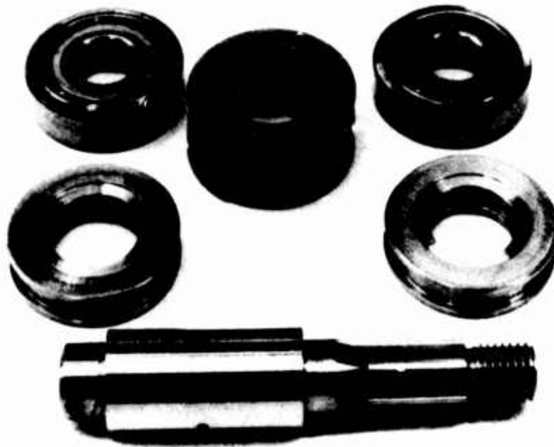
Figure 116. Clutch Components After 40-hr Overrunning at 65,000 rpm
