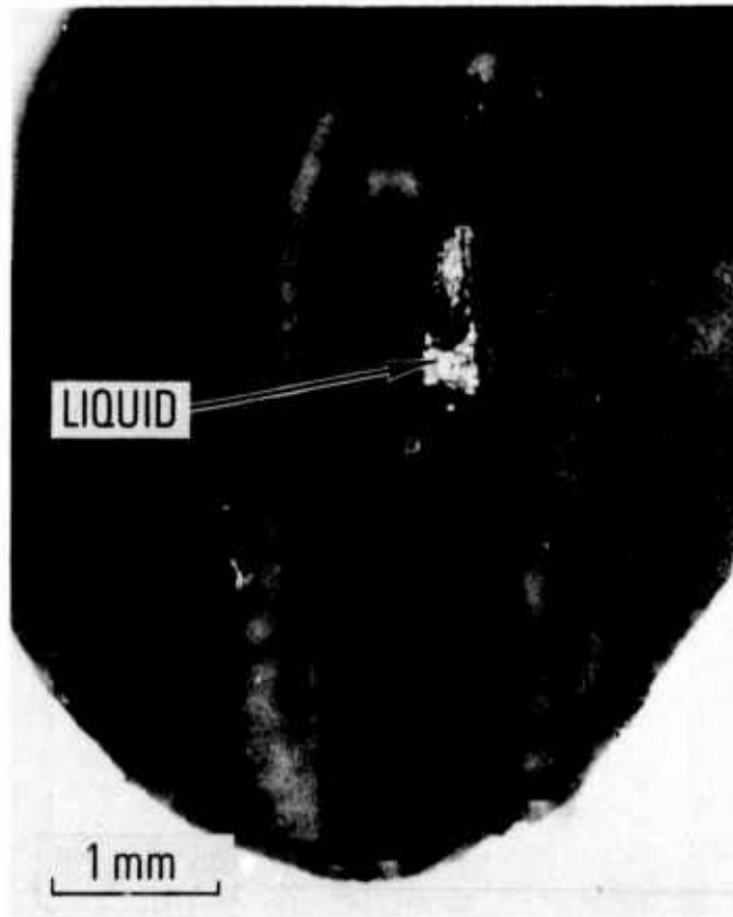
Fig. 8. Same as Fig. 7. (Photomicrograph with ordinary light. Note that liquid is very shiny and unaltered graphite is very dull dark gray.)
