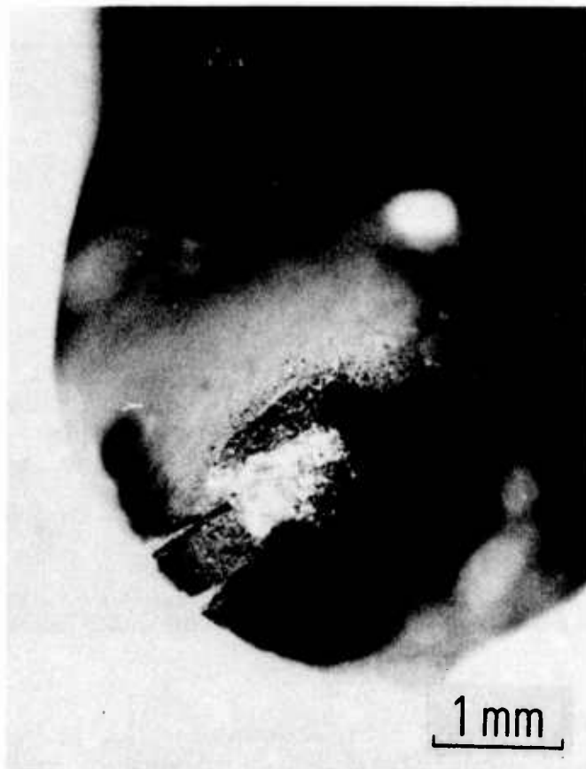
Fig. 11. Sample No. 11 at 4475 K and 160 atm of neon. (Photomicrograph with ordinary light. Liquid is at lower left.)
