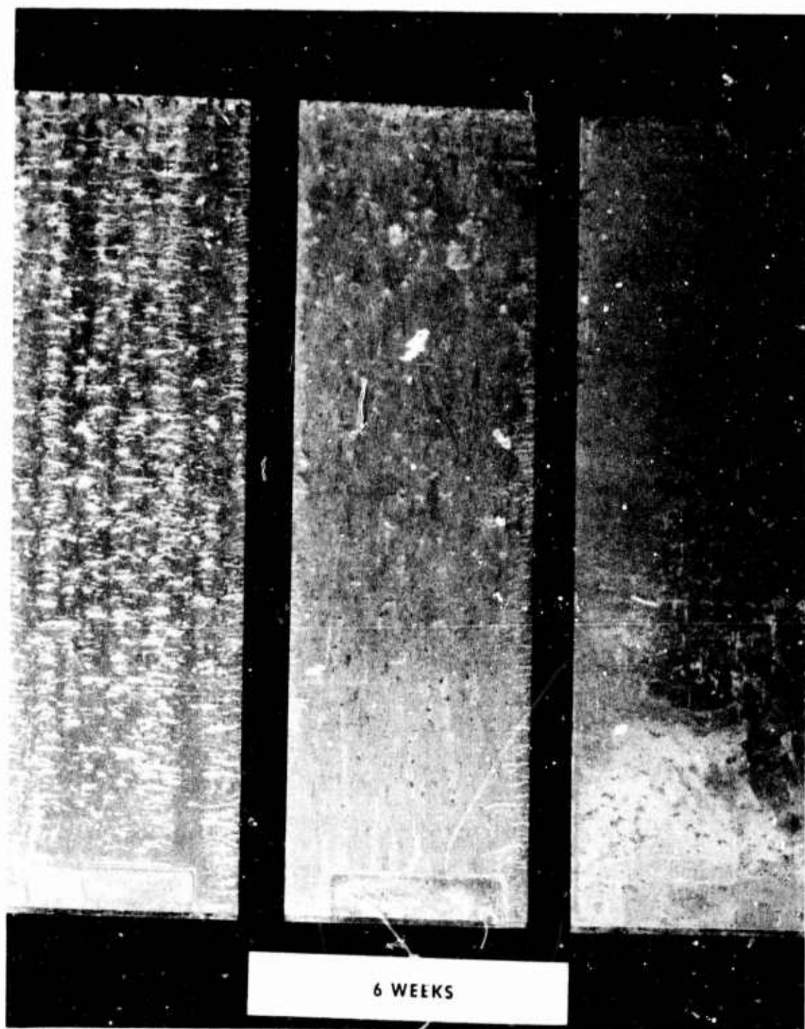
Figure 15. 6 weeks in NaCl-SO 2 salt spray.
