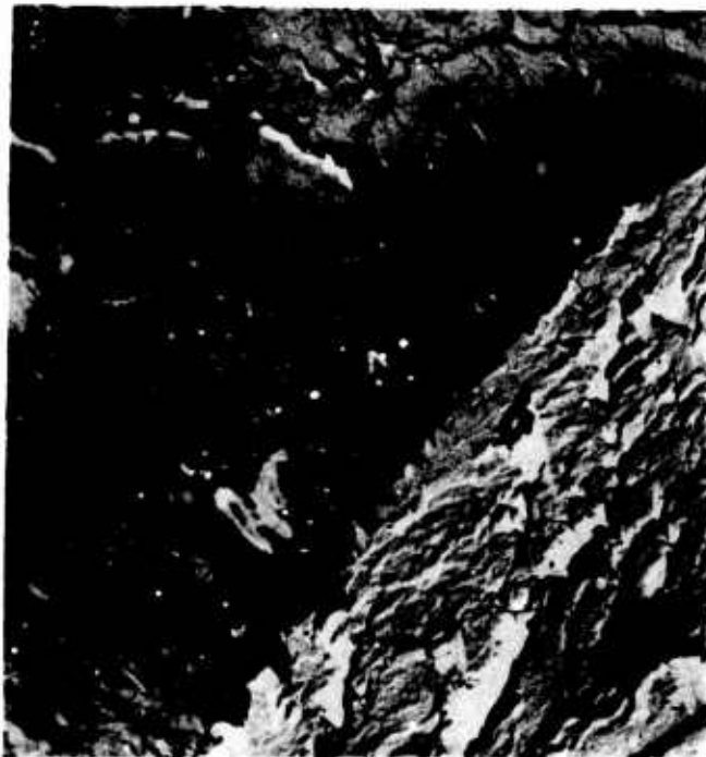
Figure 10. Fracture topology of Ti-38-6-44 of the SCC and rapid fracture zones for specimen failed in \text{CH}_3\text{OH} . Mag. 4,600X
