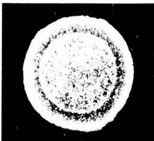
Fig. 7 L-605 Wire, Exposed to \text{NH}_3 at 1500^\circ\text{F} for 5000 min
