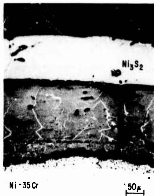
Fig. 1. Ni-35Cr alloy treated at 850^\circ\text{C} with a 10\%\text{H}_2\text{S}-\text{H}_2 gas mixture for 2\frac{1}{2} hours. The scale consists of an outer layer of nickel sulfide which was molten at temperature, and an inner layer of chromium sulfide.
