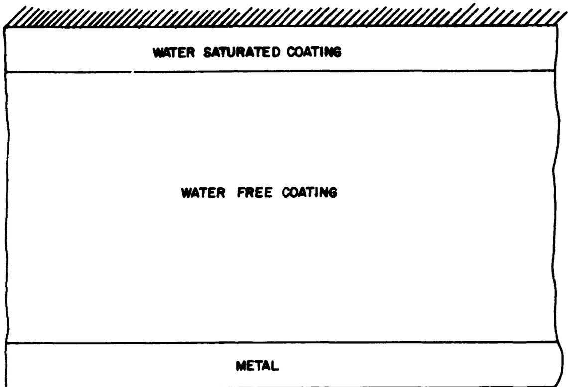
FIGURE A-1 - WATER PENETRATION MODEL CELL
