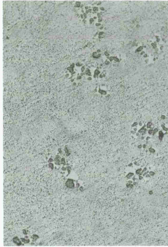
Figure 7. Photomicrographs of Sn-35wt%Pb slurries showing increasing fraction solid; equivalent cooling rate 100°C/min.; (a) g_s = .06 , (b) g_s = .15 , (c) g_s = .60 , 100X.
