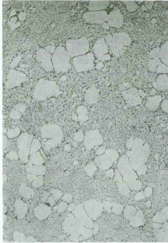
Figure 5. Photomicrographs of Sn-15wt%Pb alloy slurries at various volume fraction solid with slow cooling rates; (a) g_S = .11 , \epsilon = 39^\circ\text{C}/\text{min.} , (b) g_S = .39 , \epsilon = 31^\circ\text{C}/\text{min.} , (c) g_S = .51 , \epsilon = 23^\circ\text{C}/\text{min.} ; 100X.
