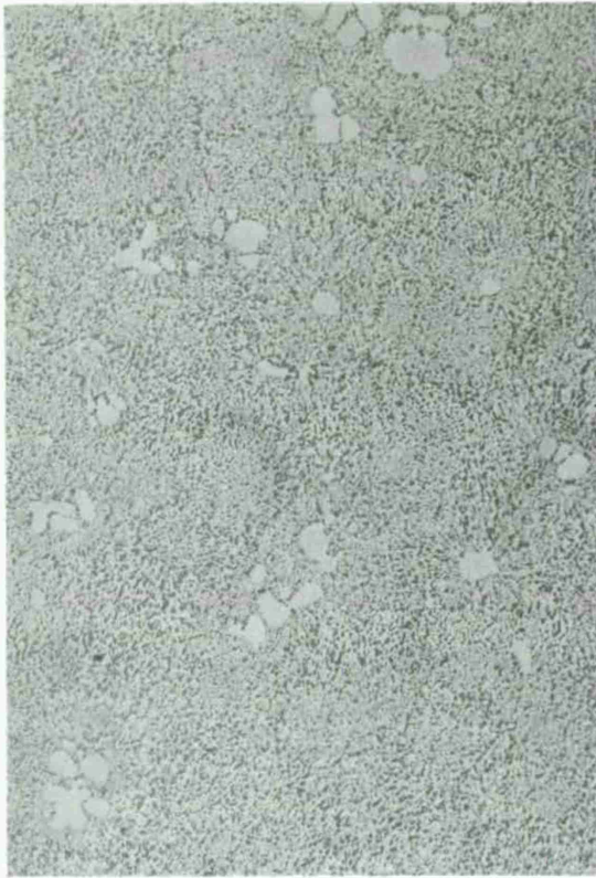
Figure 7. Photomicrographs of Sn-35wt%Pb slurries showing increasing fraction solid; equivalent cooling rate 100°C/min.; (a) g_s = .06 , (b) g_s = .15 , (c) g_s = .60 , 100X.
