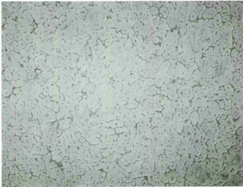
Figure 7. Microstructures of continuously produced semi-solid alloys. Samples were slowly cooled. Top: microstructure of HS 31 superalloy. Bottom: microstructure of M-2 tool steel, 50X.
