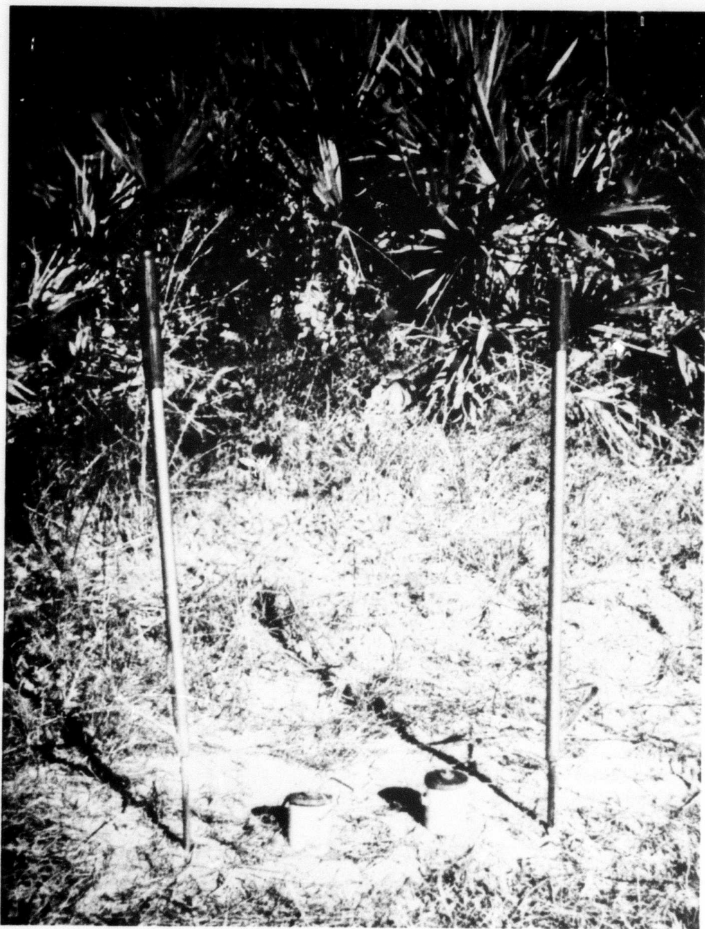
FIGURE 6. METAL CURRENT ELECTRODES AND POROUS-POT POTENTIAL ELECTRODES USED WITH THE EARTH RESISTIVITY INSTRUMENT
