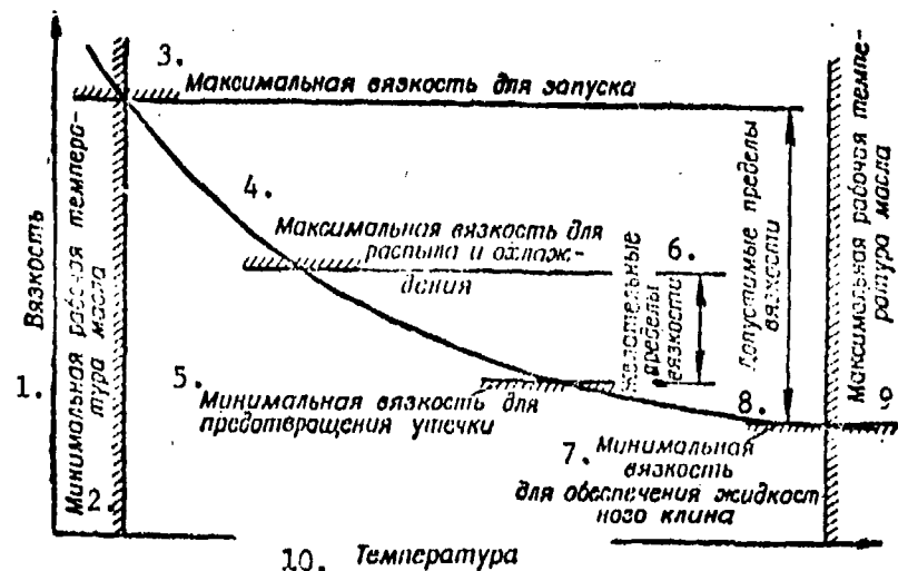
Fig. 41. Requirements placed on the viscosity-temperature properties of oils. Key:
