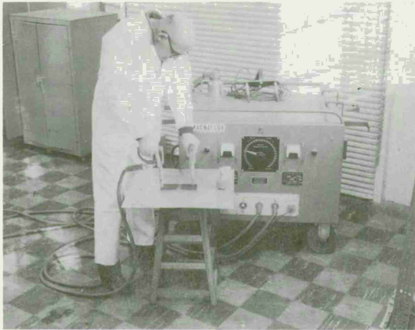
Figure 12. Magnafluxing the vibration plate.
