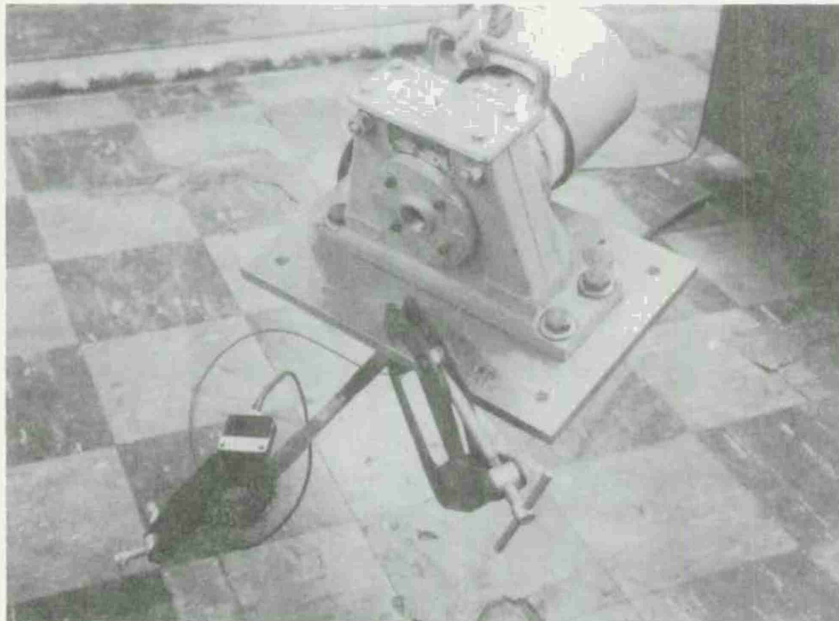
Figure 10. Tensile specimen clamped to the vibrator.
