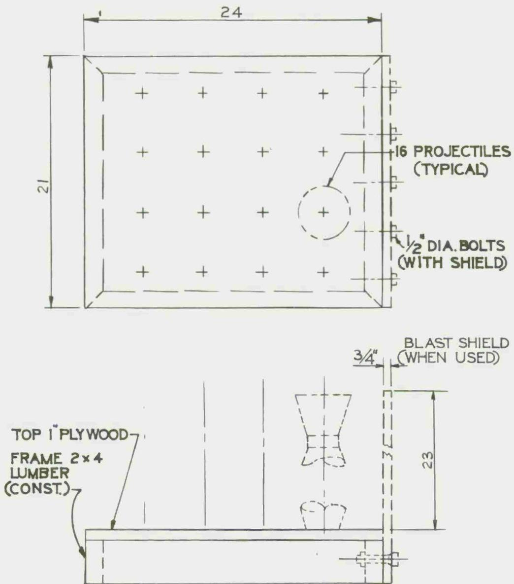
Figure 16 Pallet arrangement.
