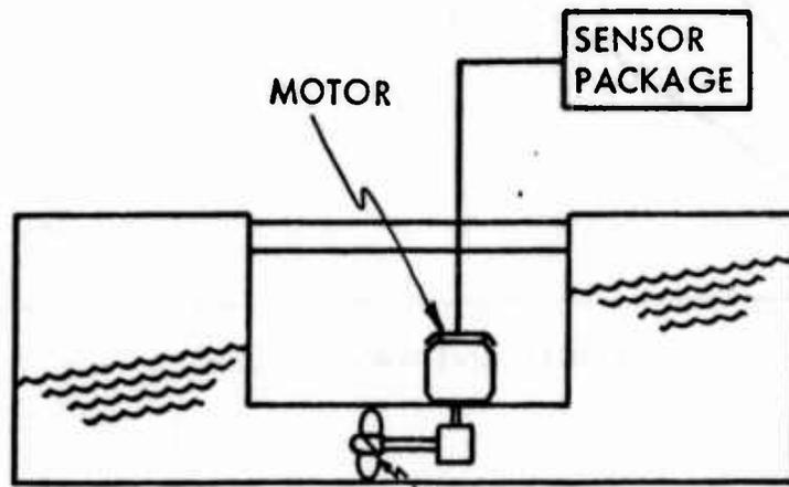
CONTROLLABLE PITCH PROPELLER
