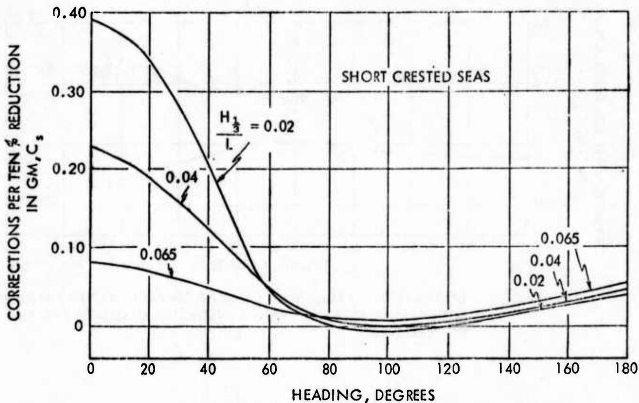
FIGURE 56 - CORRECTION TO ROLL ANGLE VARIATION WITH HEADING ANGLE FOR THREE SIGNIFICANT WAVE HEIGHT TO SHIP LENGTH RATIOS WITH PASSIVE STABILIZER TANKS INSTALLED; AUXILIARY TYPE SHIP AT  $V/\sqrt{L} = 0.8$
