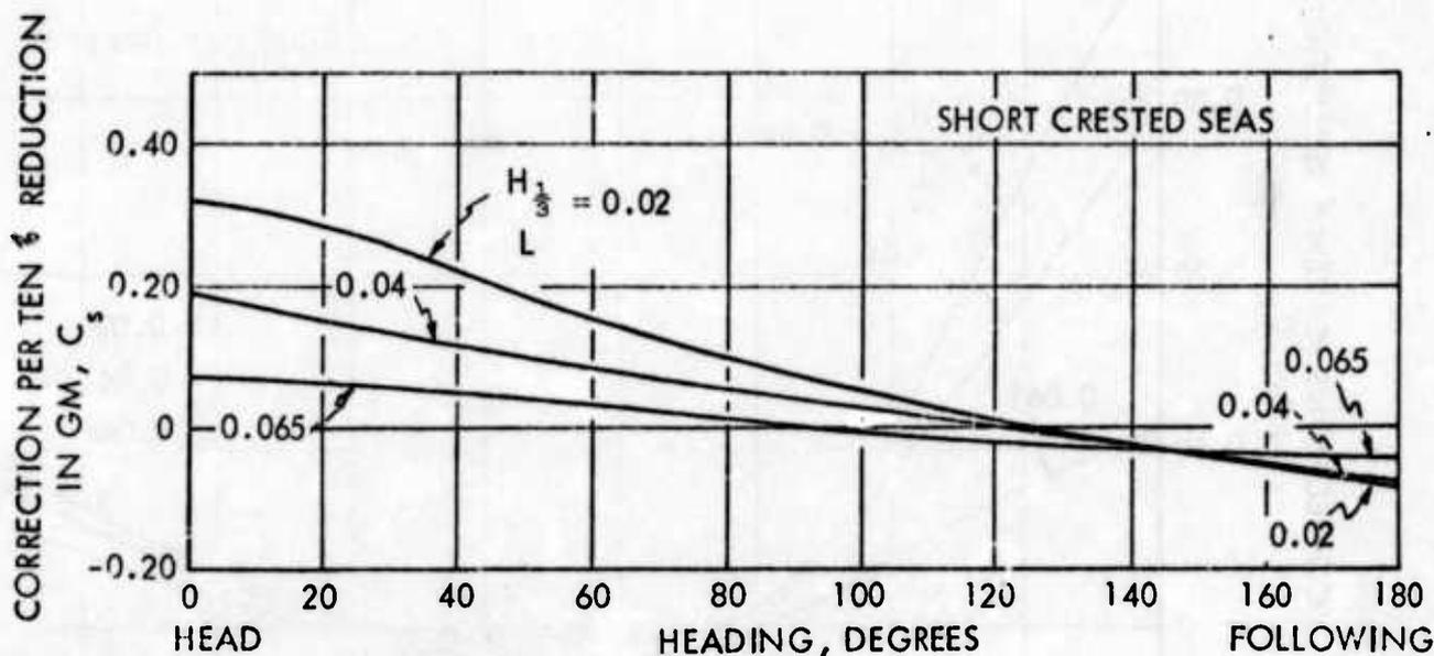
FIGURE 62 - CORRECTION TO ROLL ANGLE VARIATION WITH HEADING ANGLE FOR THREE SIGNIFICANT WAVE HEIGHT TO SHIP LENGTH RATIOS WITH ACTIVE STABILIZER TANKS INSTALLED; AUXILIARY TYPE SHIP AT  $V/\sqrt{L} = 0.04$
