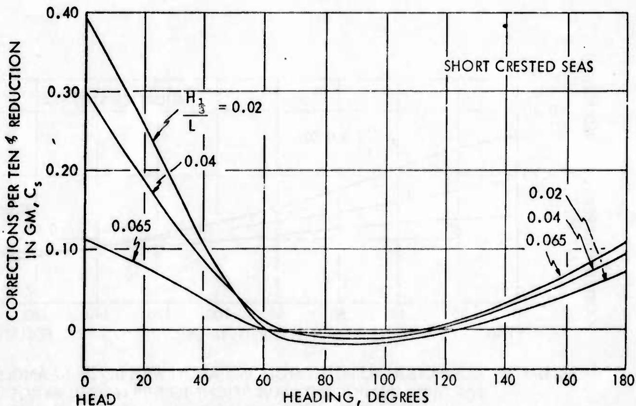
FIGURE 64 - CORRECTION TO ROLL ANGLE VARIATION WITH HEADING ANGLE FOR THREE SIGNIFICANT WAVE HEIGHT TO SHIP LENGTH RATIOS WITH ACTIVE STABILIZER TANKS INSTALLED; AUXILIARY TYPE SHIP AT  $V/\sqrt{L} = 1.2$
