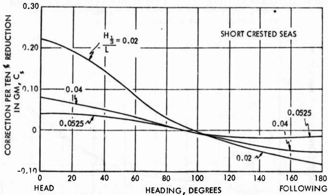
FIGURE 25 - CORRECTION TO ROLL ANGLE VARIATION WITH HEADING ANGLE WITH PASSIVE STABILIZER TANKS INSTALLED; DESTROYER TYPE SHIP AT  $V/\sqrt{L} = 0.4$
