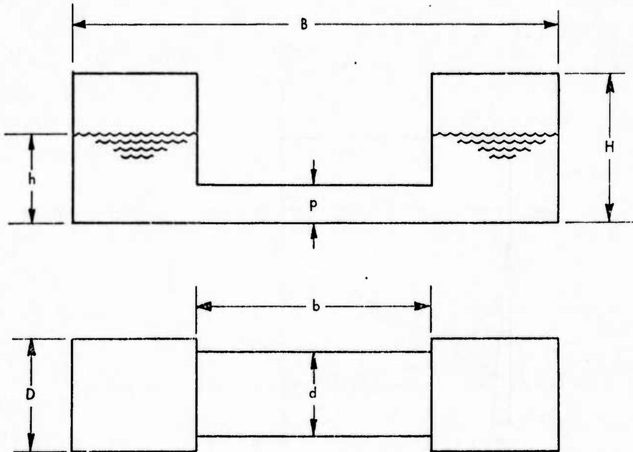
FIGURE 69 - DIMENSIONS OF U-TUBE TANK
