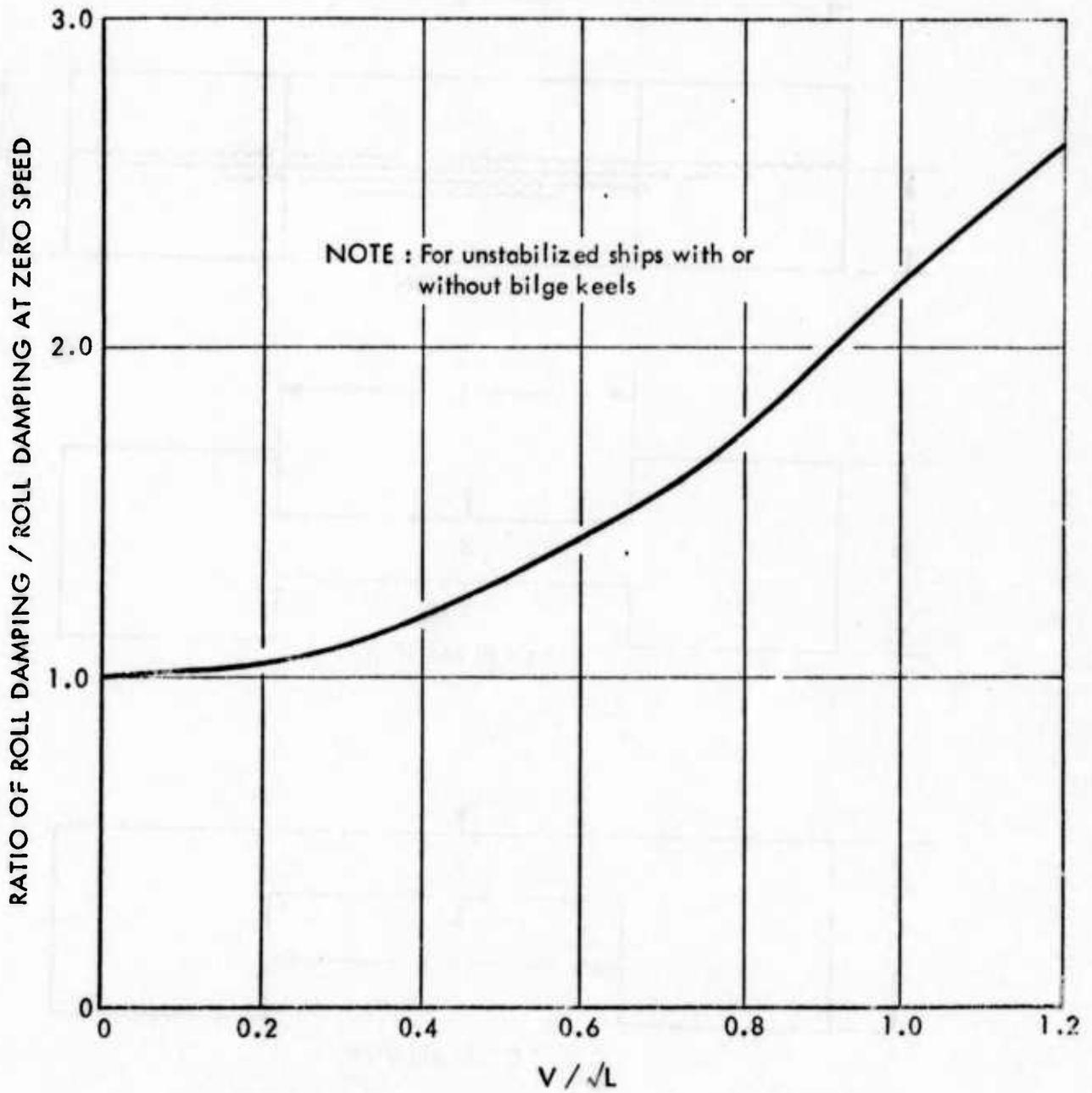
FIGURE 67 - TYPICAL VARIATION OF ROLL DAMPING COEFFICIENT WITH SPEED LENGTH RATIO
