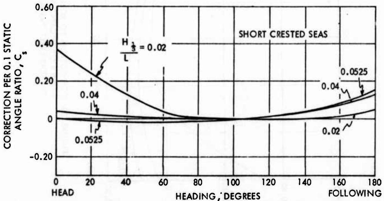
FIGURE 29 - CORRECTION TO ROLL ANGLE VARIATION WITH HEADING ANGLE FOR THREE SIGNIFICANT WAVE HEIGHT TO SHIP LENGTH RATIOS WITH ACTIVE FIN STABILIZER INSTALLED; DESTROYER TYPE SHIP AT  $V/\sqrt{L} = 0.8$
