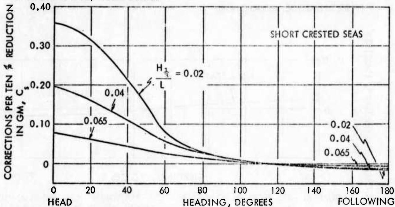
FIGURE 63 - CORRECTION TO ROLL ANGLE VARIATION WITH HEADING ANGLE FOR THREE SIGNIFICANT WAVE HEIGHT TO SHIP LENGTH RATIOS WITH ACTIVE STABILIZER TANKS INSTALLED; AUXILIARY TYPE SHIP AT  $V/\sqrt{L} = 0.8$
