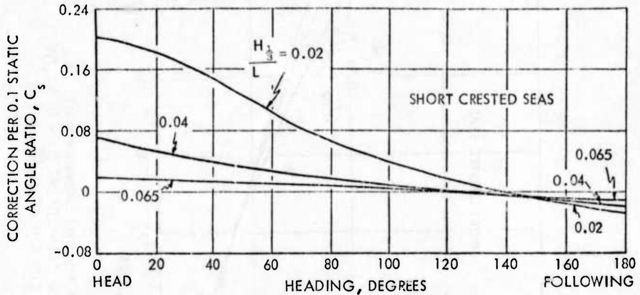
FIGURE 58 - CORRECTION TO ROLL ANGLE VARIATION WITH HEADING ANGLE FOR THREE SIGNIFICANT WAVE HEIGHT TO SHIP LENGTH RATIOS WITH ACTIVE FIN STABILIZER INSTALLED; AUXILIARY TYPE SHIP AT  $V/\sqrt{L} = 0.4$
