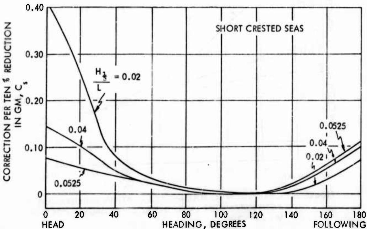
FIGURE 34 - CORRECTION TO ROLL ANGLE VARIATION WITH HEADING ANGLE FOR THREE SIGNIFICANT WAVE HEIGHT TO SHIP LENGTH RATIOS WITH ACTIVE STABILIZER TANK INSTALLED; DESTROYER TYPE SHIP AT  $V/\sqrt{L} = 1.2$
