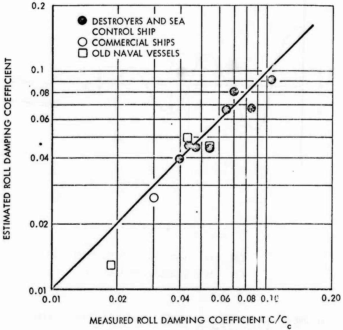
FIGURE 66 - COMPARISON OF ESTIMATED AND MEASURED ROLL DAMPING COEFFICIENTS
