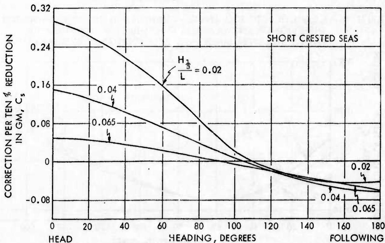
FIGURE 55 - CORRECTION TO ROLL ANGLE VARIATION WITH HEADING ANGLE FOR THREE SIGNIFICANT WAVE HEIGHT TO SHIP LENGTH RATIOS WITH PASSIVE STABILIZER TANKS INSTALLED; AUXILIARY TYPE SHIP AT  $V/\sqrt{L} = 0.04$
