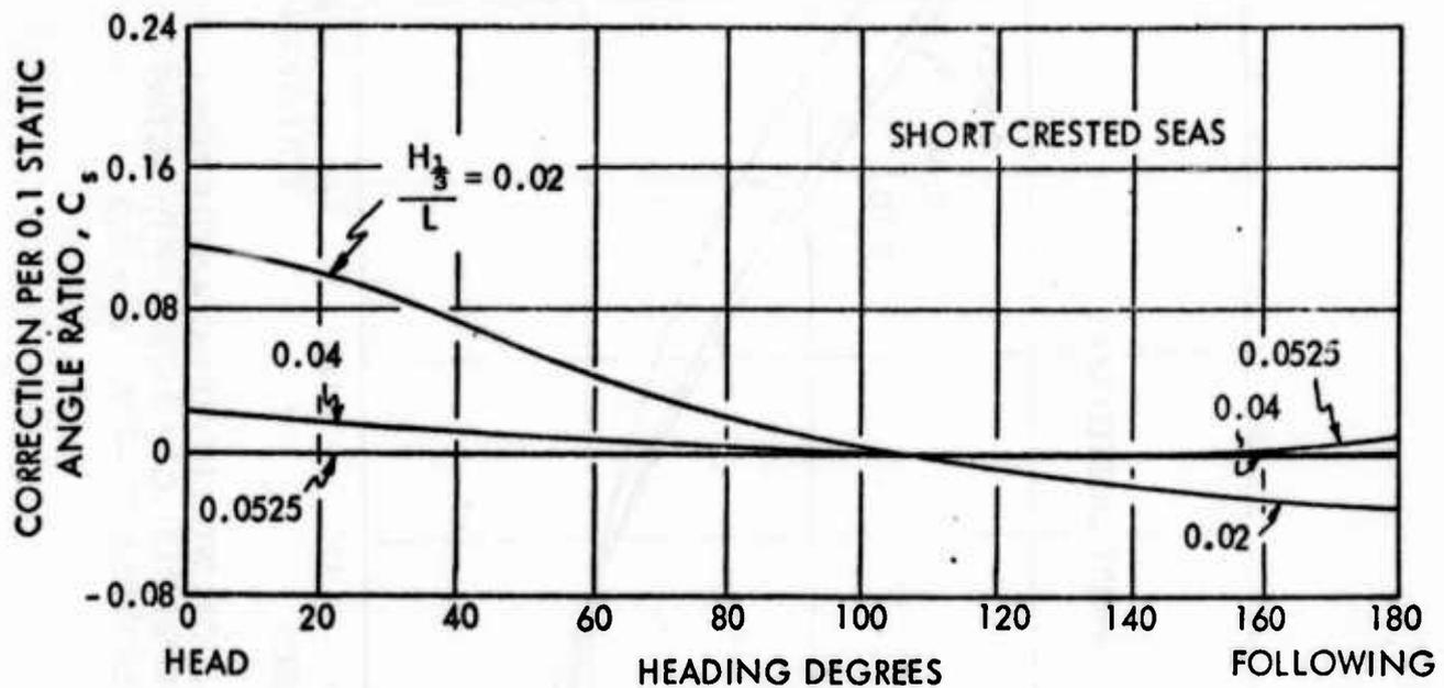
FIGURE 28 - CORRECTION TO ROLL ANGLE VARIATION WITH HEADING ANGLE FOR THREE SIGNIFICANT WAVE HEIGHT TO SHIP LENGTH RATIOS WITH ACTIVE FIN STABILIZER INSTALLED; DESTROYER TYPE SHIP AT  $V/\sqrt{L} = 0.4$
