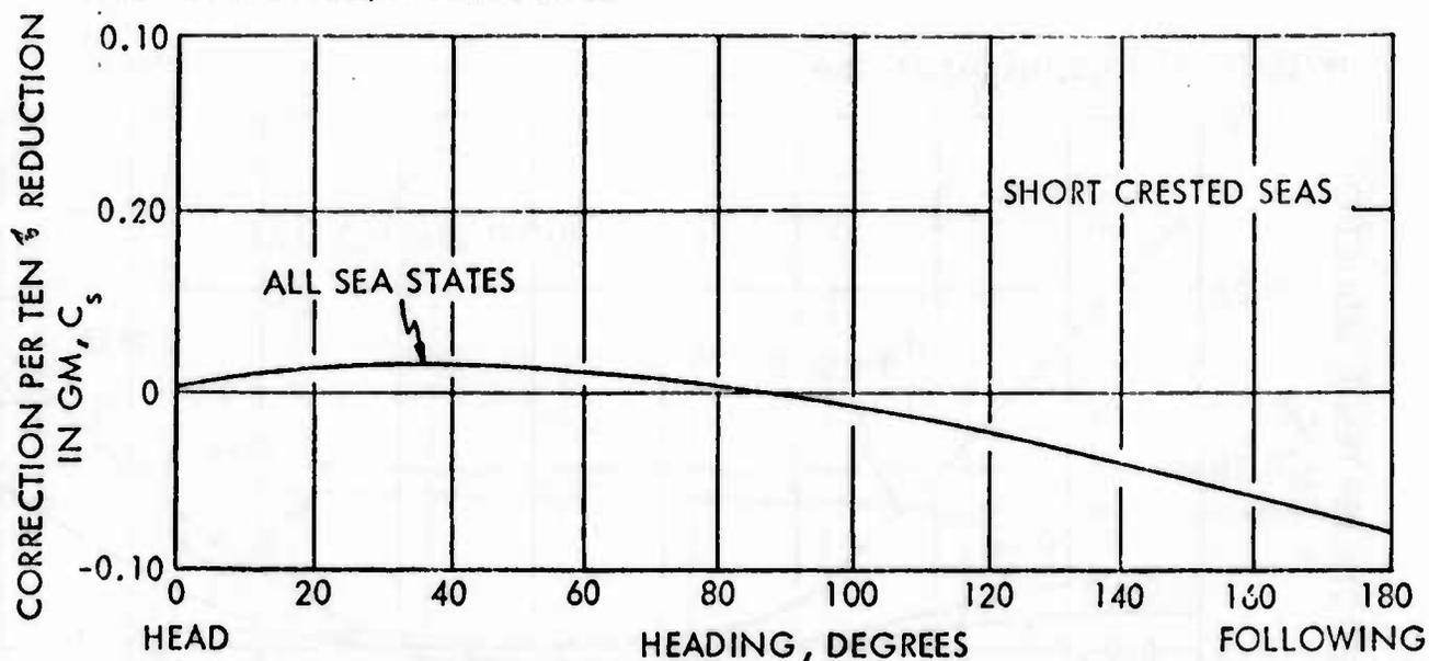
FIGURE 24 - CORRECTION TO ROLL ANGLE VARIATION WITH HEADING ANGLE WITH PASSIVE STABILIZER TANKS INSTALLED; DESTROYER TYPE SHIP AT ZERO SPEED
