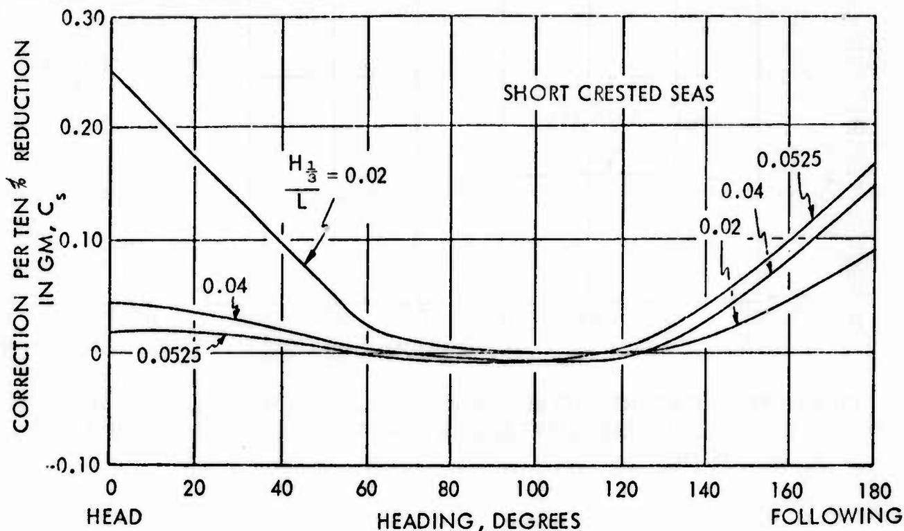
FIGURE 26 - CORRECTION TO ROLL ANGLE VARIATION WITH HEADING ANGLE FOR THREE SIGNIFICANT WAVE HEIGHT TO SHIP LENGTH RATIOS WITH PASSIVE STABILIZER TANKS INSTALLED; DESTROYER TYPE SHIP AT  $V/\sqrt{L} = 0.8$
