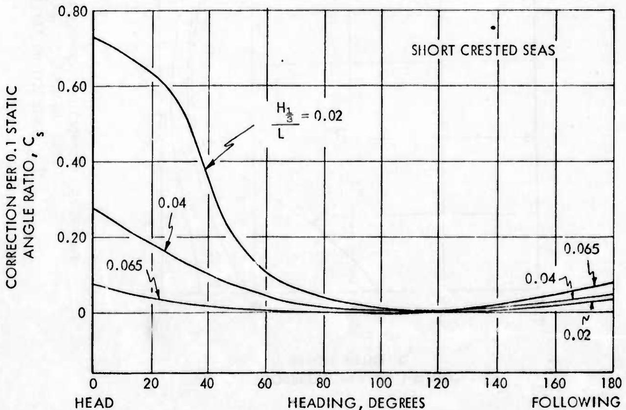
FIGURE 59 - CORRECTION TO ROLL ANGLE VARIATION WITH HEADING ANGLE FOR THREE SIGNIFICANT WAVE HEIGHT TO SHIP LENGTH RATIOS WITH ACTIVE FIN STABILIZER INSTALLED; AUXILIARY TYPE SHIP AT  $V/\sqrt{L} = 0.8$
