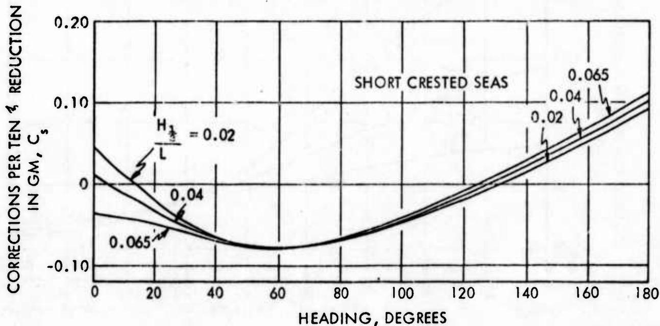
FIGURE 57 - CORRECTION TO ROLL ANGLE VARIATION WITH HEADING ANGLE FOR THREE SIGNIFICANT WAVE HEIGHT TO SHIP LENGTH RATIOS WITH PASSIVE STABILIZER TANKS INSTALLED; AUXILIARY TYPE SHIP AT  $V/\sqrt{L} = 1.2$
