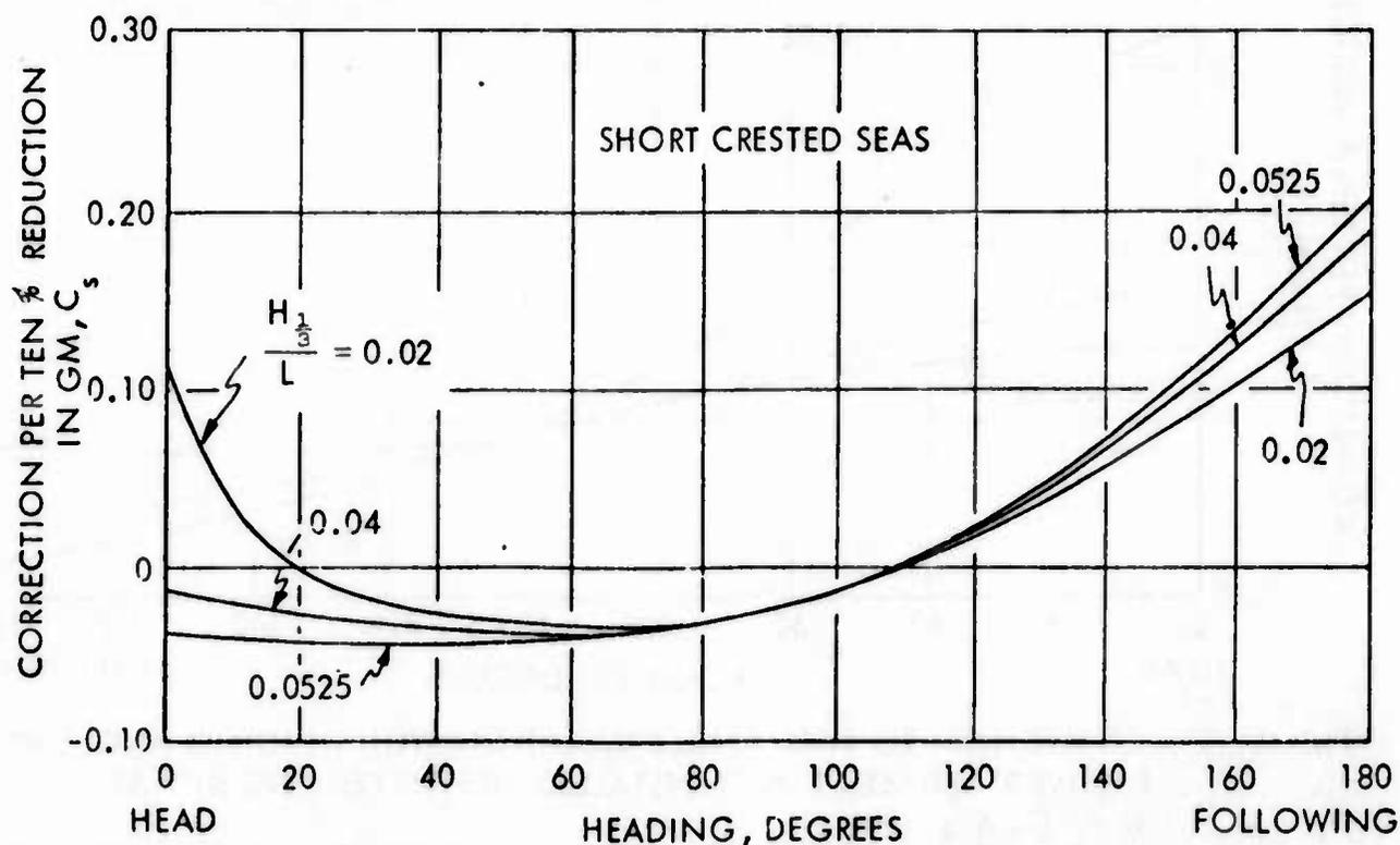
FIGURE 27 - CORRECTION TO ROLL ANGLE VARIATION WITH HEADING ANGLE FOR THREE SIGNIFICANT WAVE HEIGHT TO SHIP LENGTH RATIOS WITH PASSIVE STABILIZER TANKS INSTALLED; DESTROYER TYPE SHIP AT  $V/\sqrt{L} = 1.2$
