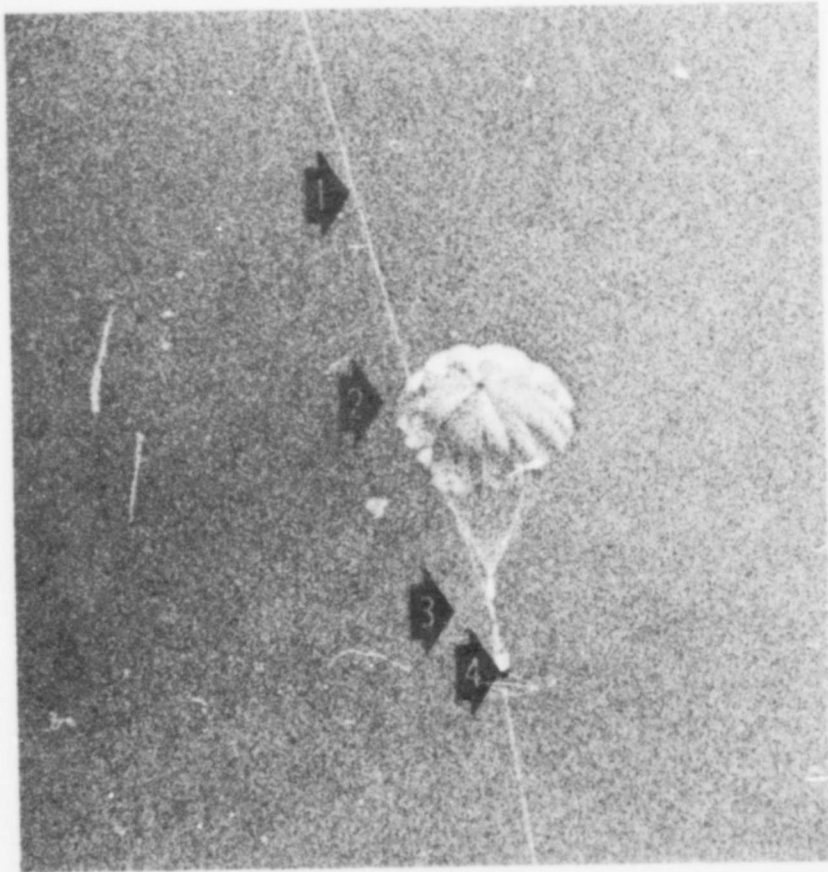
Figure 13. Paraslide 1. Long-Line 2. Parachute 3. Paraslide Ring 4. Dummy Load
