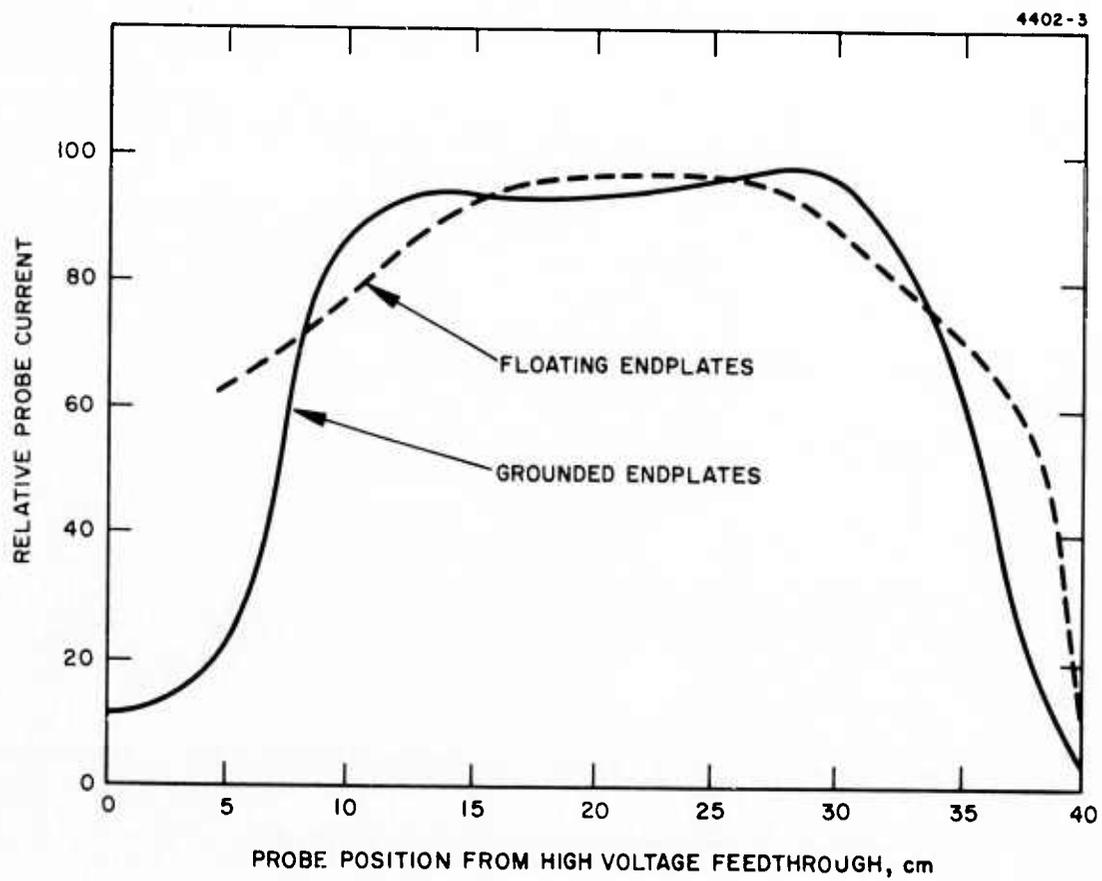
Fig. 8. Comparison of spatial distribution of output current.
