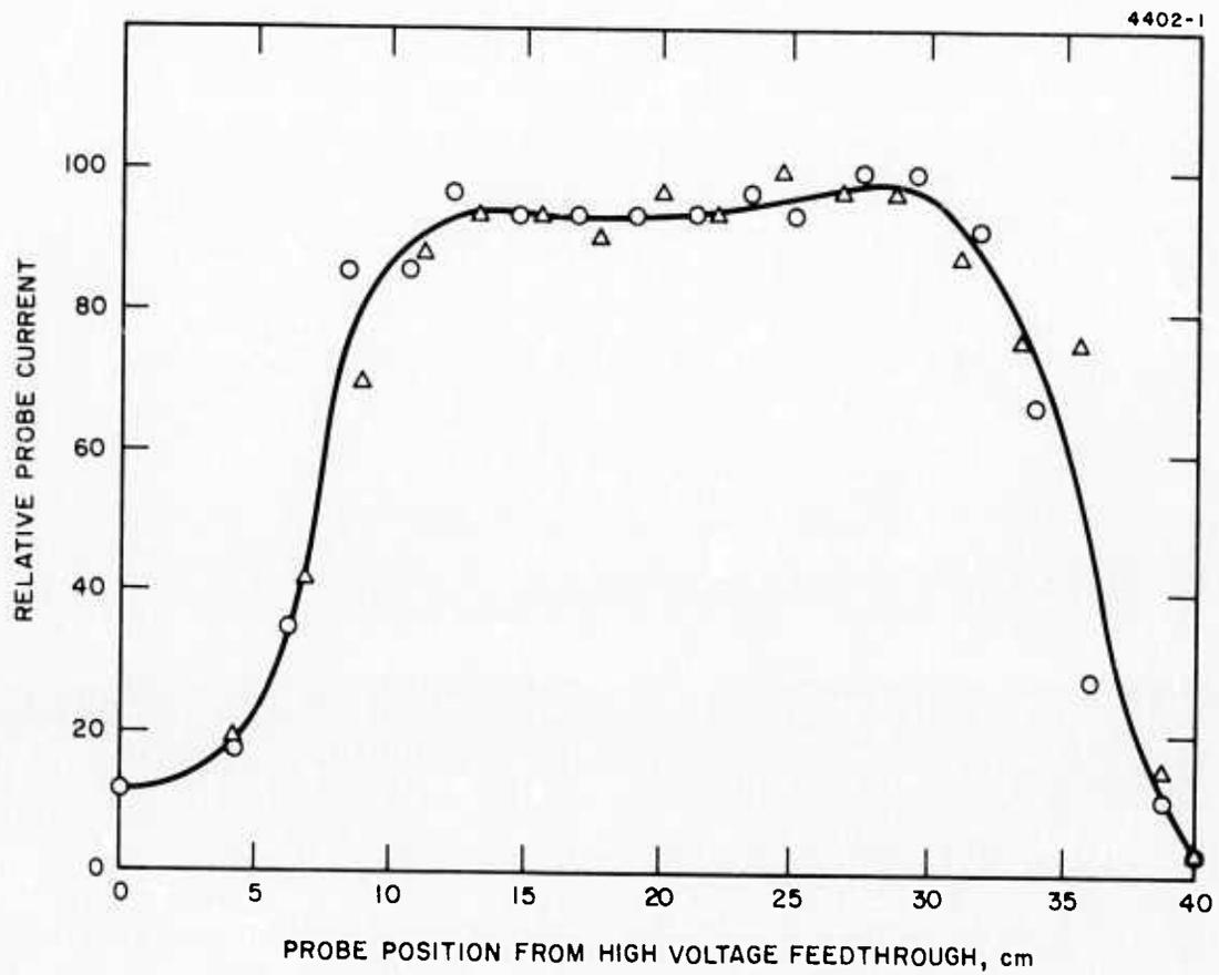
Fig. 6. Relative transmitted beam current versus probe position with endplates tied to the cathode and with a beam voltage of 100 kV and an average current density of  $30 \mu\text{A}/\text{cm}^2$ .
