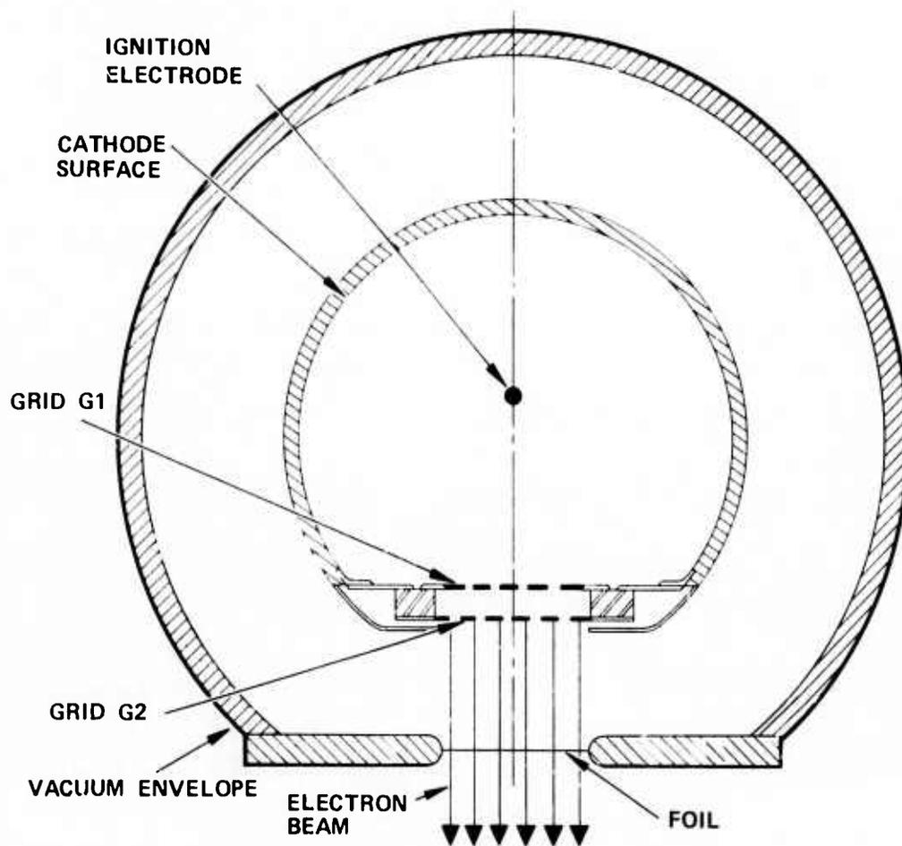
Fig. 4. Cross section of the coaxial e-gun design.
