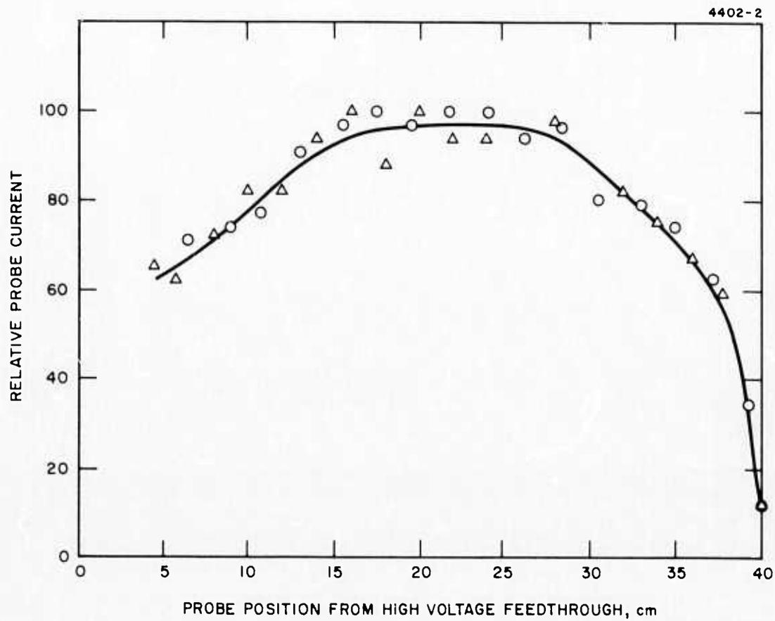
Fig. 7. Relative transmitted beam current versus probe position with endplates floating and with a beam voltage of 100 kV and an average current density of  $30 \mu\text{A}/\text{cm}^2$ .
