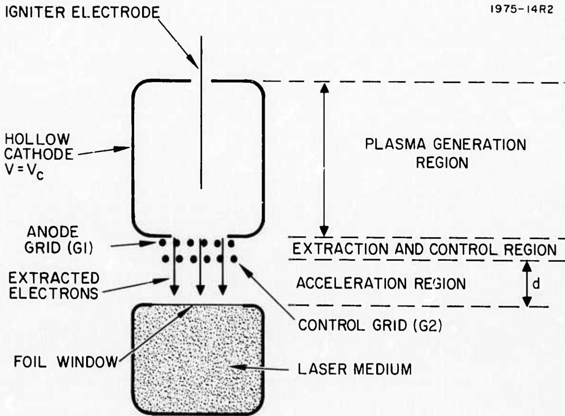
Fig. 1. Schematic of the plasma cathode electron gun.
