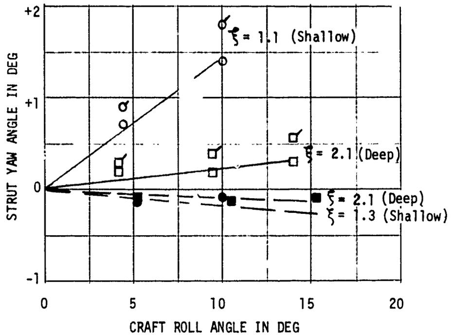
Figure 15 - Average Strut Yaw Angle for the Steady Coordinated Turn in Calm Water as a Function of the Craft Roll Angle
