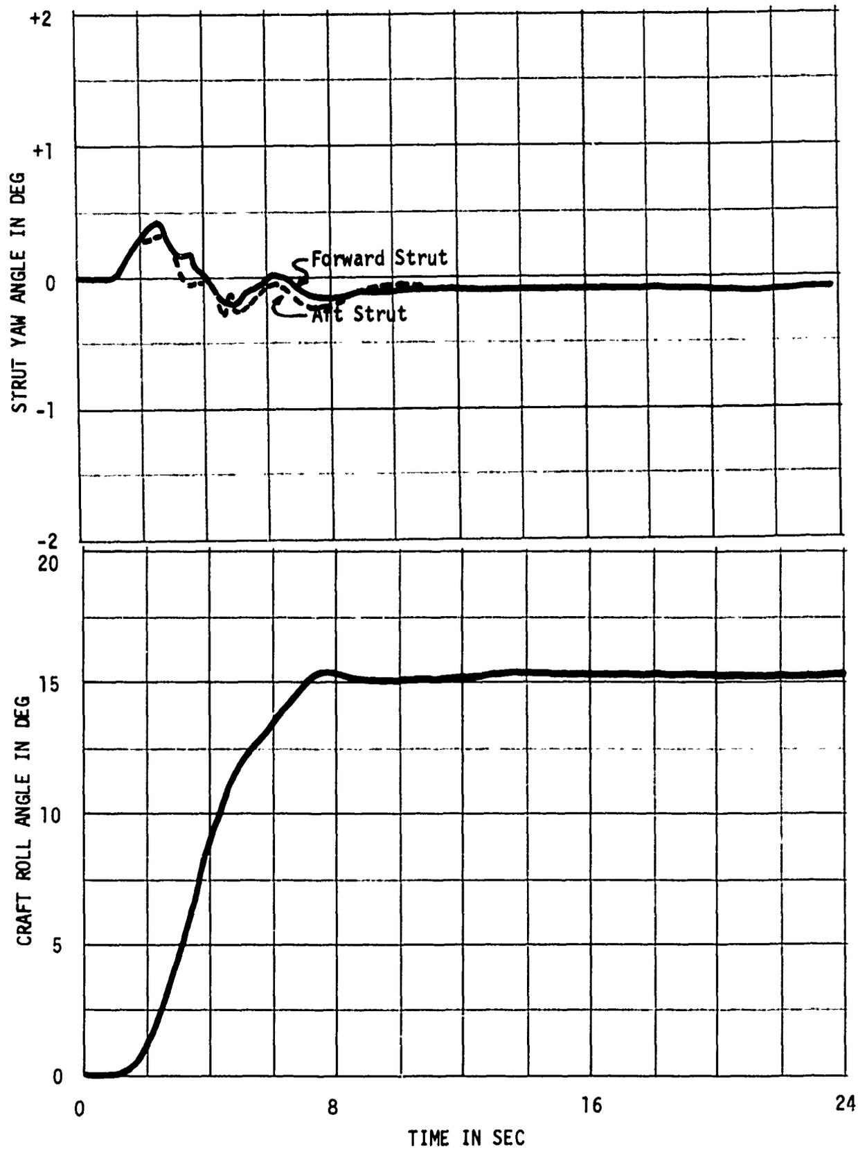
Figure 14(h) - Speed = 60 Knöts; Forward Strut Depth-to-Chord Ratio = 2.1;
