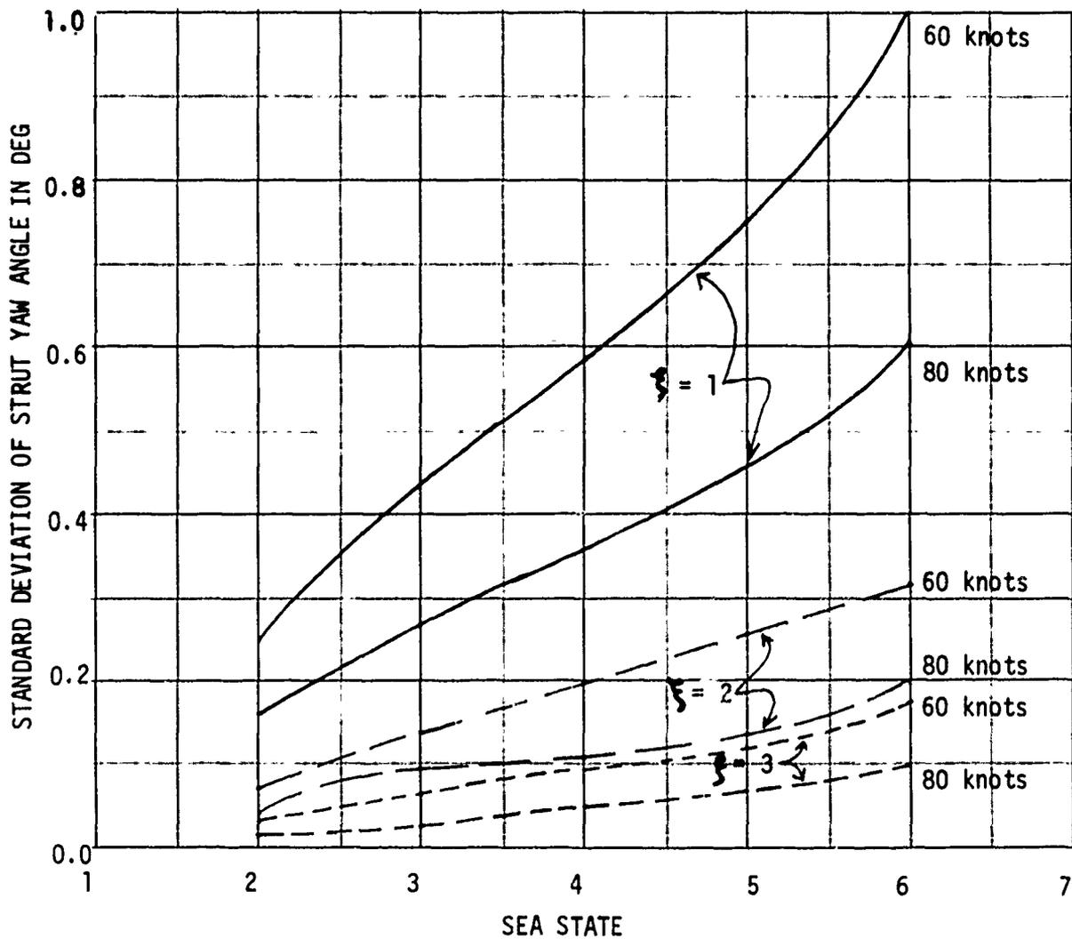
Figure 13 - Standard Deviation of Strut Yaw Angle as a Function of Sea State for Several Values for Strut Depth-to-Chord Ratio  $\xi$
