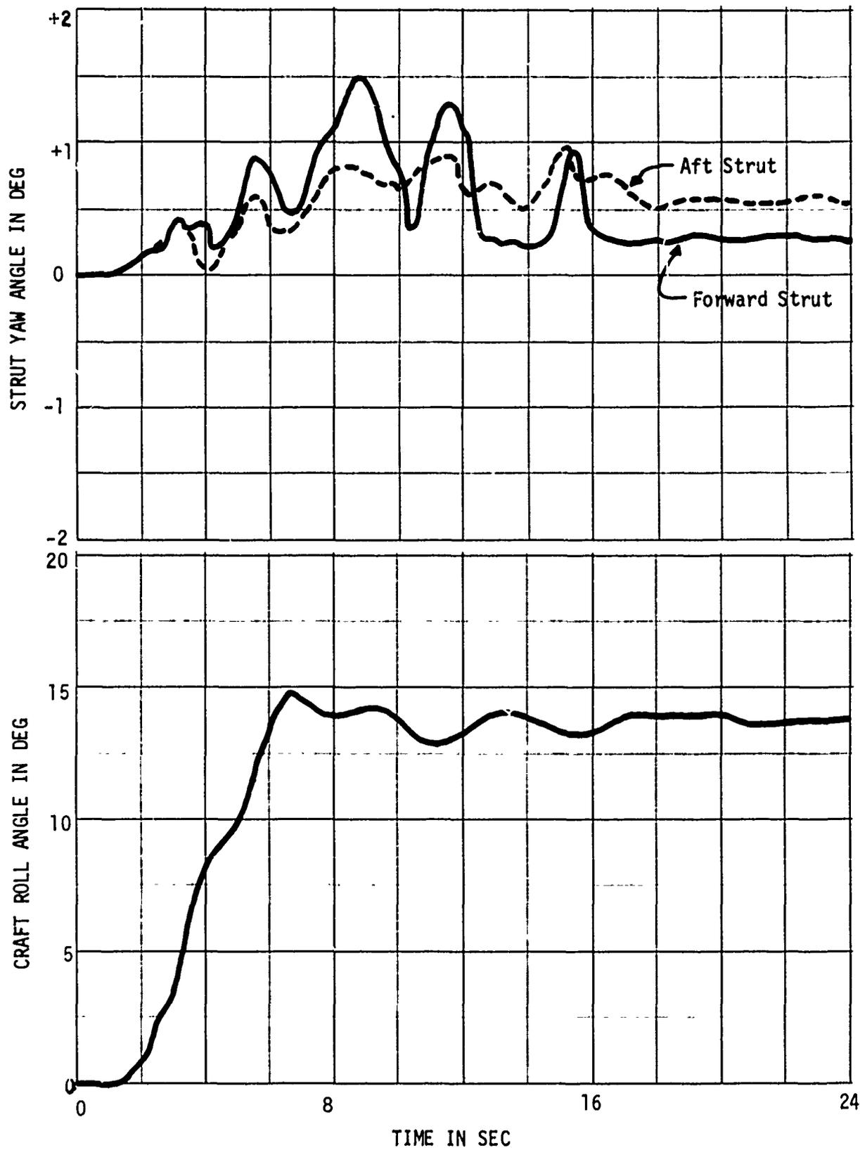
Figure 14(c) - Speed = 80 Knots; Forward Strut Depth-to-Chord Ratio = 2.1;
