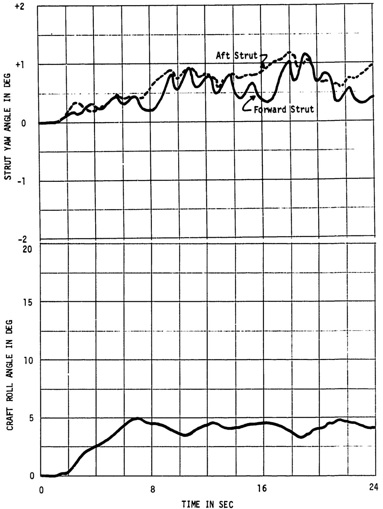
Figure 14(d) - Speed = 80 Knots; Forward Strut Depth-to-Chord Ratio = 1.1;
