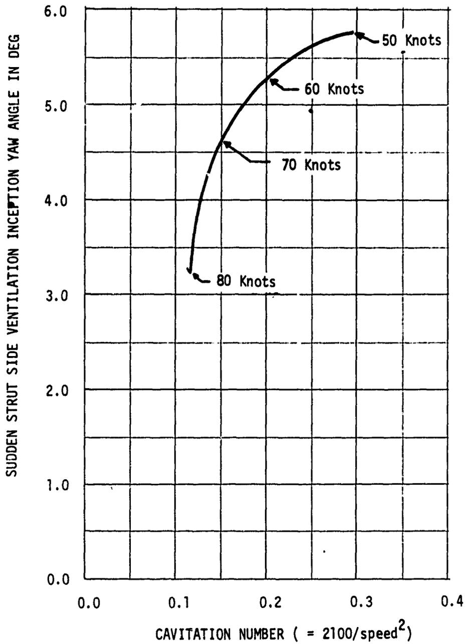
Figure 6 - Sudden Strut Side Ventilation Inception Yaw Angle as a Function of Cavitation Number for a Strut Depth-to-Chord Ratio Equal to One.
