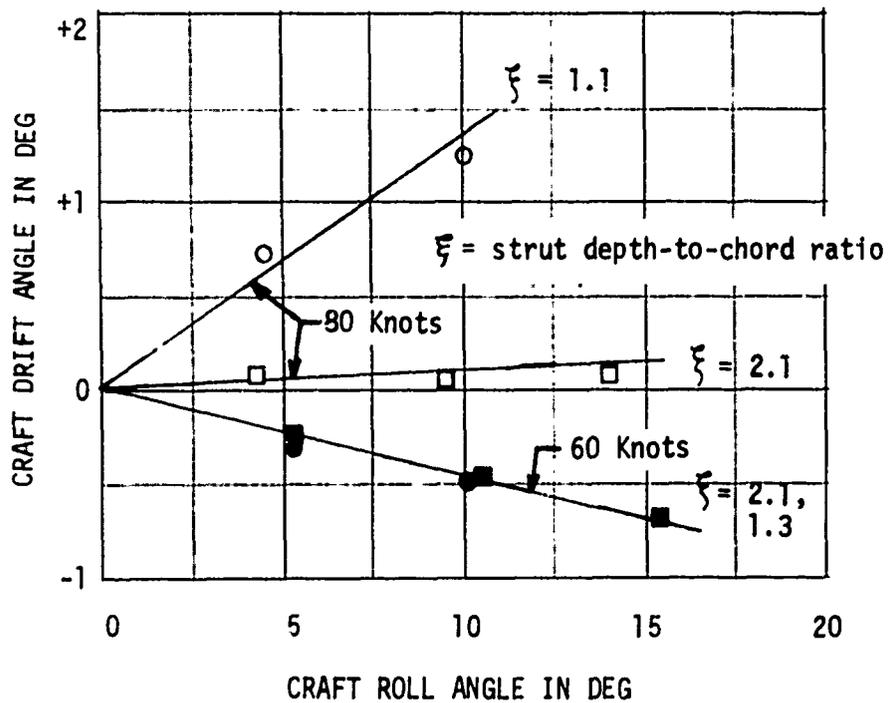
Figure 18 - Craft Drift Angle for the Steady Coordinated Turn in Calm Water as a Function of the Craft Roll Angle
