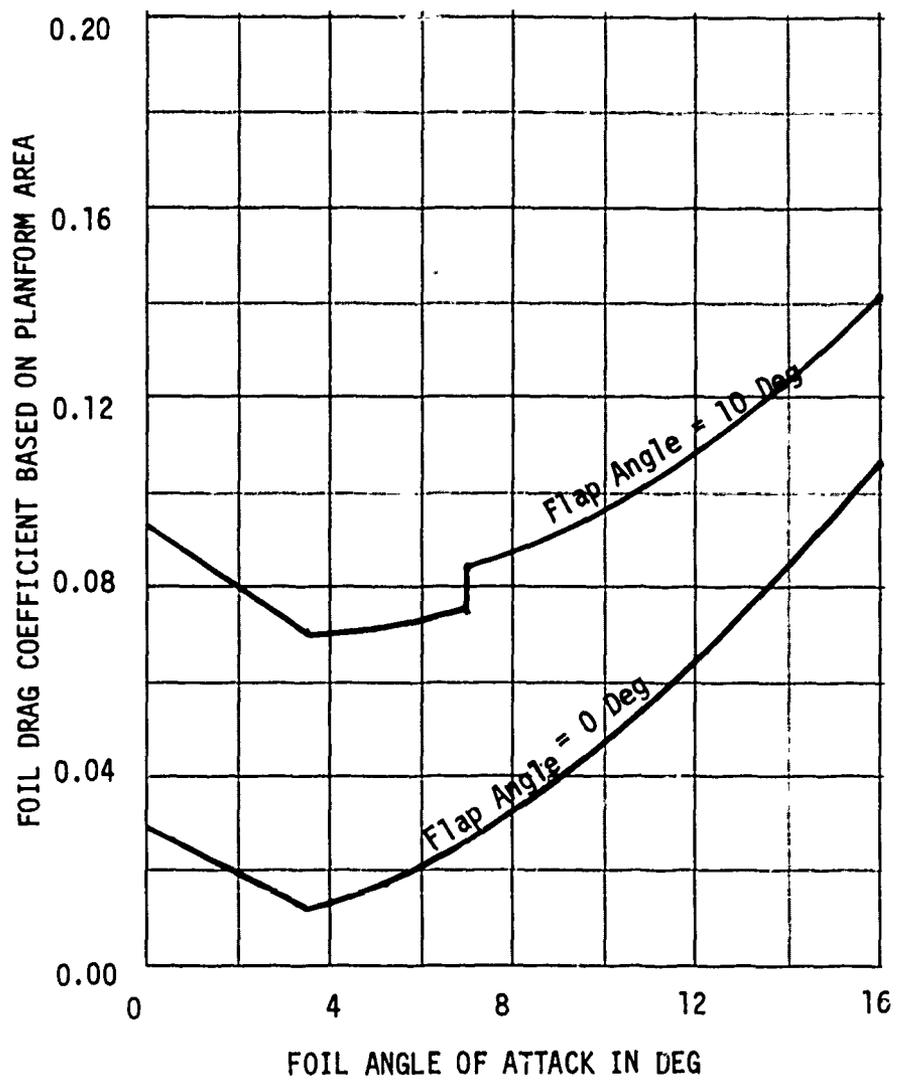
Figure 10 - Foil Drag Coefficient as a Function of Foil Angle of Attack for a Speed of 80 Knots
