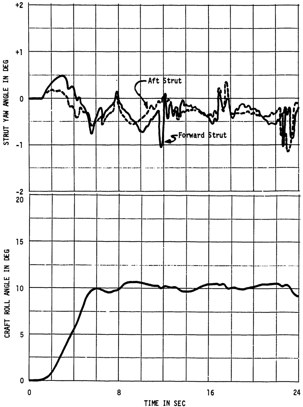
Figure 14(j) - Speed = 60 Knots; Forward Strut Depth-to-Chord Ratio = 1.3;
