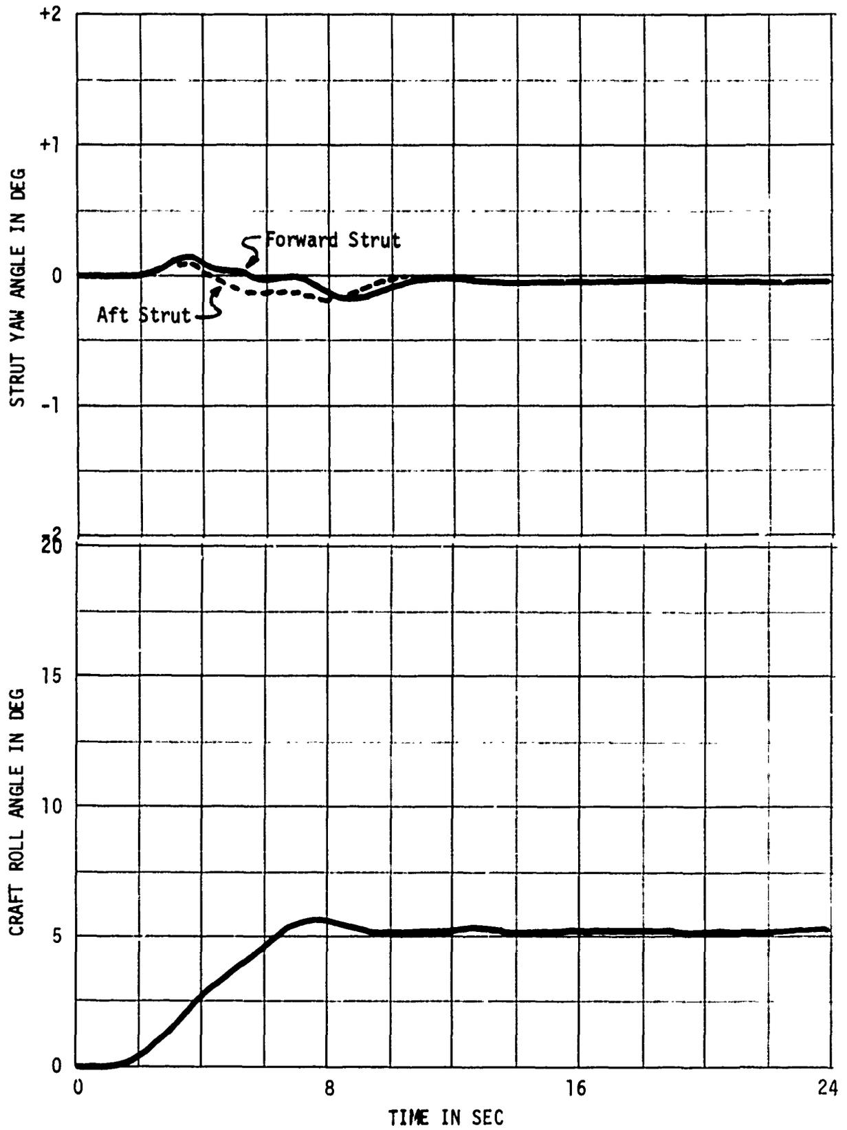
Figure 14(f) - Speed = 60 Knots; Forward Strut Depth-to-Chord Ratio = 2.1;
