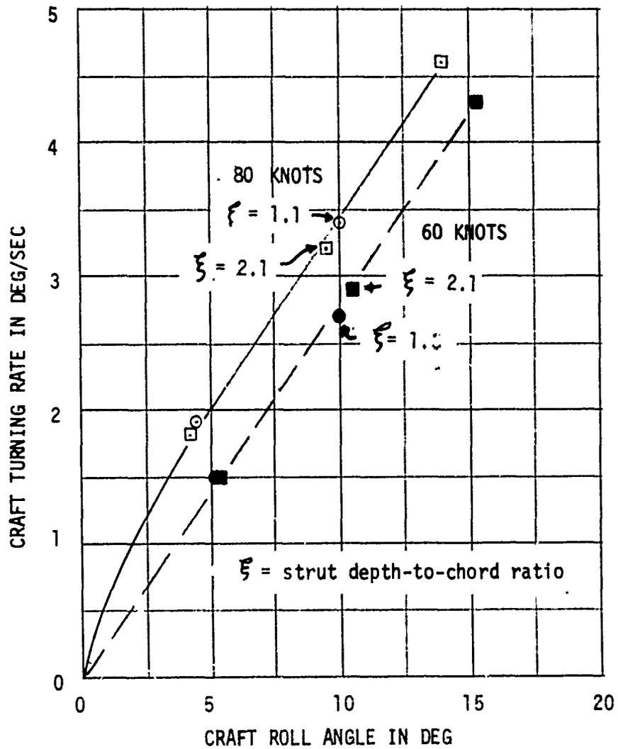
Figure 17 - Craft Turning Rate for the Steady Coordinated Turn in Calm Water as a Function of the Craft Roll Angle
