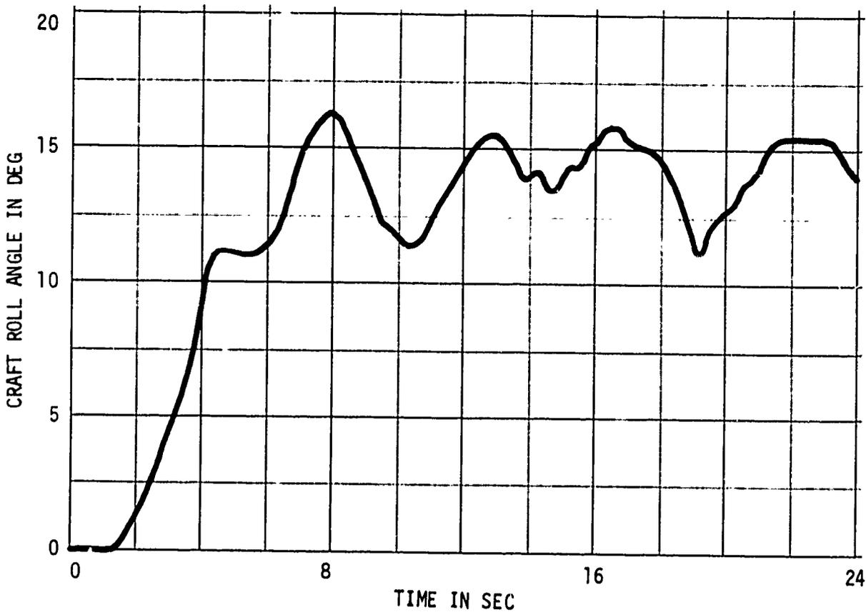
Figure 14(k) - Speed = 60 Knots; Forward Strut Depth-to-Chord Ratio = 1.3;
