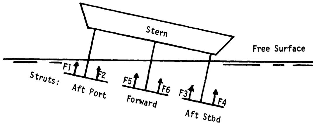
The horizontal components of the forces F1 through F6 provide the lateral acceleration, while the vertical components balance the craft weight.
