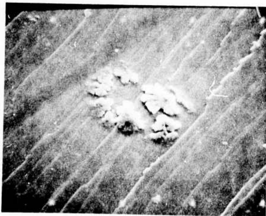
Fig 5b Fracture Surface of Cast \text{SrF}_2 Sample. SEM 2000 \times
