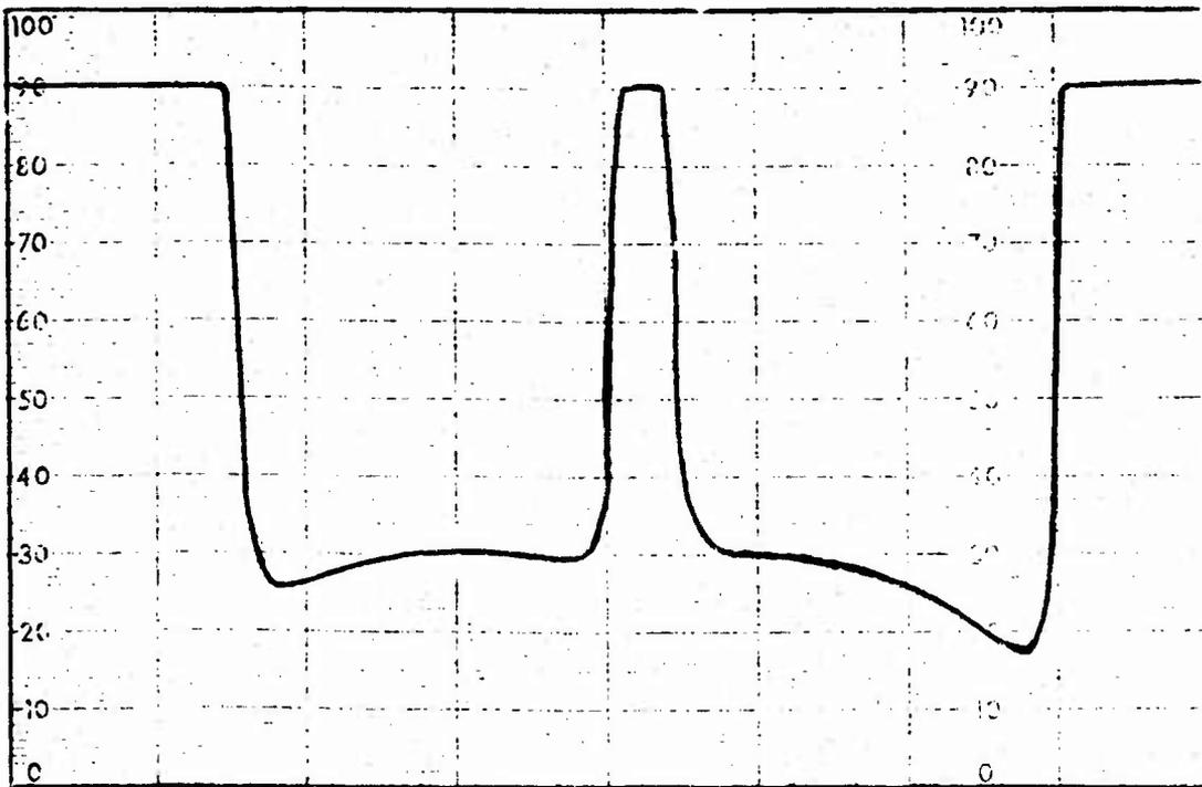
Figure 29. Dektak Trace Showing Profile of the  $50\mu$  Wide Two Dimensional Waveguide. Horizontal Magnification 100, Vertical Full Scale  $50\mu$ .
