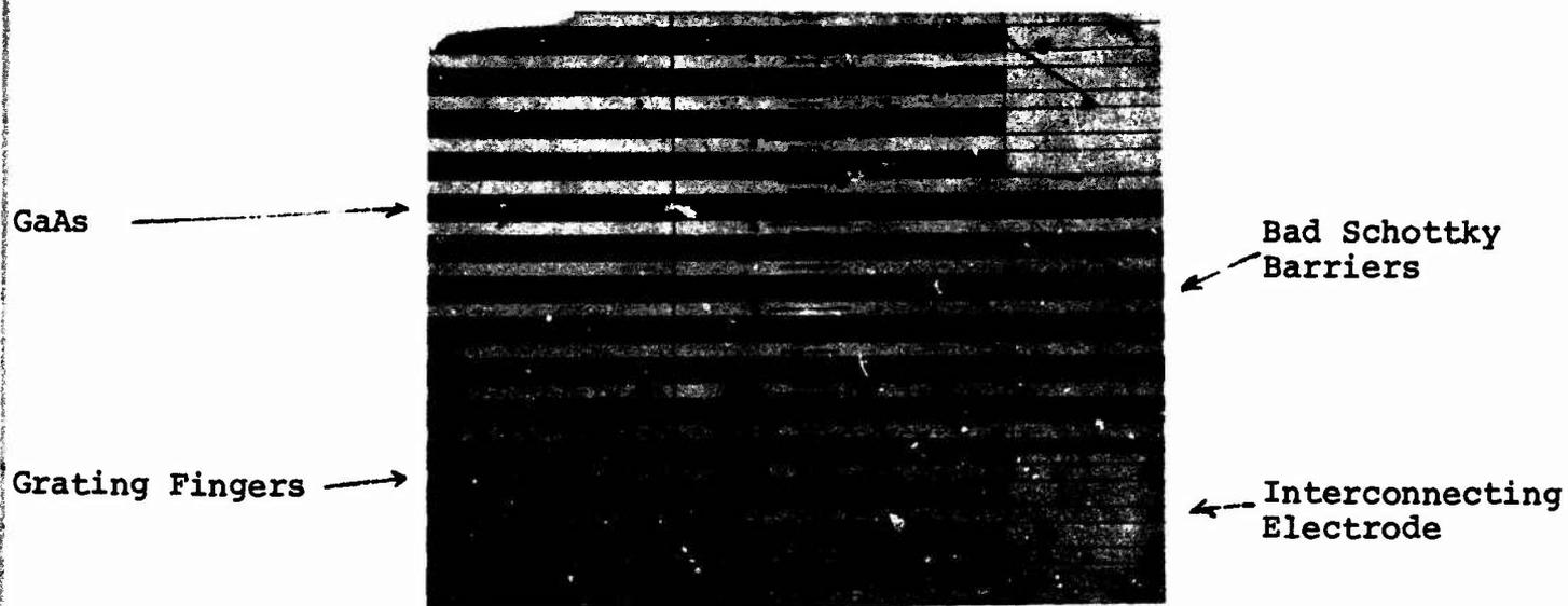
Figure 41: Microscope Picture of the Grating Electrodes
