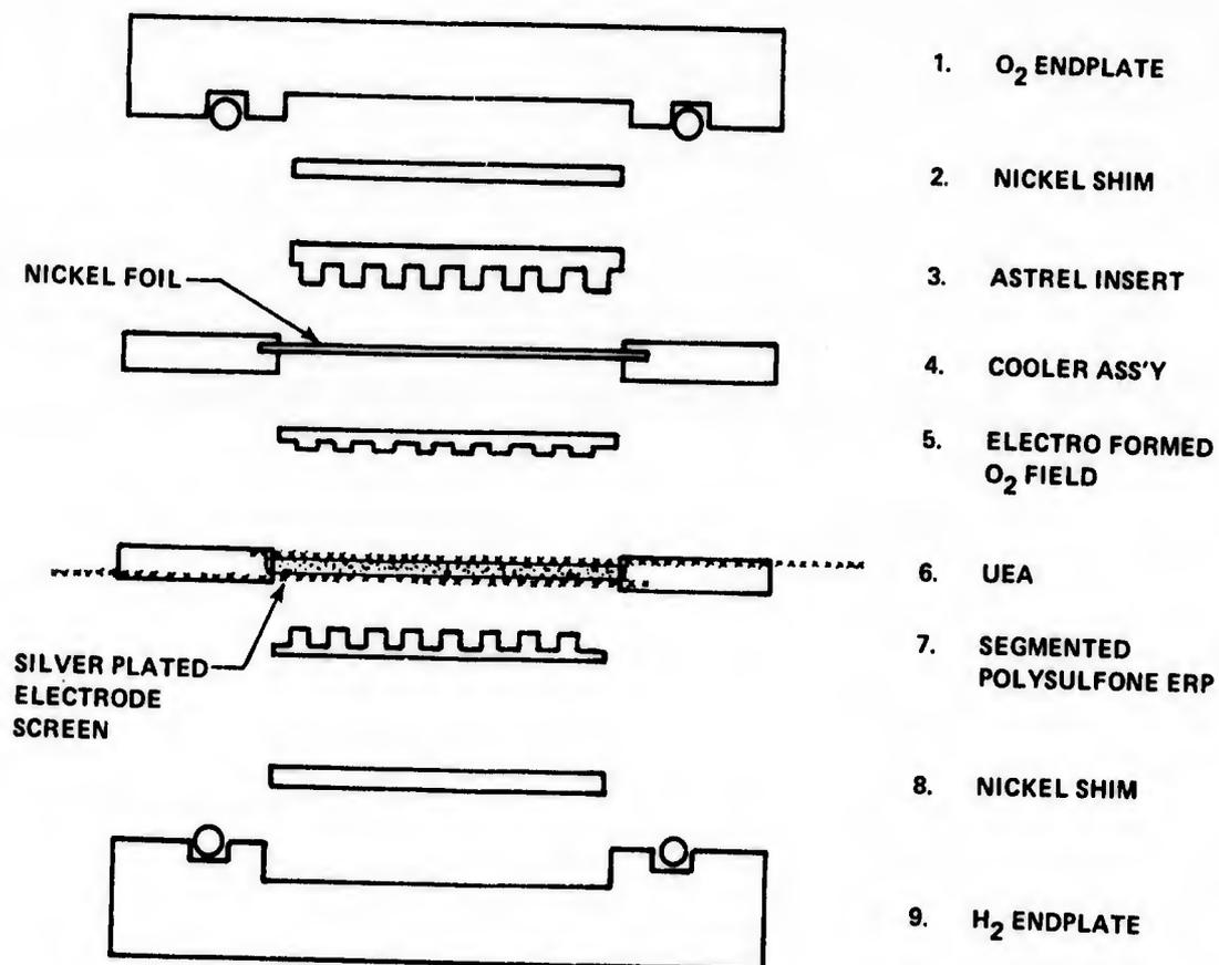
Figure 2 – Configuration 4 Cell Cross Section
