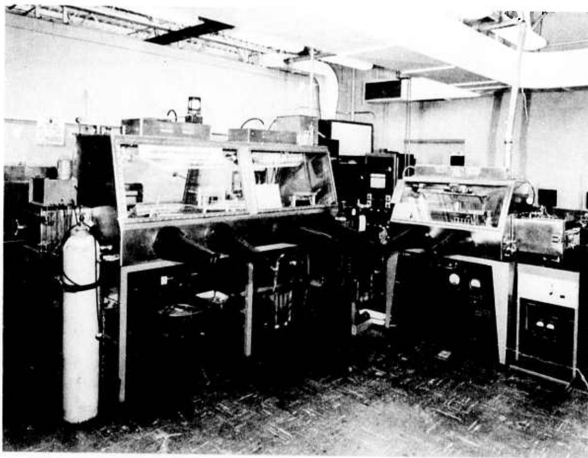
Fig. 5.2: Glove box facilities utilized for the preparation and handling of materials being evaluated for NaK compatibility
