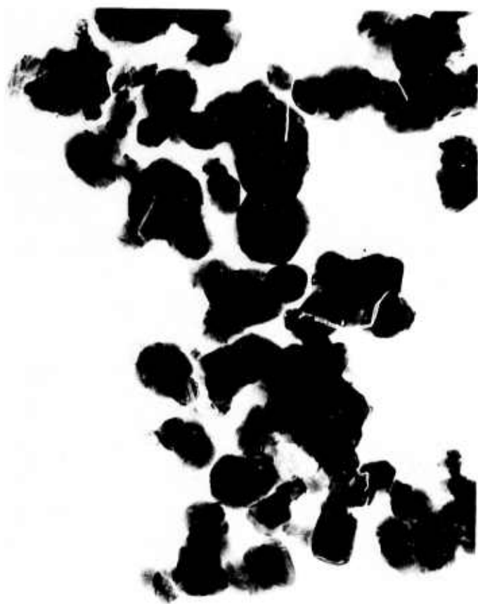
Fig. 25 TEM photomicrograph of sintered particles of loose powder of \beta -SiC containing 0.8% C fired at 1900°C for 1 hr in argon. 24,400X
