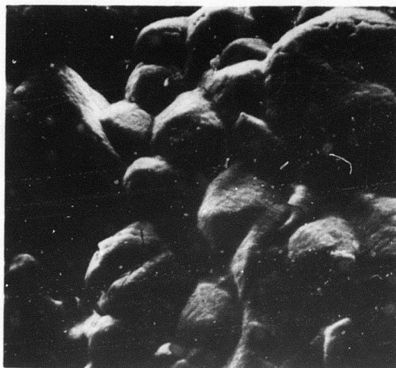
Fig. 3 Scanning electron micrograph of the surface of the CVD \text{Si}_3\text{N}_4 after oxidation for 259 hours in air at 1410^\circ\text{C} . 500X
