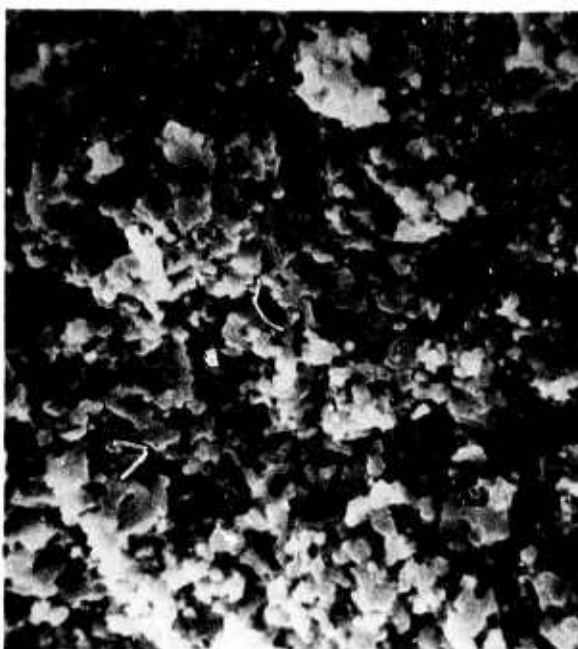
Fig. 32 Microstructure of a sintered specimen of \beta -SiC containing 0.8% C fired at 1900°C for 1 hr in argon. SEM of fractured surface. 2000X
