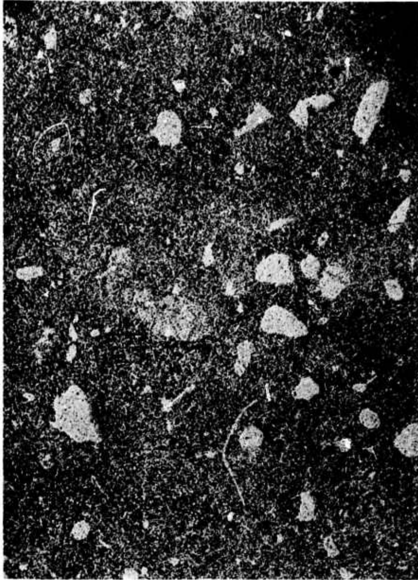
Fig. 22 Polished section of a specimen of Powder I ( \beta -SiC + 0.8% C + 0.6% B) sintered for 300 min at 2000°C. Note large dense regions in the micro-structure. 150X
