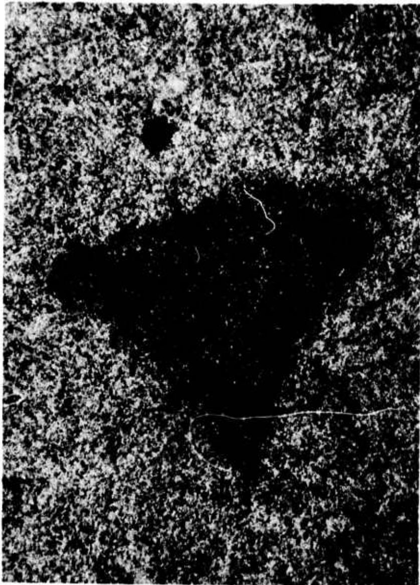
Fig. 23 Microstructure of a dense, solid region in sintered \beta -SiC containing 0.8% C and 0.6% B chemically etched in 10 parts KOH + 1 part \text{KNO}_3 at 650^\circ\text{C} for 30 seconds.
