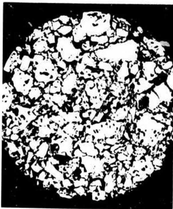
Fig. 6 Cross section of a commercial SiC heater rod before use. 14X
