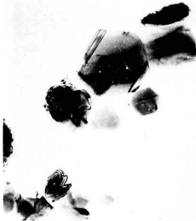
Fig. 29 Sintered particles of loose powder of \beta -SiC containing 0.6% B fired at 1900°C for 2 hrs in argon. 64,000X
