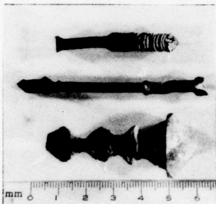
Figure 4. ECT grown crystals ( [111] ) with various current-pull rate combinations. Top: Constant pull rate with current doubled after initial growth period. Middle: Current and pull rate varied to maintain constant cross section. Branching due to exceeding maximum stable pull rate. Bottom: Constant pull rate with constantly varying current.
