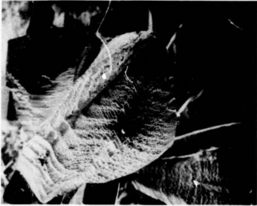
Figure 9. Dendrites along [111] direction, 500X.
