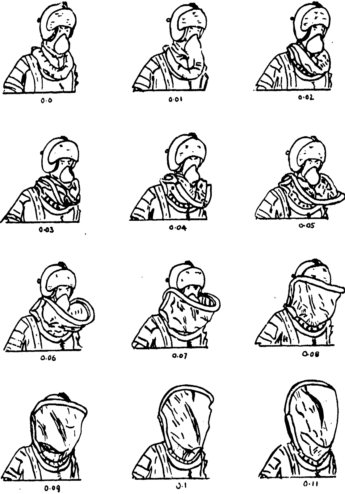
Fig.6 Erection of anti-blast hood V_s time (sec)
