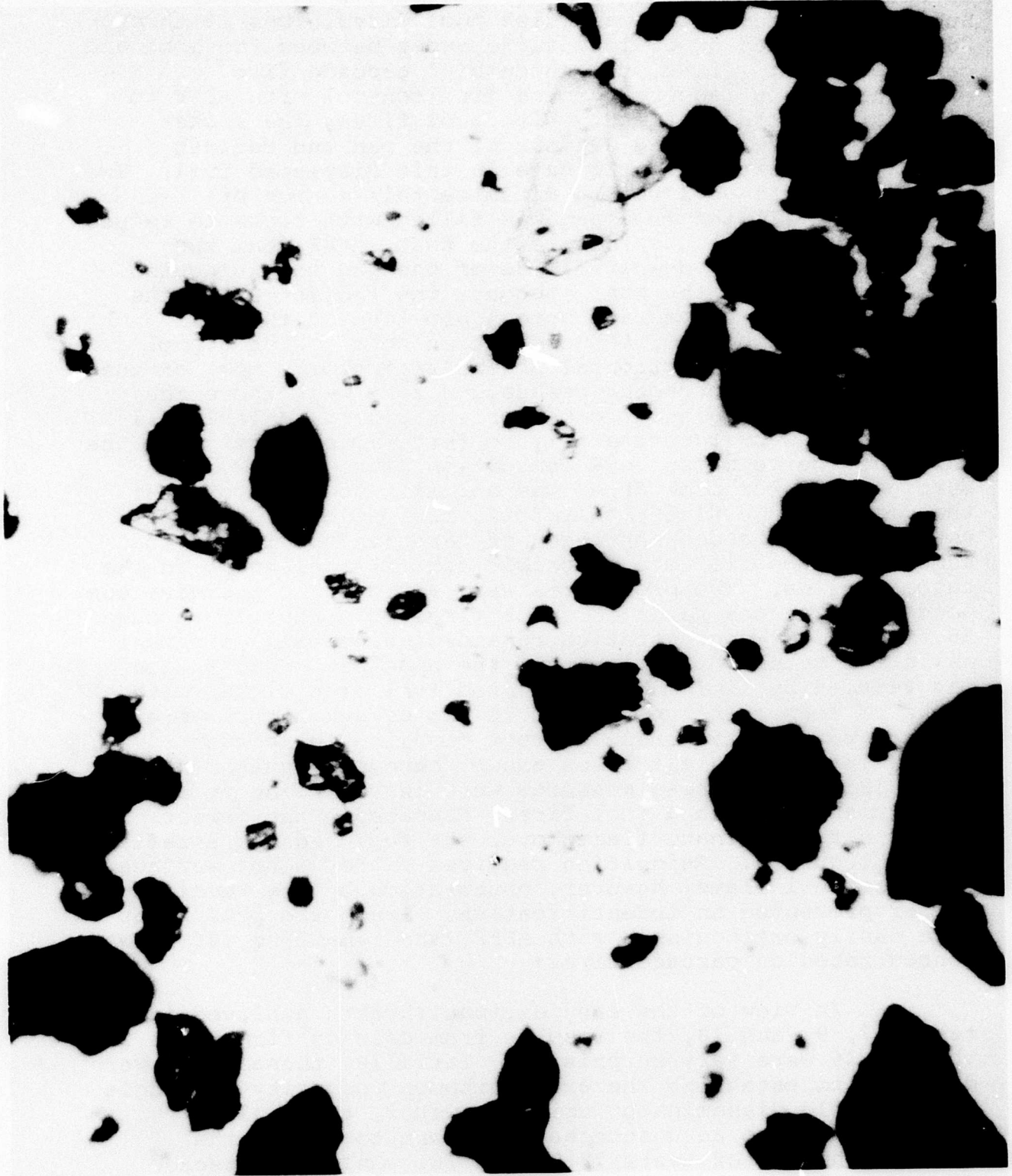
FIG. 3.5.2 PHOTOMICROGRAPH OF MONNEX DISCHARGED THROUGH THE POWDER DISSEMINATOR, MAGNIFICATION = 360X
