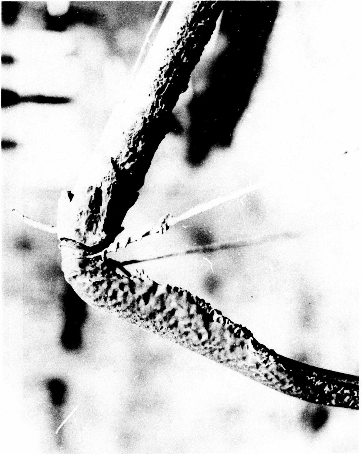
FIG. 3.4 SLURRY DEPOSIT ON PIPE AND WIRES AFTER A SINGLE DISCHARGE
