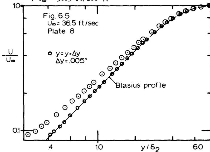
Fig. 6.5 Laminar mean velocity profile on a rough plate.
