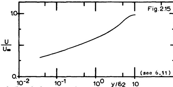
Fig. 2.15 Typical rough surface mean velocity profile.
