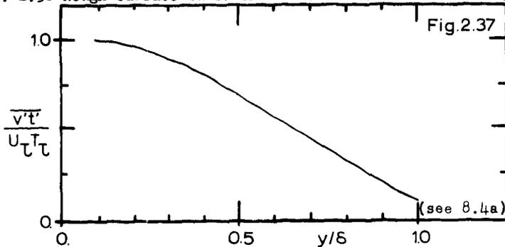
Fig. 2.37 Rough surface turbulent heat flux distribution.
