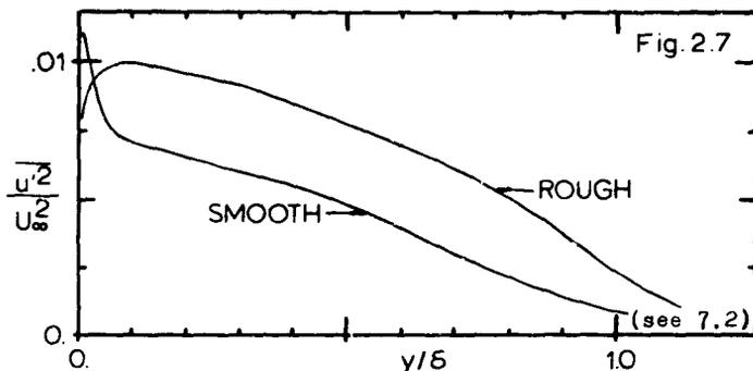
Fig. 2.7 Rough vs. smooth axial velocity fluctuations.
