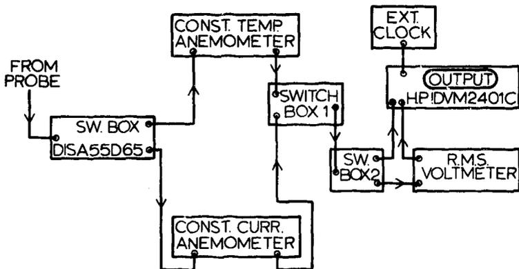
Fig. 4.5 Schematic of the hot-wire instrumentation and circuitry.
