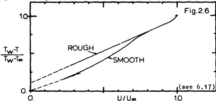
Fig. 2.6 Rough vs. smooth mean temperature-mean velocity profiles.
