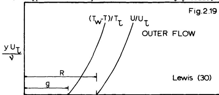
Fig. 2.19 Outer flow of a rough wall layer and wall functions  $R$  and  $g$  according to Lewis.
