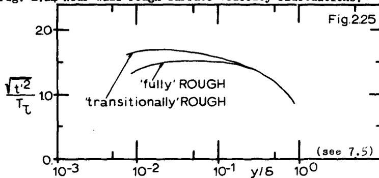
Fig. 2.25 Near wall rough surface temperature fluctuations.
