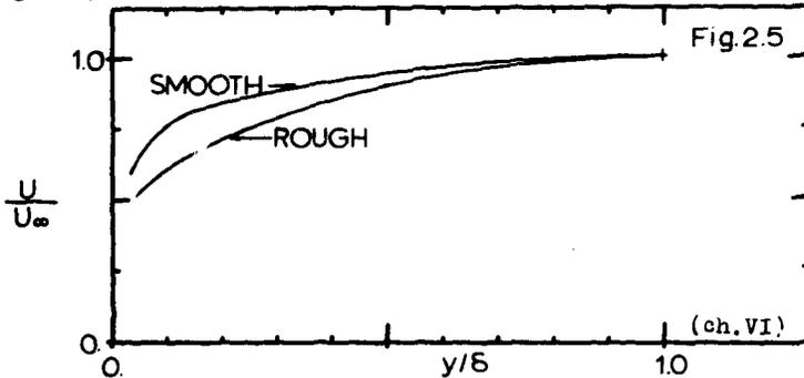
Fig. 2.5 Rough vs. smooth mean velocity profiles.
