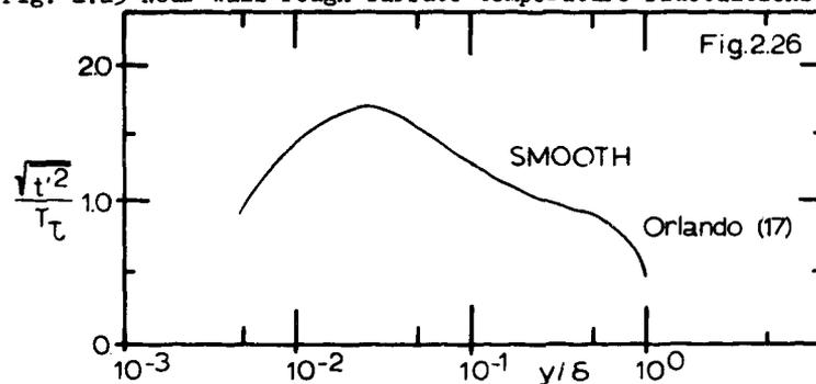
Fig. 2.26 Near wall smooth surface temperature fluctuations.
