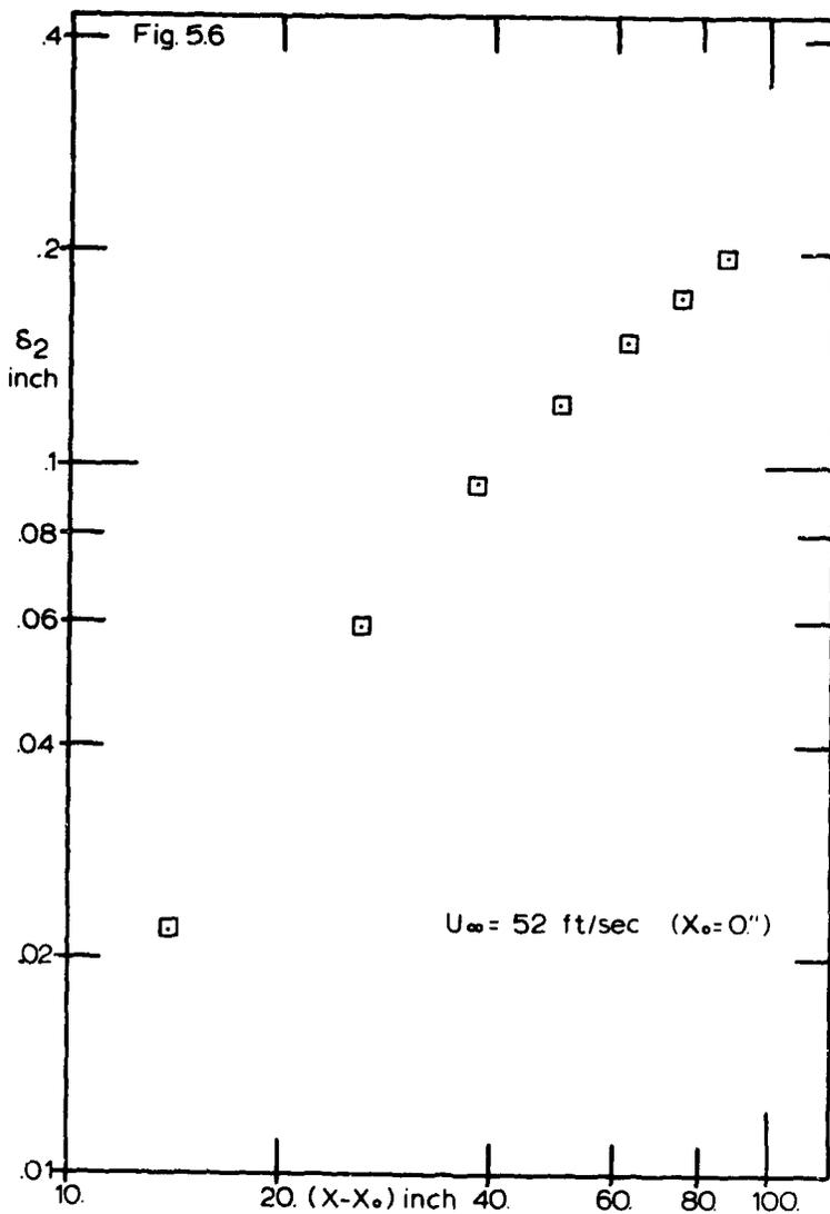
Fig. 5.6 Measured momentum thicknesses at different x-stations - transitionally rough state.
