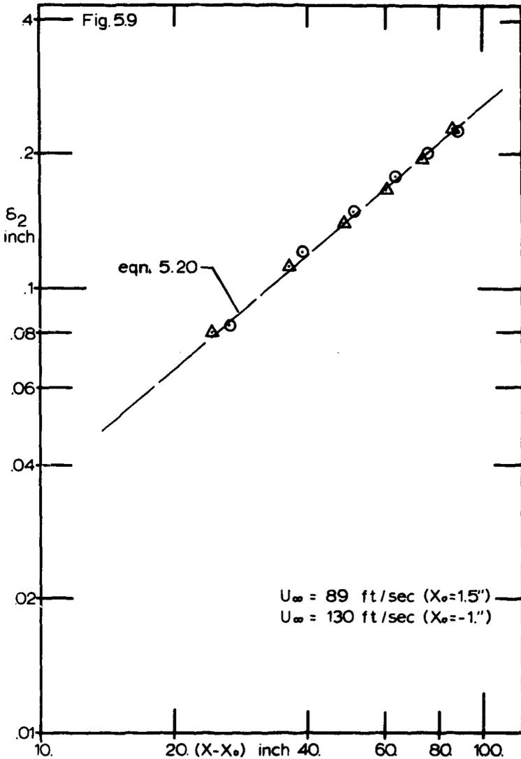
Fig. 5.9 Momentum thickness distribution for the rully rough state.
