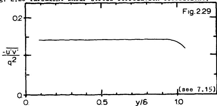
Fig. 2.29 Ratio between turbulent shear stress and turbulent kinetic energy.
