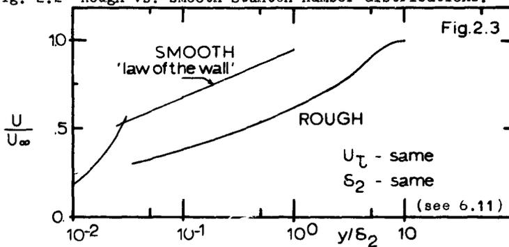
Fig. 2.3 Rough vs. smooth near wall velocity profiles.
