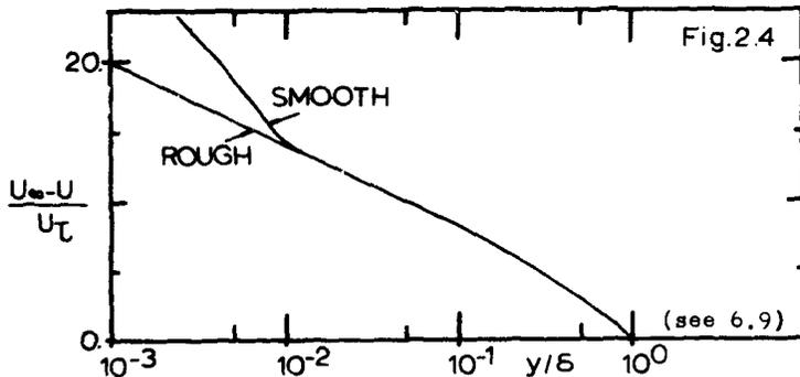
Fig. 2.4 Rough vs. smooth mean velocity defect profiles.
