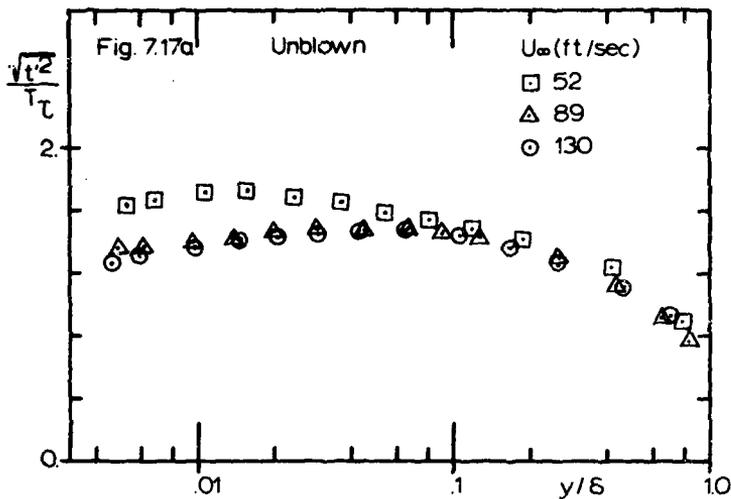
Fig. 7.17a Temperature fluctuation profiles - flows with different free-stream velocities.
