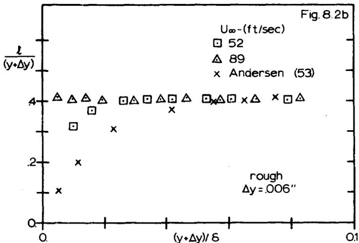
Fig. 8.2b Near wall mixing-length distributions - comparison with smooth wall data.
