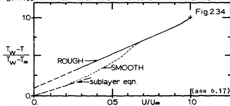
Fig. 2.34 Rough surface mean temperature-mean velocity profile.
