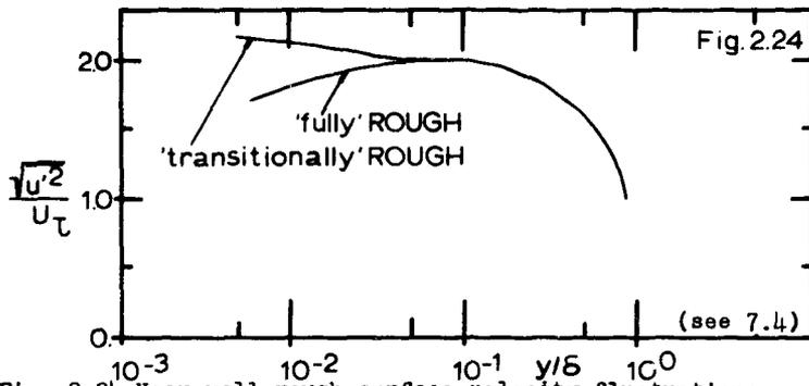
Fig. 2.24 Near wall rough surface velocity fluctuations.
