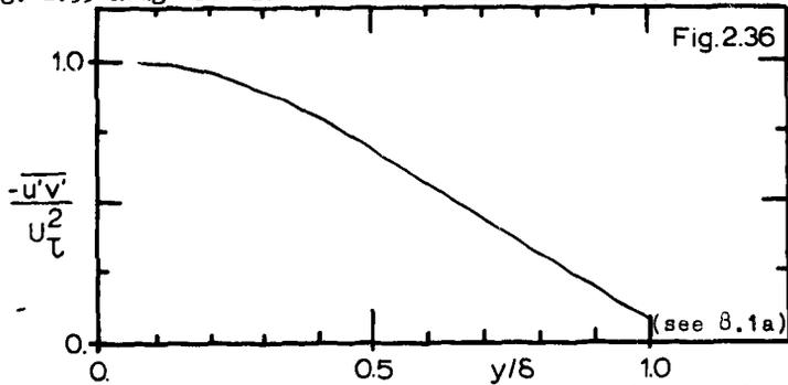
Fig. 2.36 Rough surface turbulent shear stress distribution.
