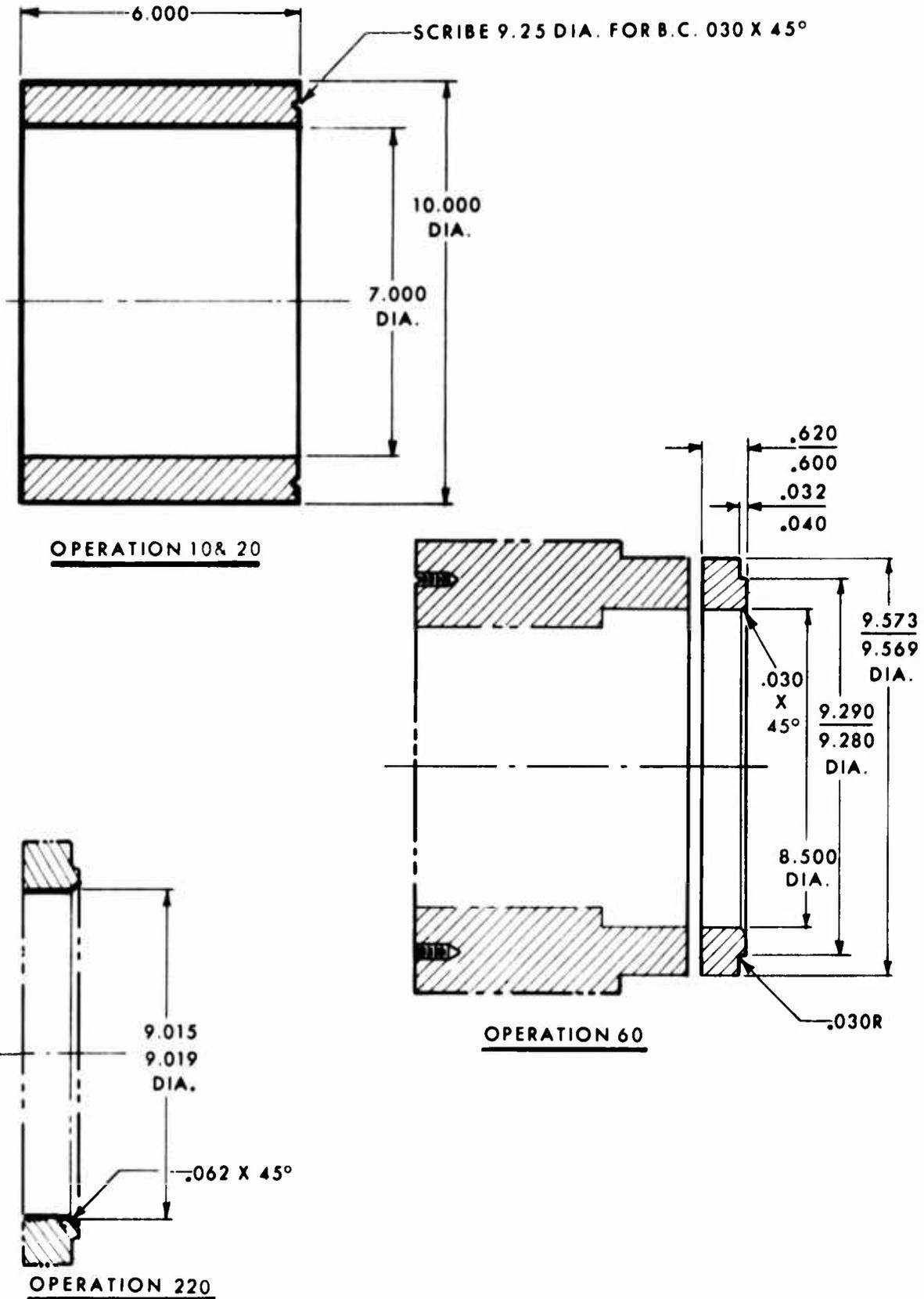
Figure C-4. RG351-11181-104 Machine Operation Drawing.
