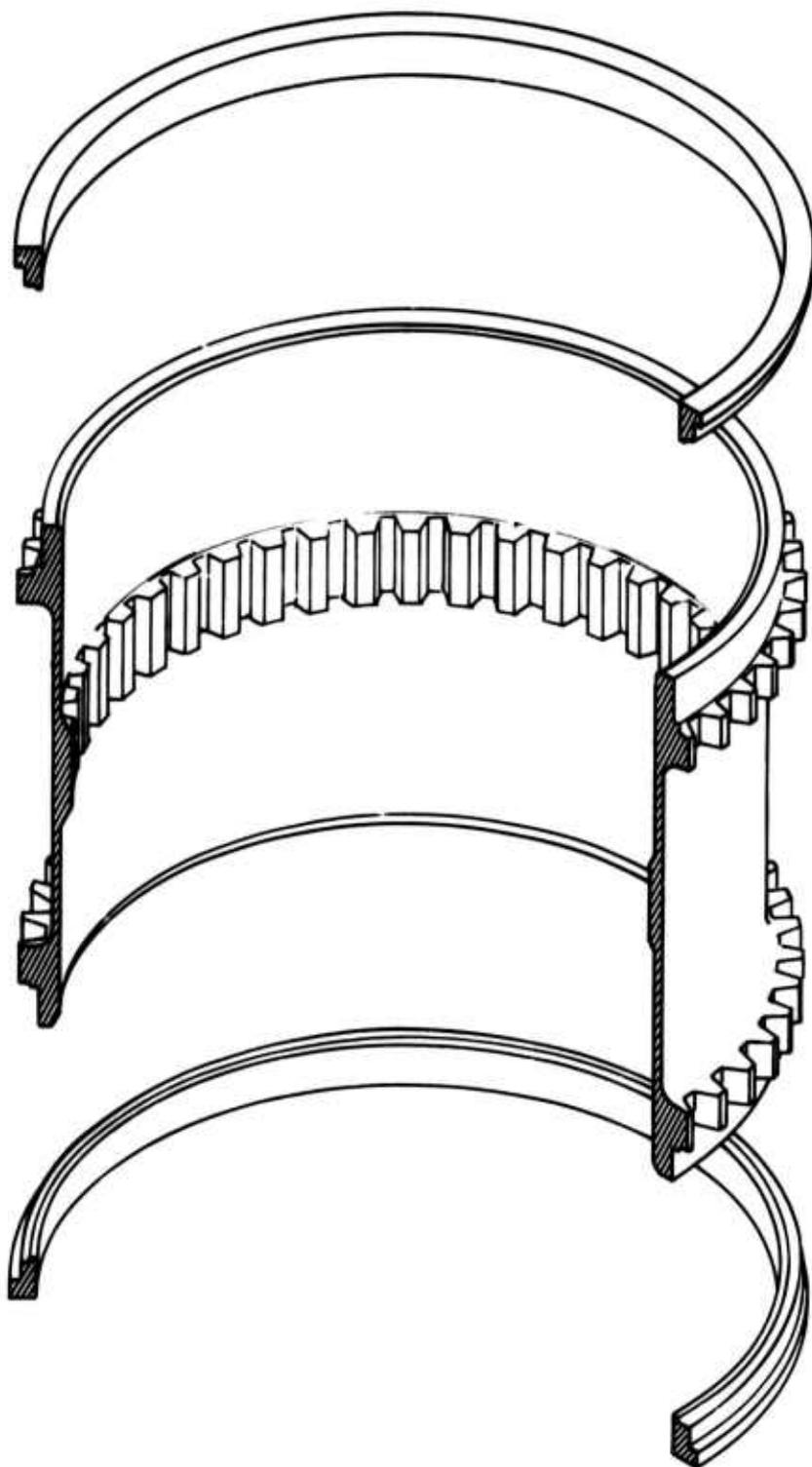
Figure 20. Sun Gear, Exploded View.
