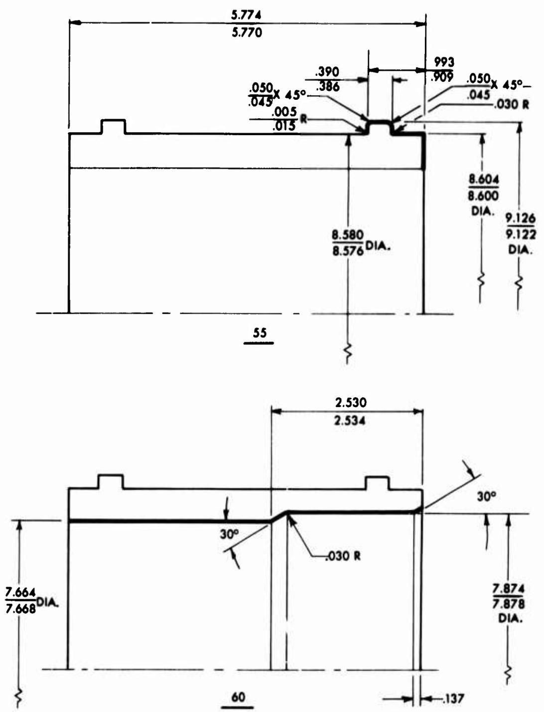
Figure F-3. RG351-11183-041, Machine Operation Drawing. (Sheet 2 of 4).
