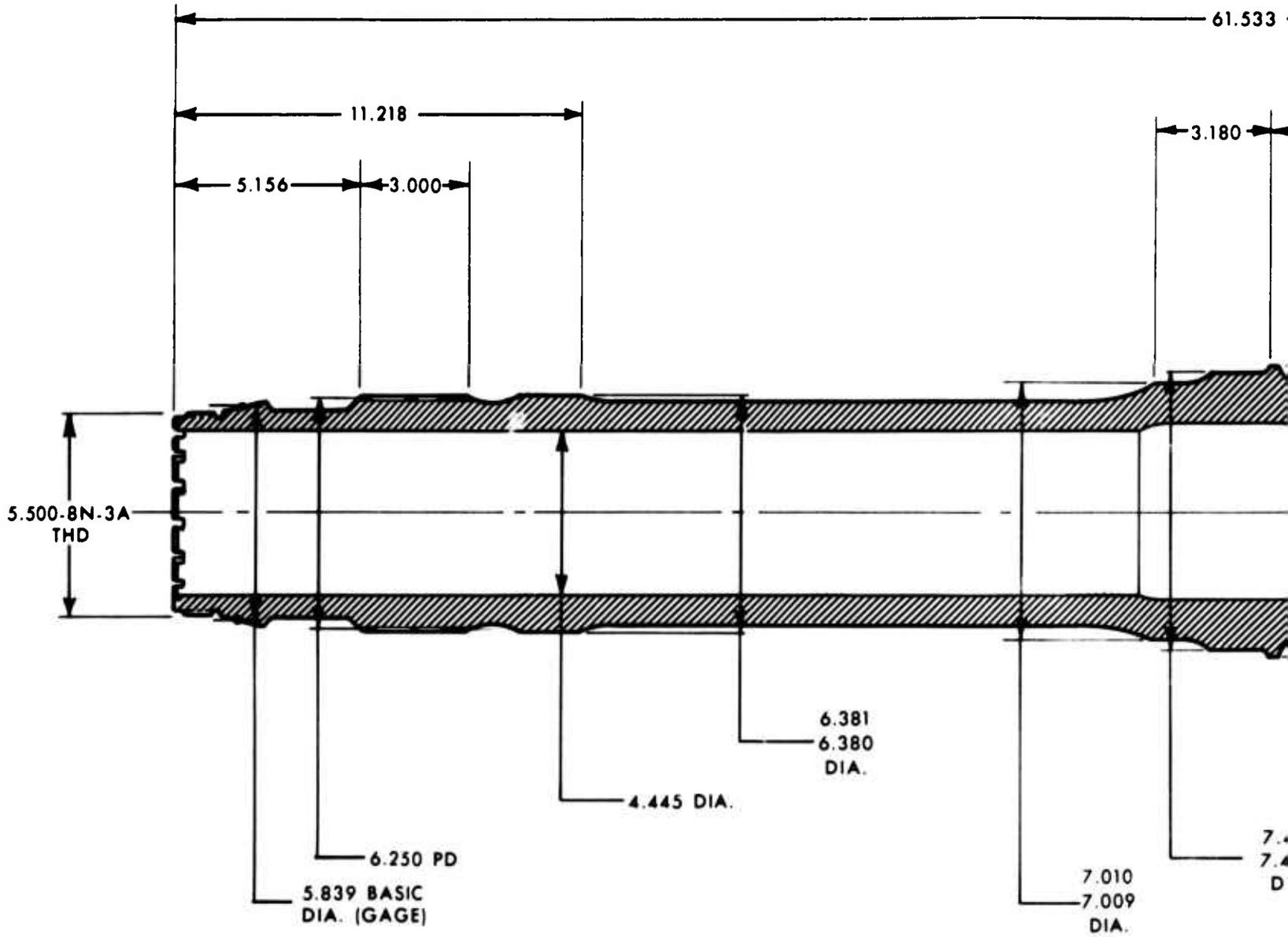
Figure 106. Main Rotor Shaft.
