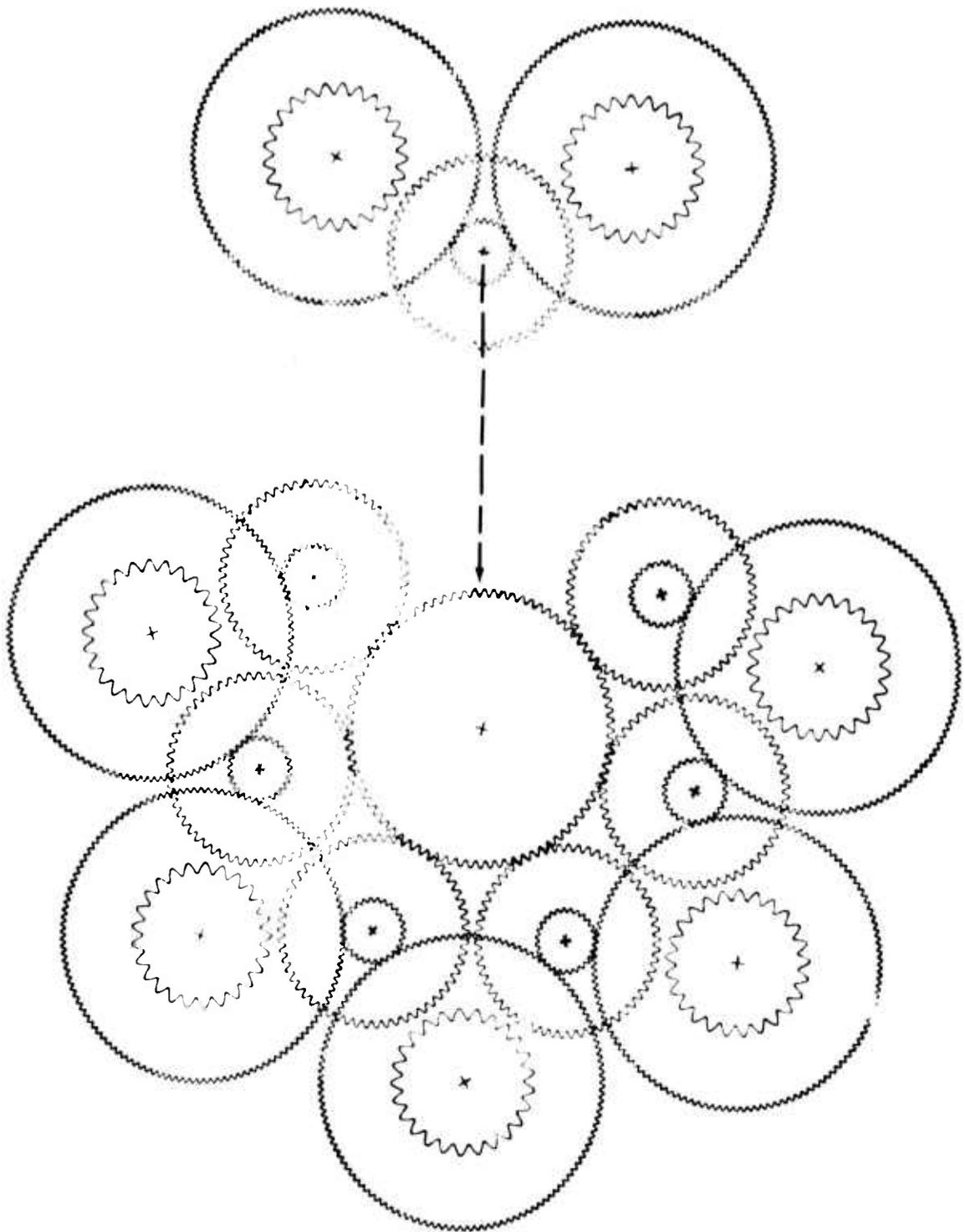
Figure 85. Roller Gear Unit Assembly, Final Step.
