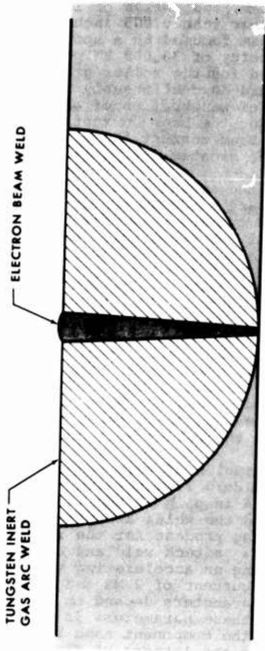
Figure 37. Comparison of Depth-to-Width Ratios of TIG and Electron beam Welding.
