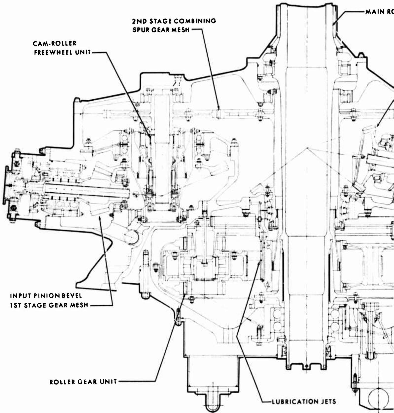
Figure 6. Cross Section of Roller Gear Transmission.
