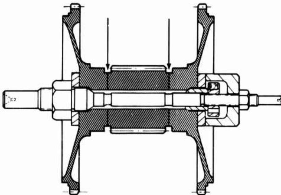
Figure 45. Welding Fixture for First-Row Pinion Butt Weld.
