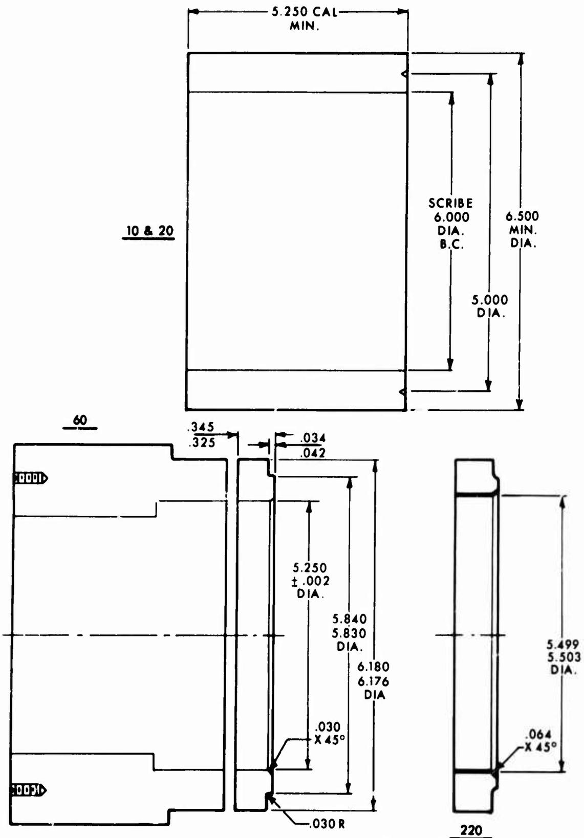
Figure E-2. RG351-11182-103, Machine Operation Drawing.
