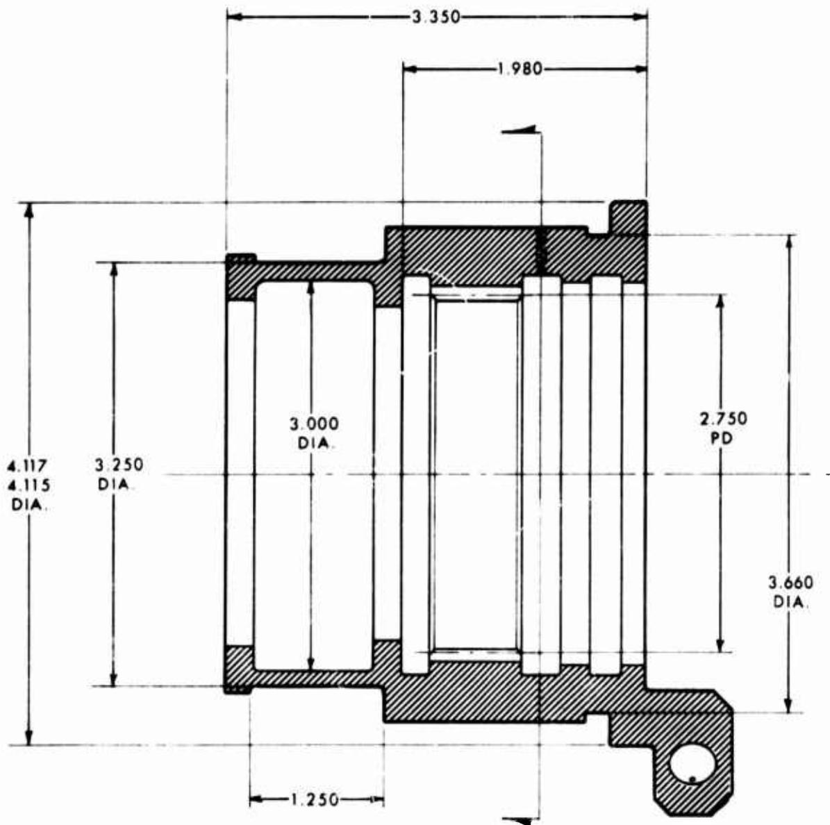
Figure 104. Freewheel Unit Cam, Dimensions.
