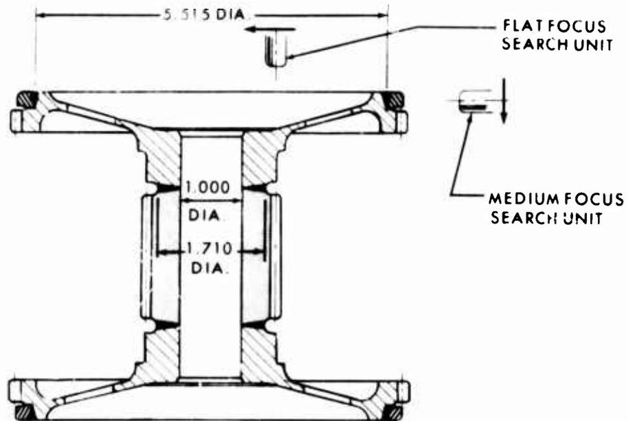
Figure A-4. Ultrasonic Inspection, First-Row Pinion.
