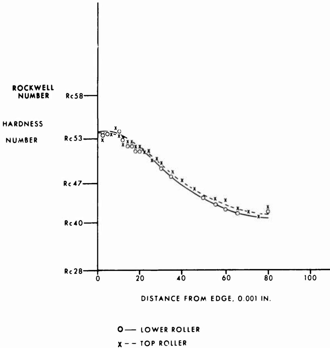
Figure 57. Microhardness Traverse Through Roller Core.
