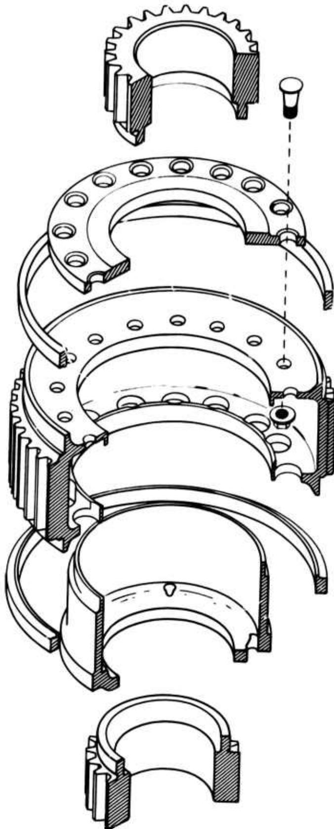
Figure 27. Second-Row Pinion, Exploded View.
