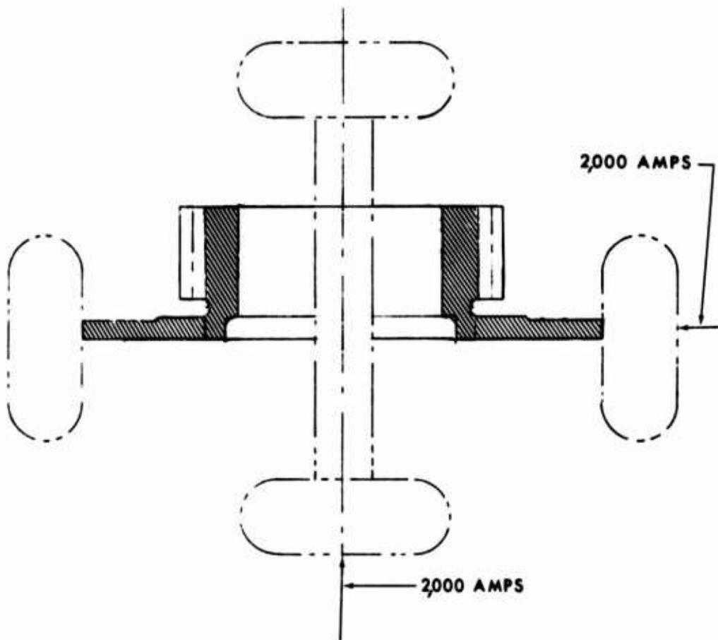
Figure 75 . Magnetization Currents and Orientation for Inspection of Second-Row Pinion, Upper Gear and Flange.
