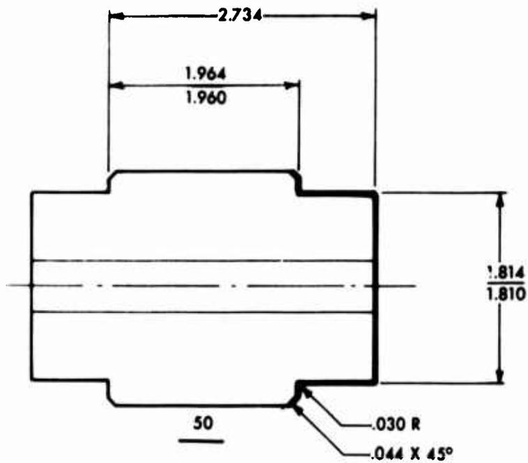
Figure E-3. RG351-11182-105, Machine Operation Drawing. (Sheet 1 of 4.)
