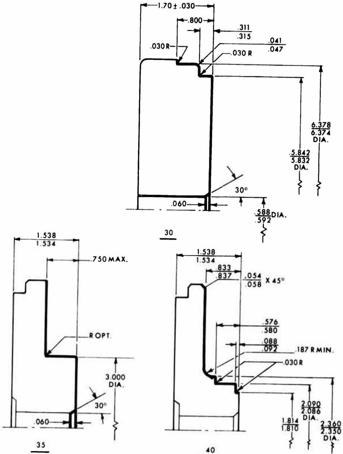
Figure E-4. RG351-11182-106, Machine Operation Drawing. (Sheet 1 of 4).
