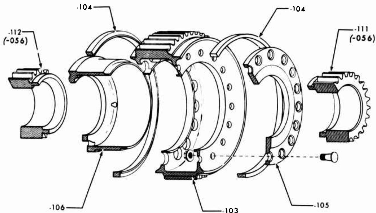
Figure C-1. Second-Row Pinion, Exploded View.
