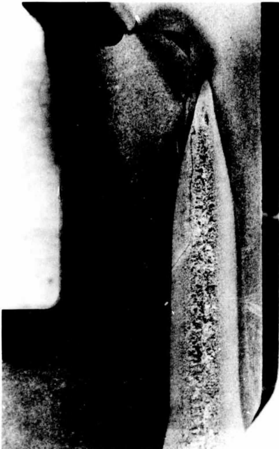
Figure 55. Cross-Sectional Sample Through First-Row Pinion Spalled Roller.
