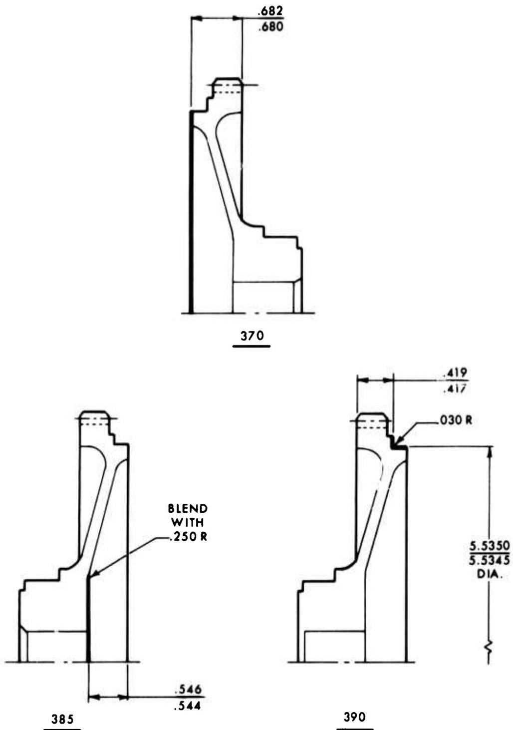
Figure E-4. RG351-11182-106, Machine Operation Drawing. (Sheet 4 of 4).
