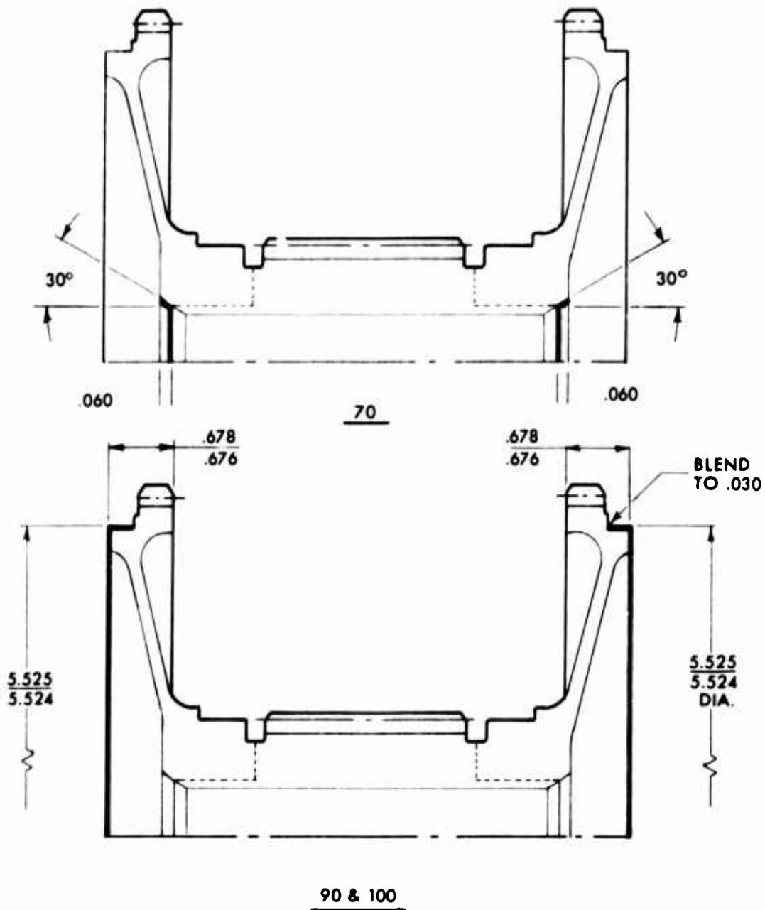
Figure E-5. RG351-11182-063, Machine Operation Drawing.
