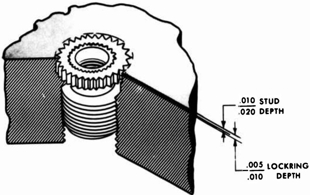
Figure 95. Rosan Insert for Main Housing.
