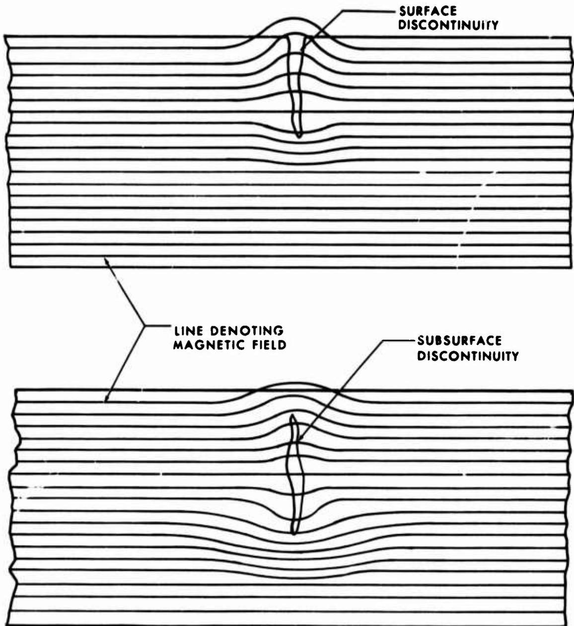
Figure 74. Effect of Discontinuities on Magnetic Field.
