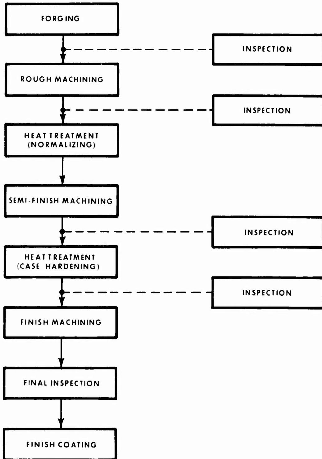
Figure 11. Basic Gear Manufacturing Process.
