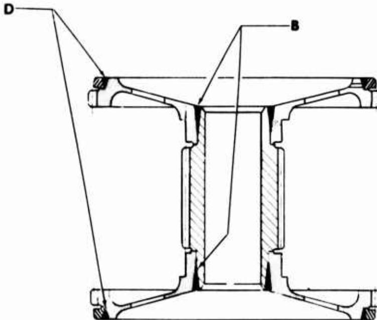
Figure 41. Assembled View of First-Row Pinion Showing Electron Beam Welds (Original Configuration).
