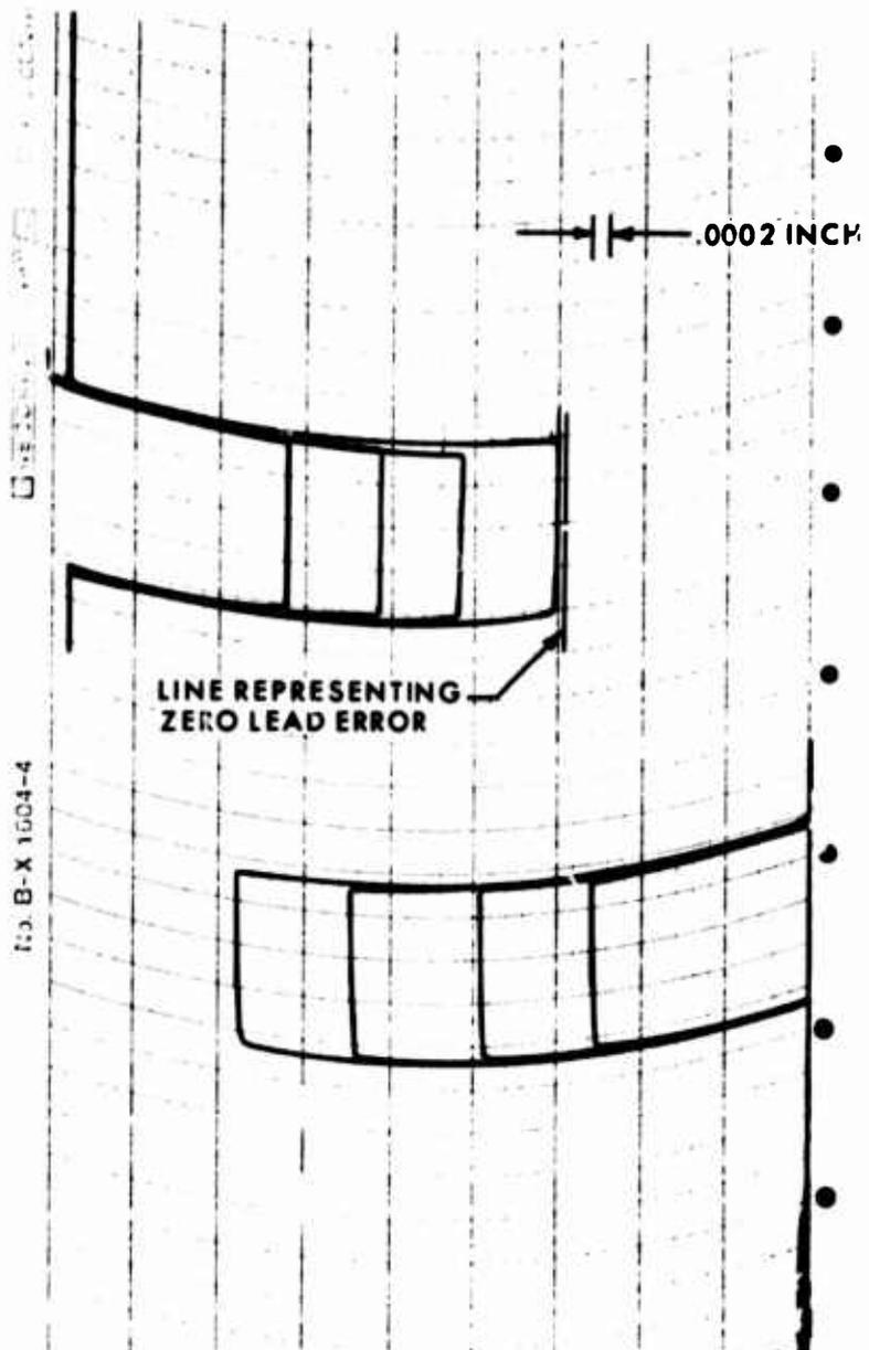
Figure 34. Lead Inspection Chart for First-Row Pinion Large Diameter Gear.
