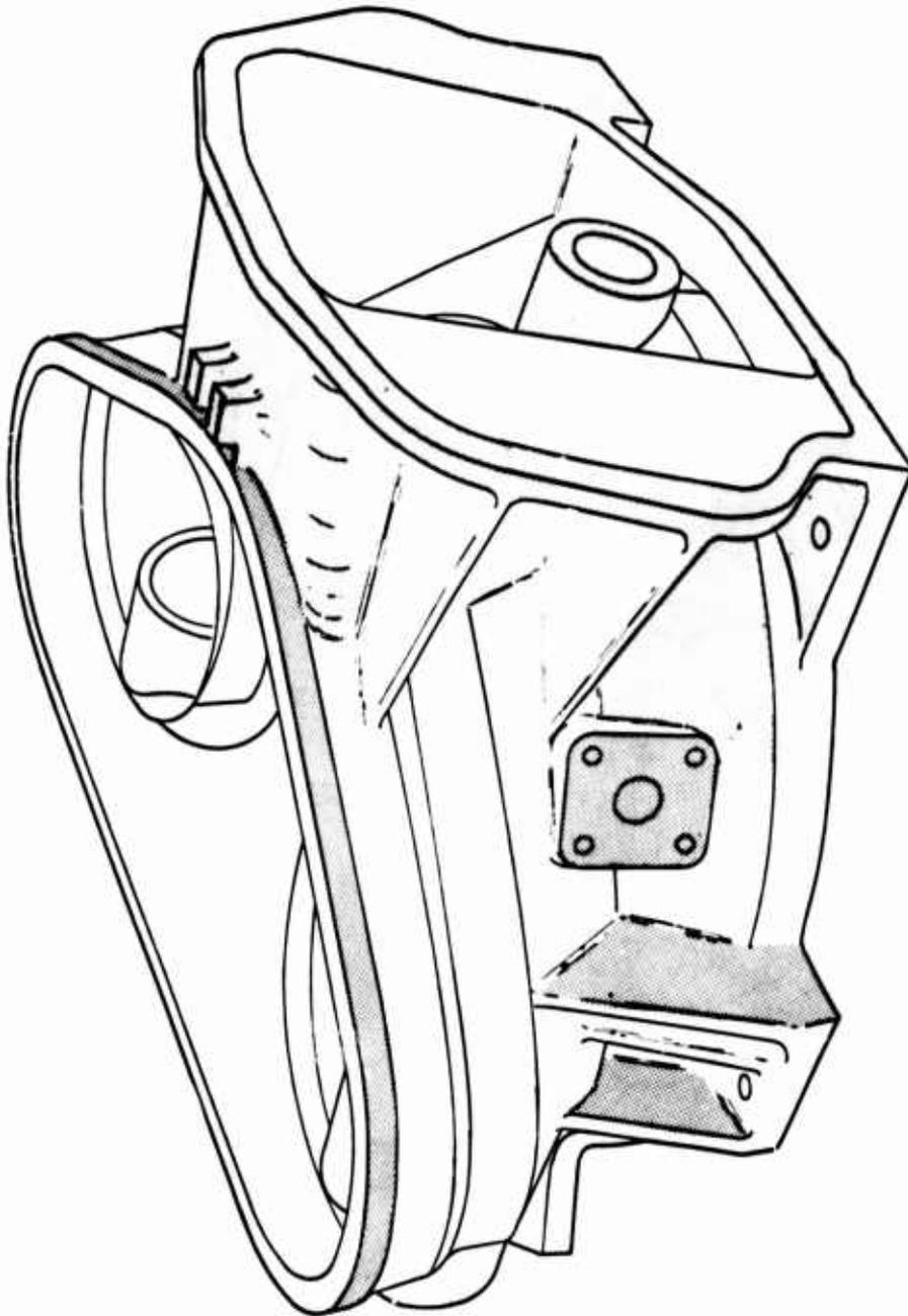
Figure 89. Critical Zones, Main Housing.
