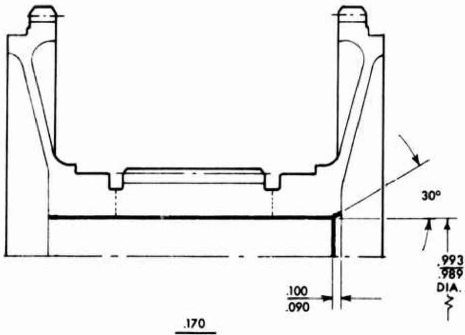
Figure E-5. RG351-11182-063, Machine Operation Drawing.
