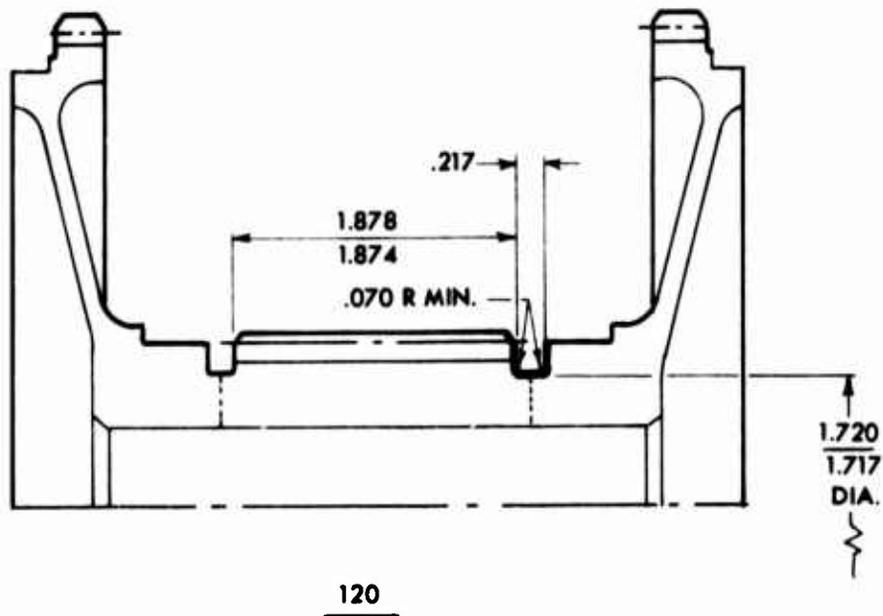
Figure E-5. RG351-11182-063, Machine Operation Drawing.
