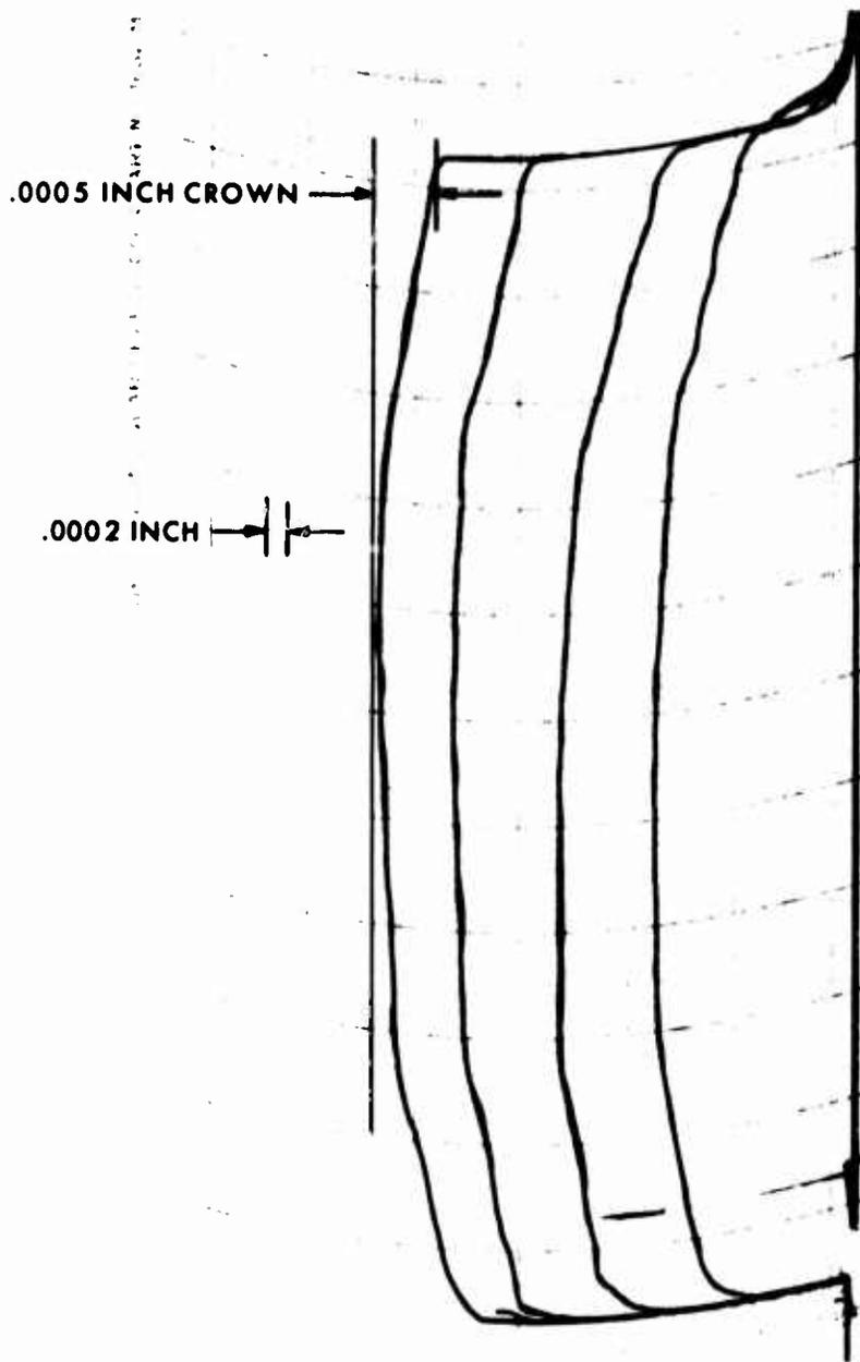
Figure 35. Crown Inspection Chart for Second-Row Pinion Large Diameter Gear.
