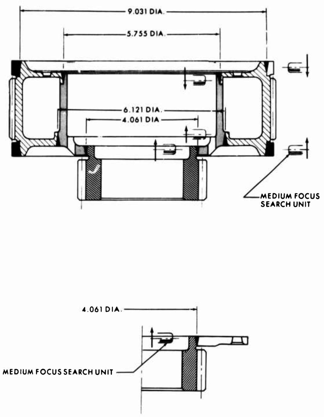
Figure A-5. Ultrasonic Inspection, Second-Row Pinion.
