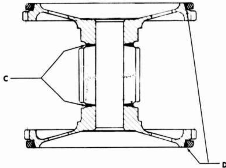
Figure 42. Assembled View of First-Row Pinion Showing Electron Beam Welds (Butt Weld Configuration).
