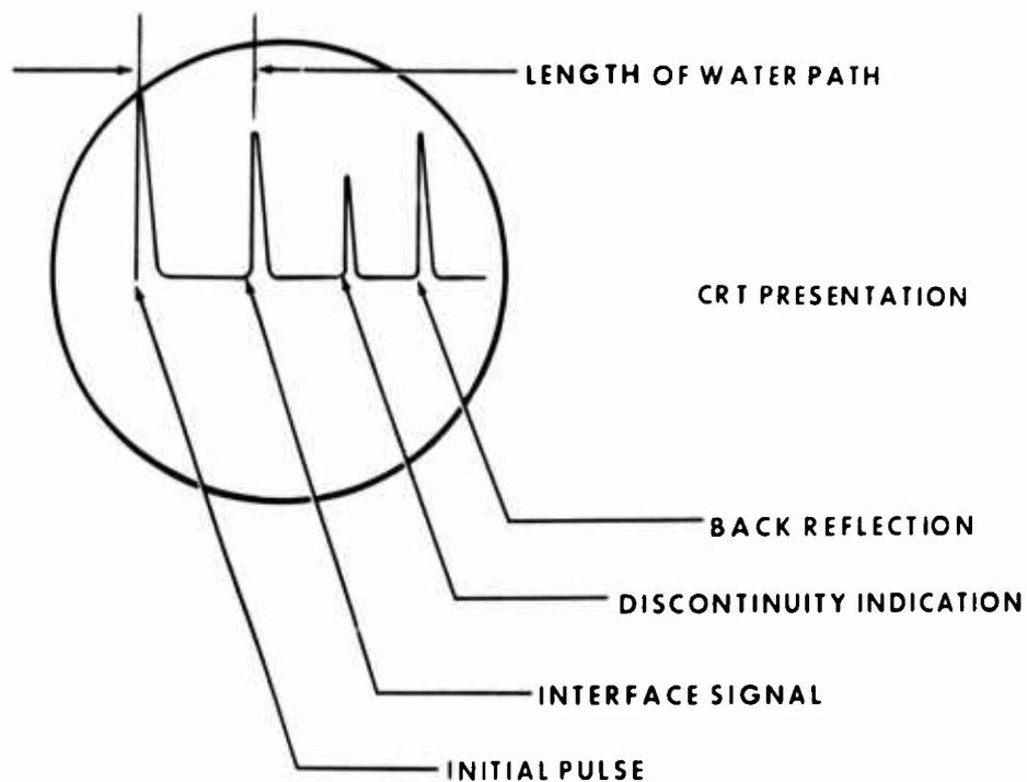
Figure 79. Ultrasonic Inspection, "A"-Scan.
