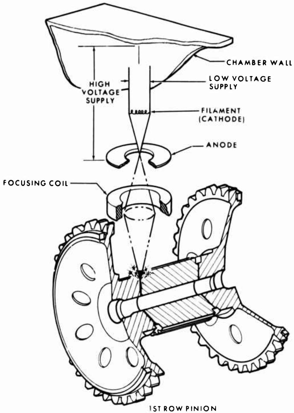
Figure 36. Electron Beam Welding Process, Schematic.
