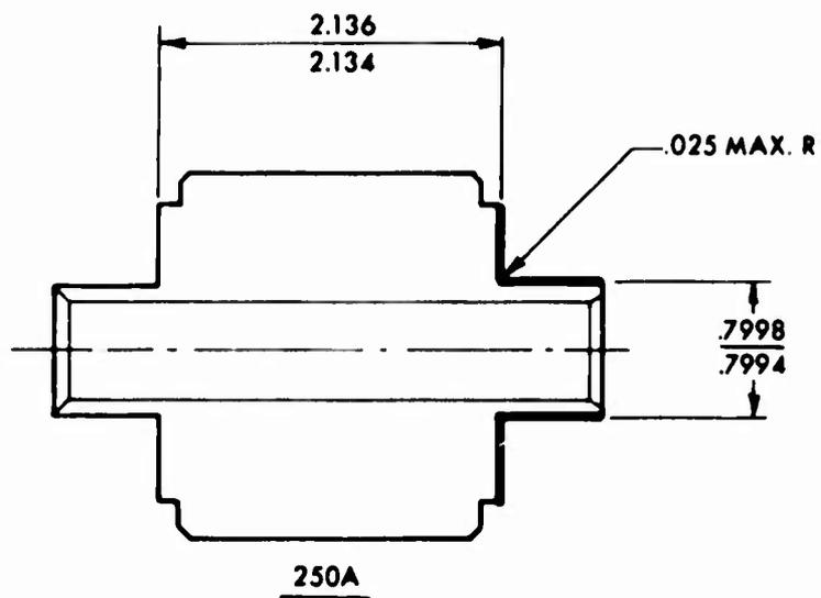
Figure E-3. RG351-11182-105, Machine Operation Drawing.
