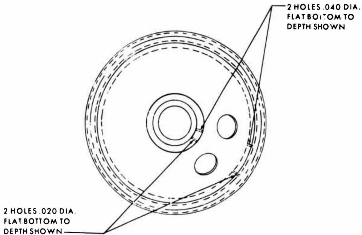
Figure A-1. Calibration Standard, Diametral Weld.
