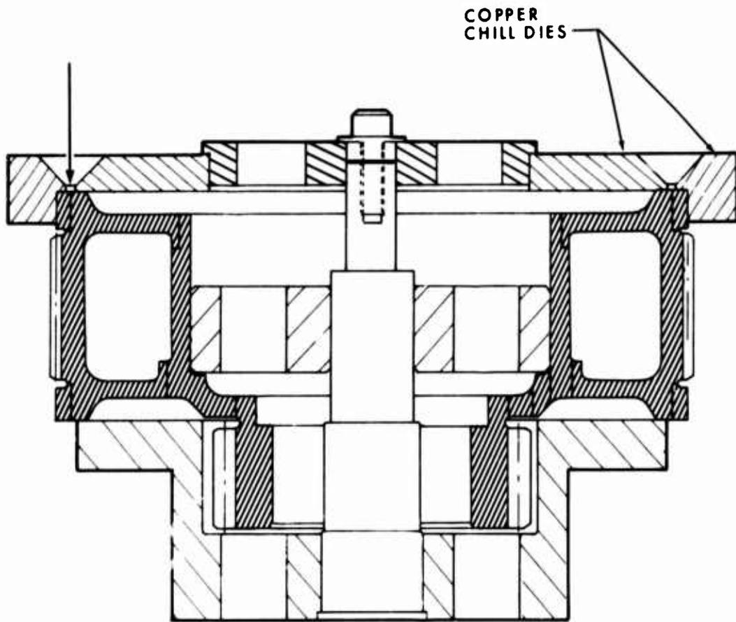
Figure 51. Welding Fixture for Second-Row Pinion Upper Roller Weld.
