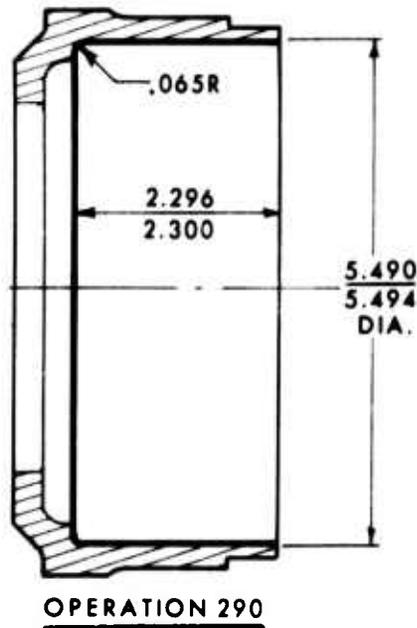
Figure C-6. RG351-11181-106 Machine Operation Drawings (Sheet 2 of 3).
