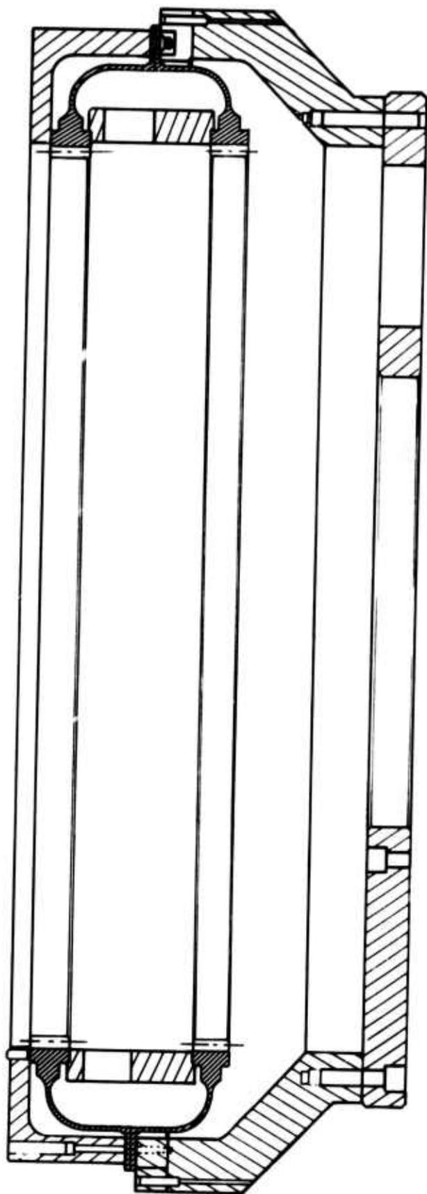
Figure 31. Ring Gear Mounted in Special Machining Fixture.
