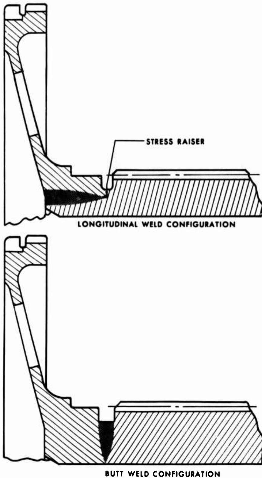
Figure 60. First-Row Pinion Weld Redesign.
