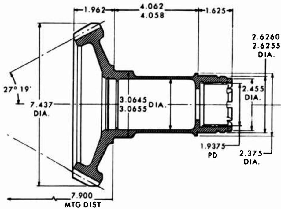
Figure 16. Dimensions, Tail Takeoff Bevel Set.
