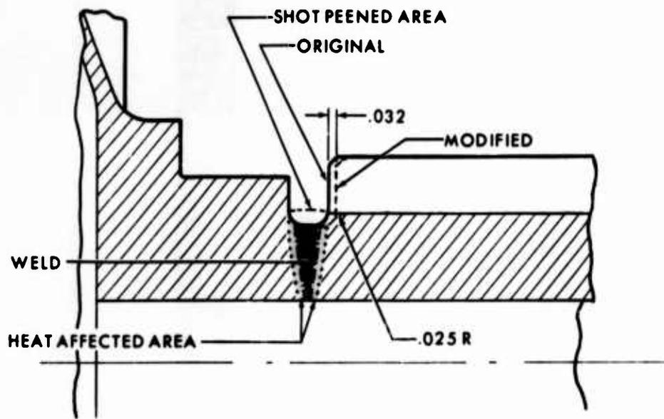
Figure 71. First-Row Pinion Rework.
