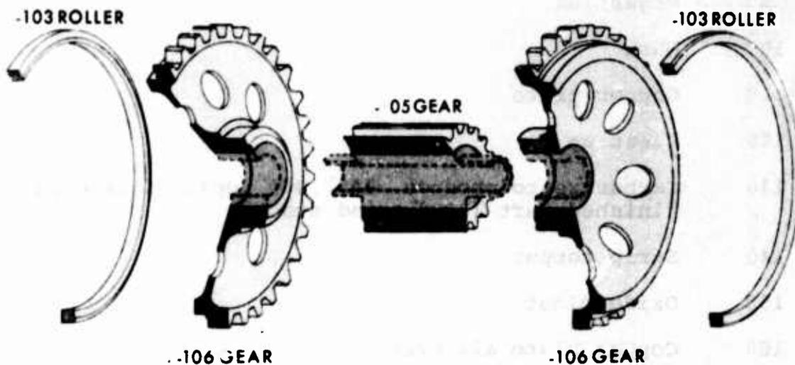
Figure E-1. Exploded View, First-Row Pinion RG351-11182.
