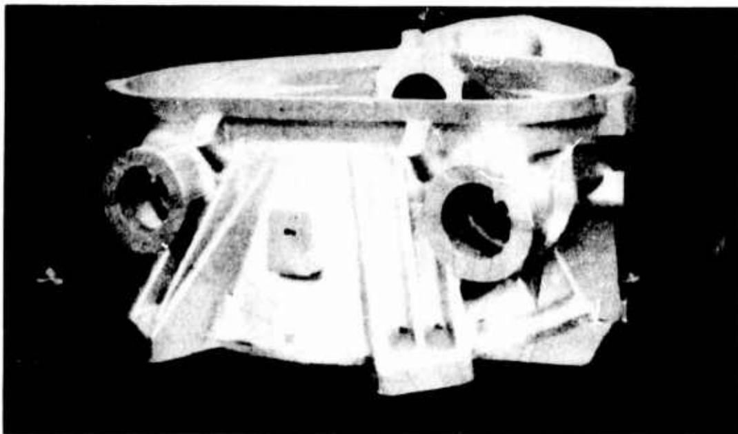
Figure 92. Completed Main Housing Casting.
