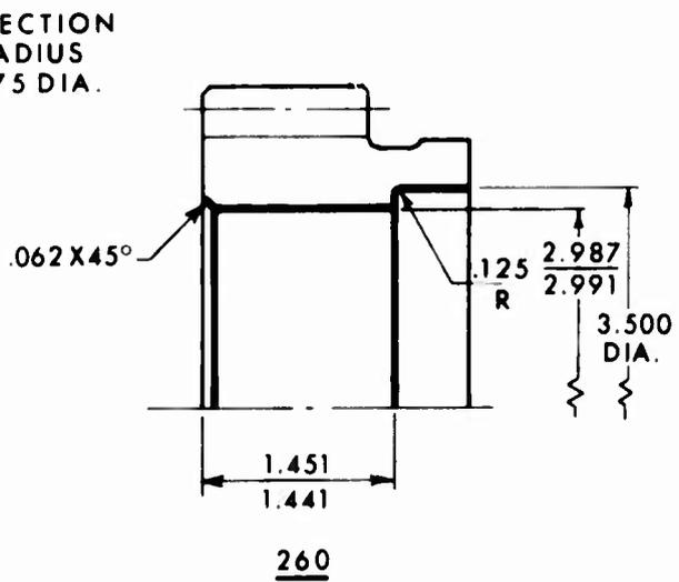
Figure D-6, RG351-11278-046: Machine Operation Drawing.
