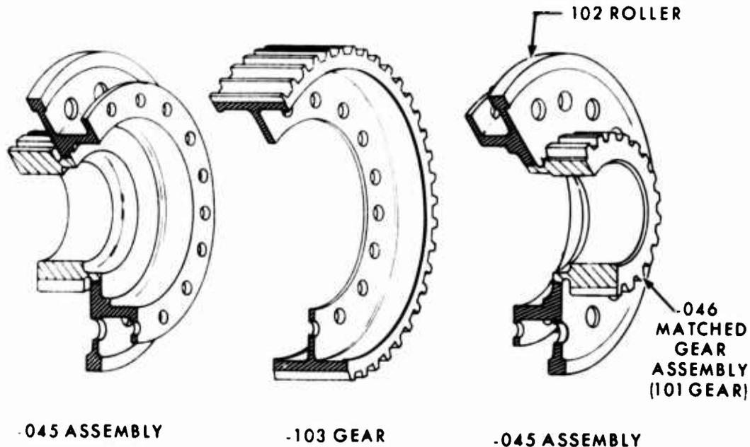
Figure D-2. Exploded View, Second-Row Pinion RG351-11278.
