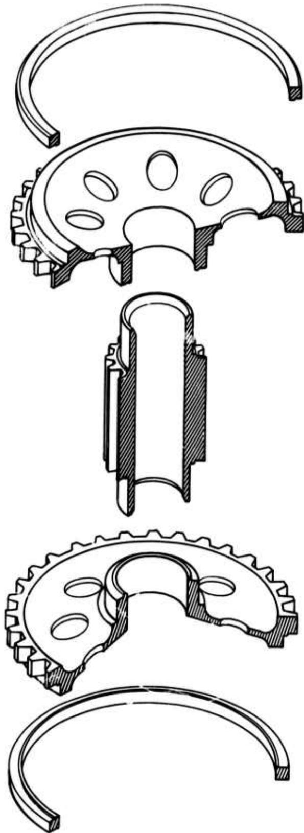
Figure 23. First-Row Pinion, Exploded View.
