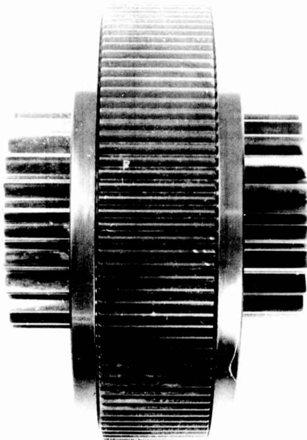
Figure 28. Roller Gear Drive Second-Row Pinion.
