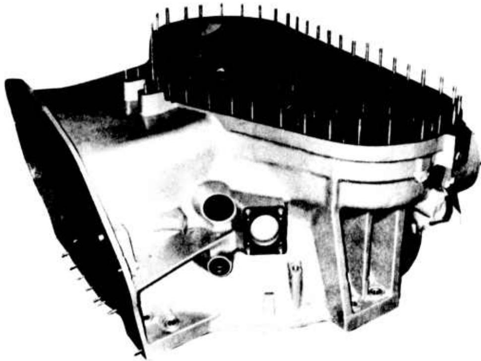
Figure 96. Main Housing With Liner and Studs.
