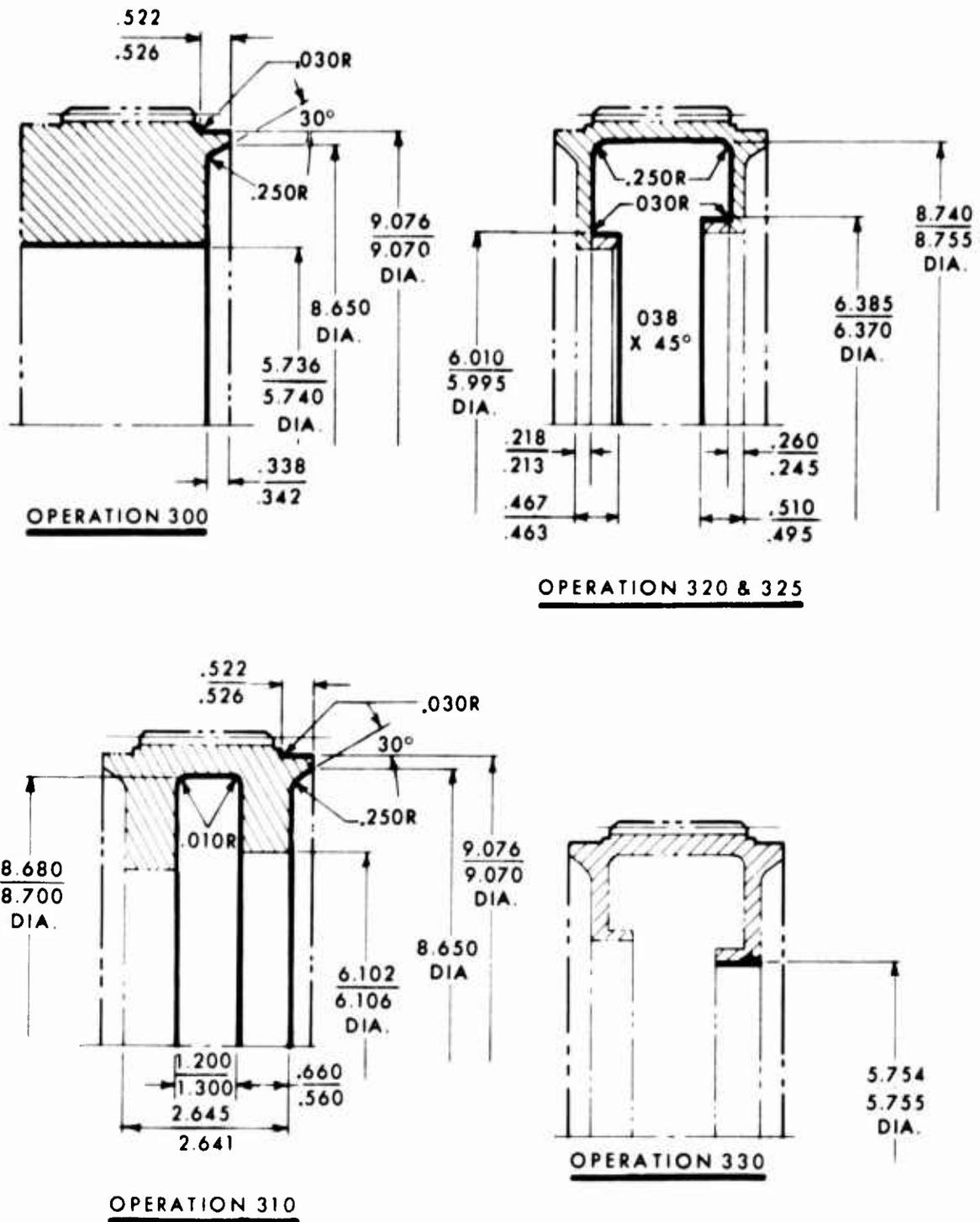
Figure C-3. RG351-11181-103 Machine Operation Drawings (Sheet 2 of 3).
