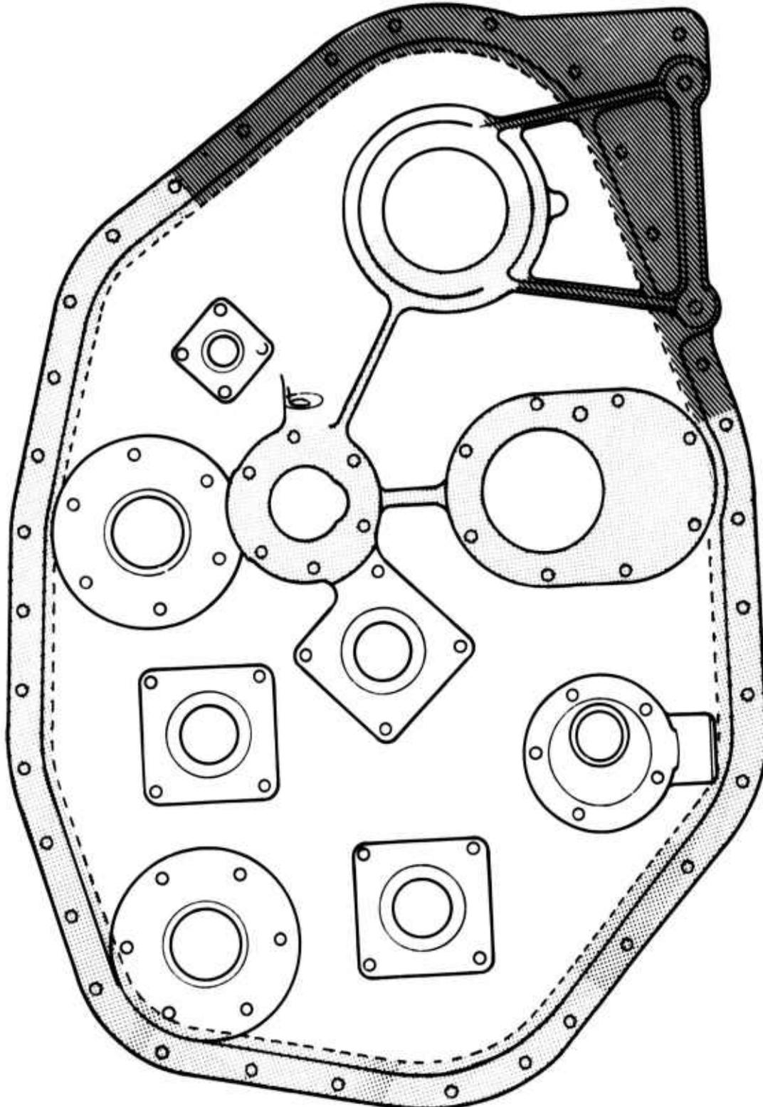
Figure 10u. Critical Zones, Rear Cover Outboard.
