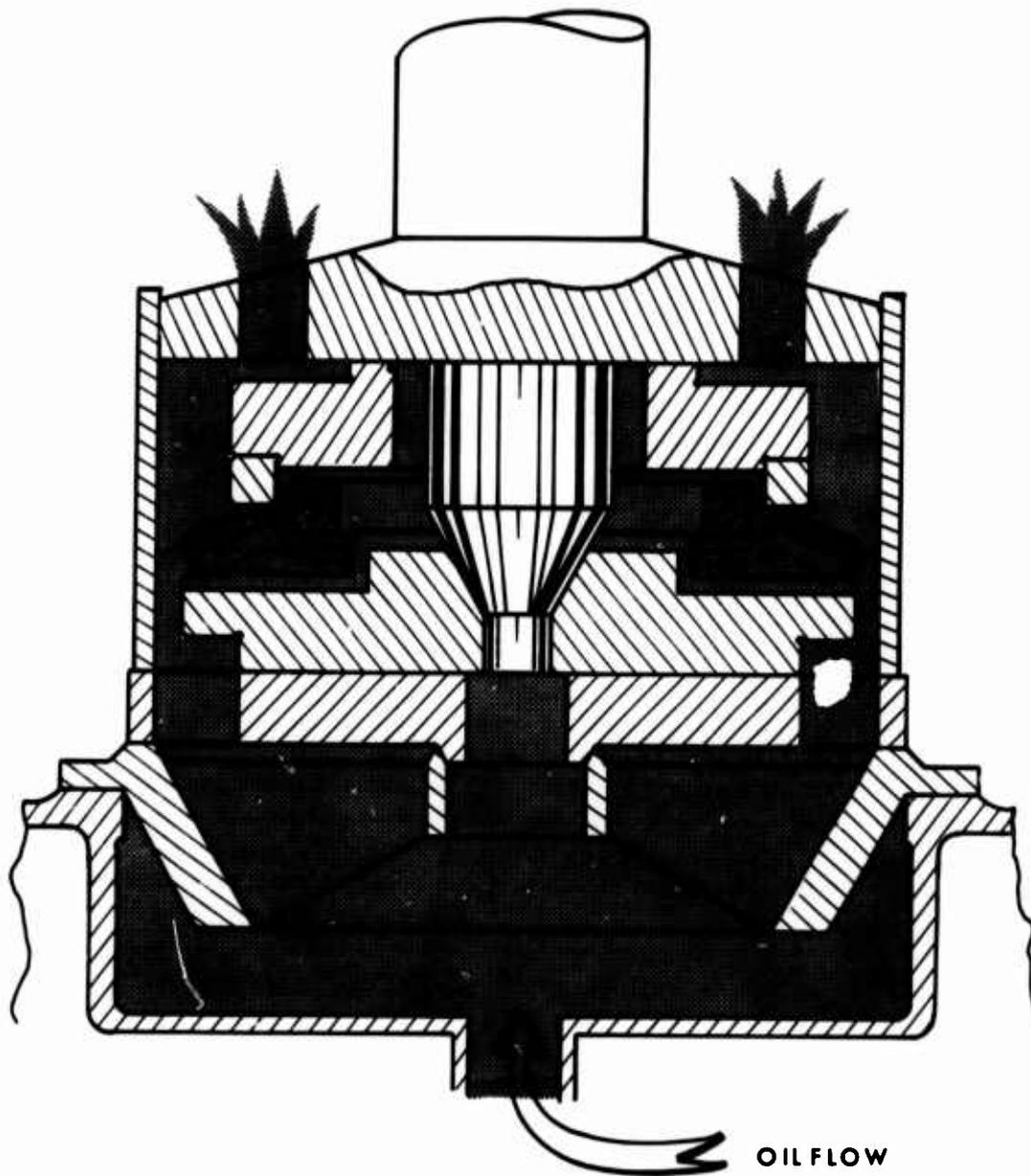
Figure 12. Input Bevel Gear Quench Press.
