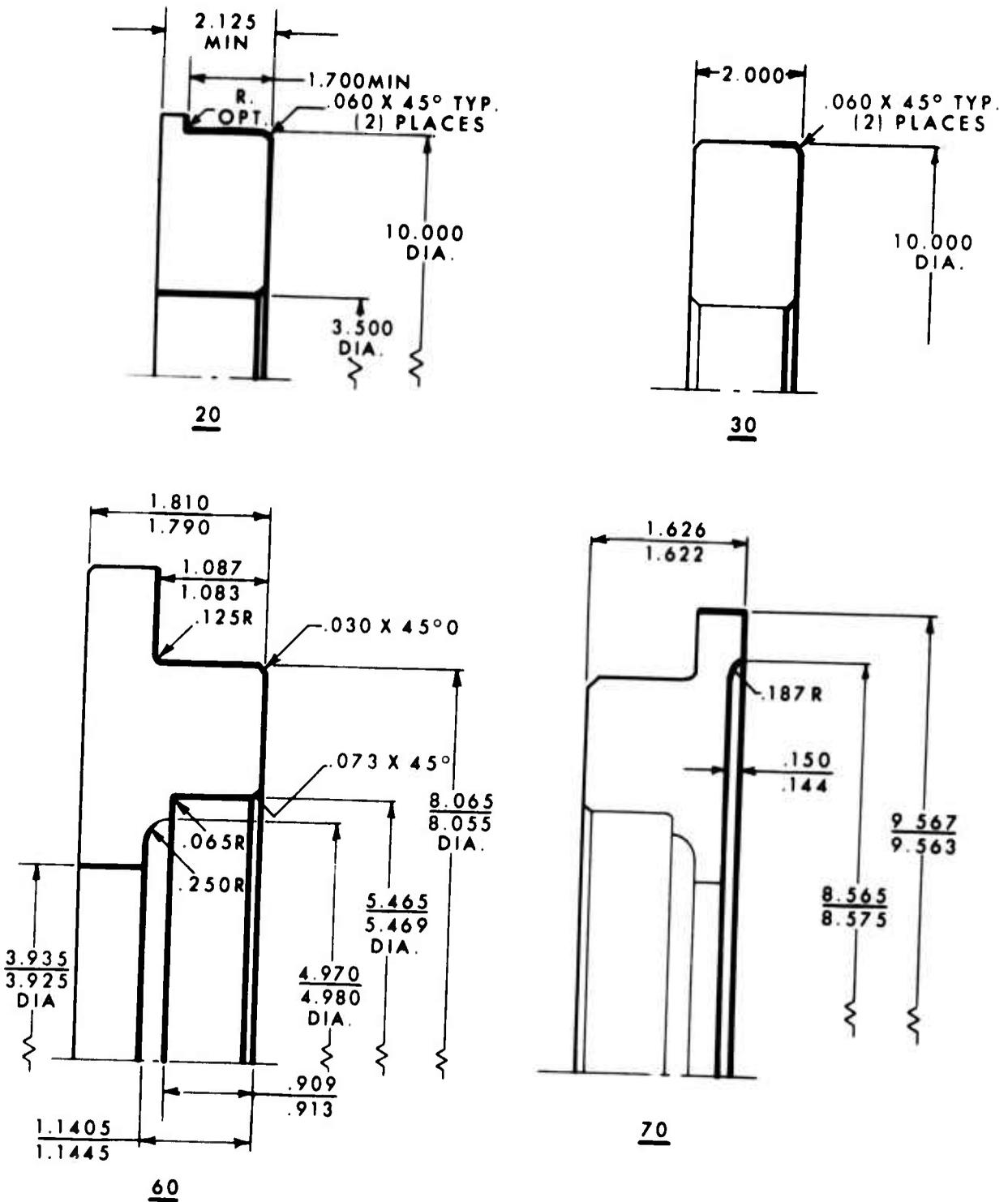
Figure D-4. RG351-11278-102: Machine Operation Drawing
