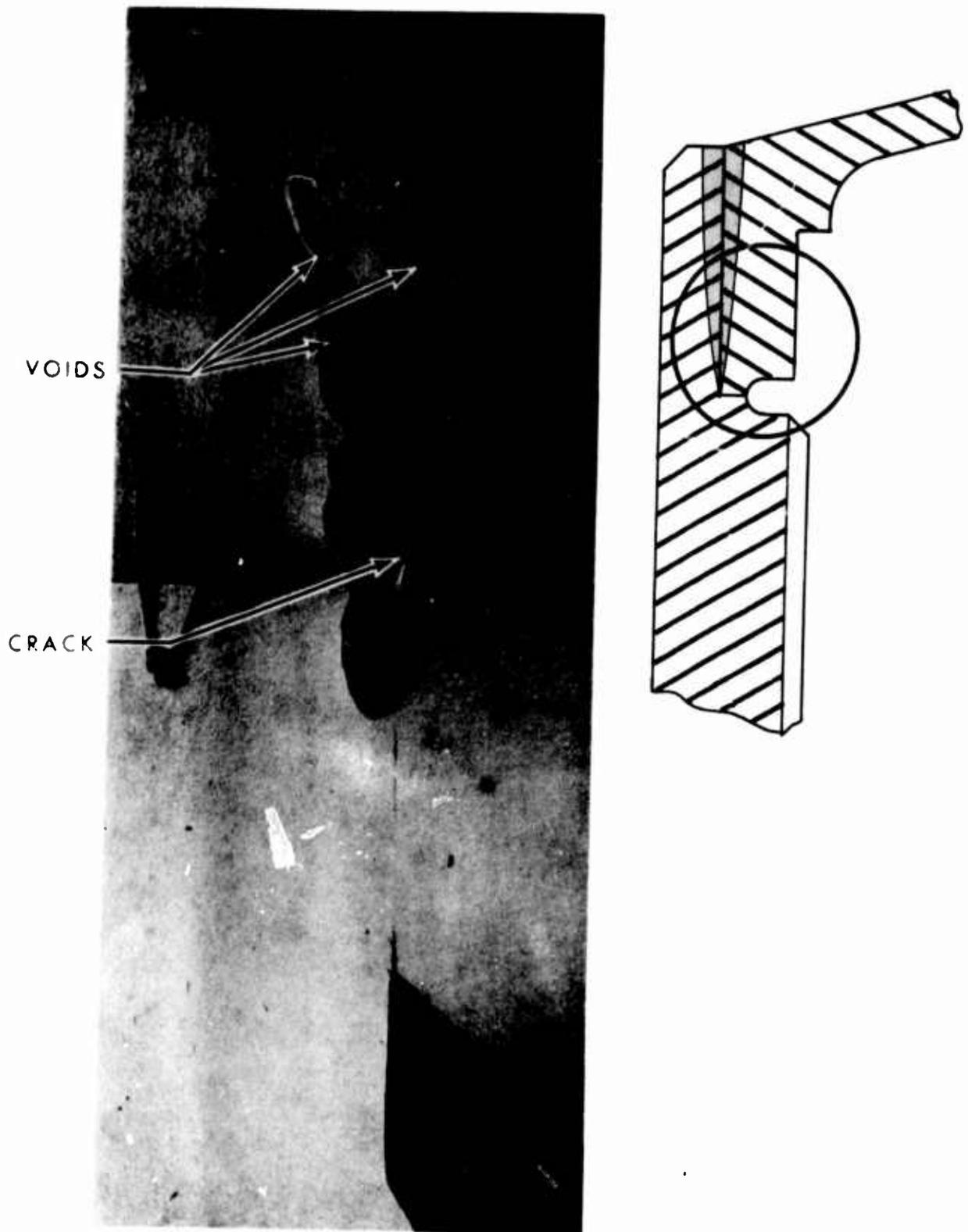
Figure 56. Metallographic Inspection of First-Row Pinions Revealing Voids at Weld Line.
