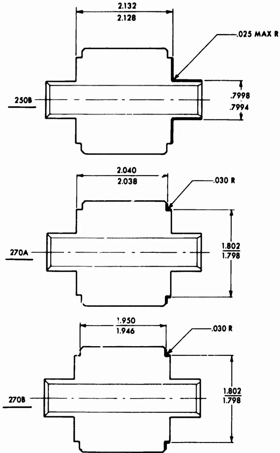
Figure E-3. RG351-11182-105, Machine Operation Drawing.
