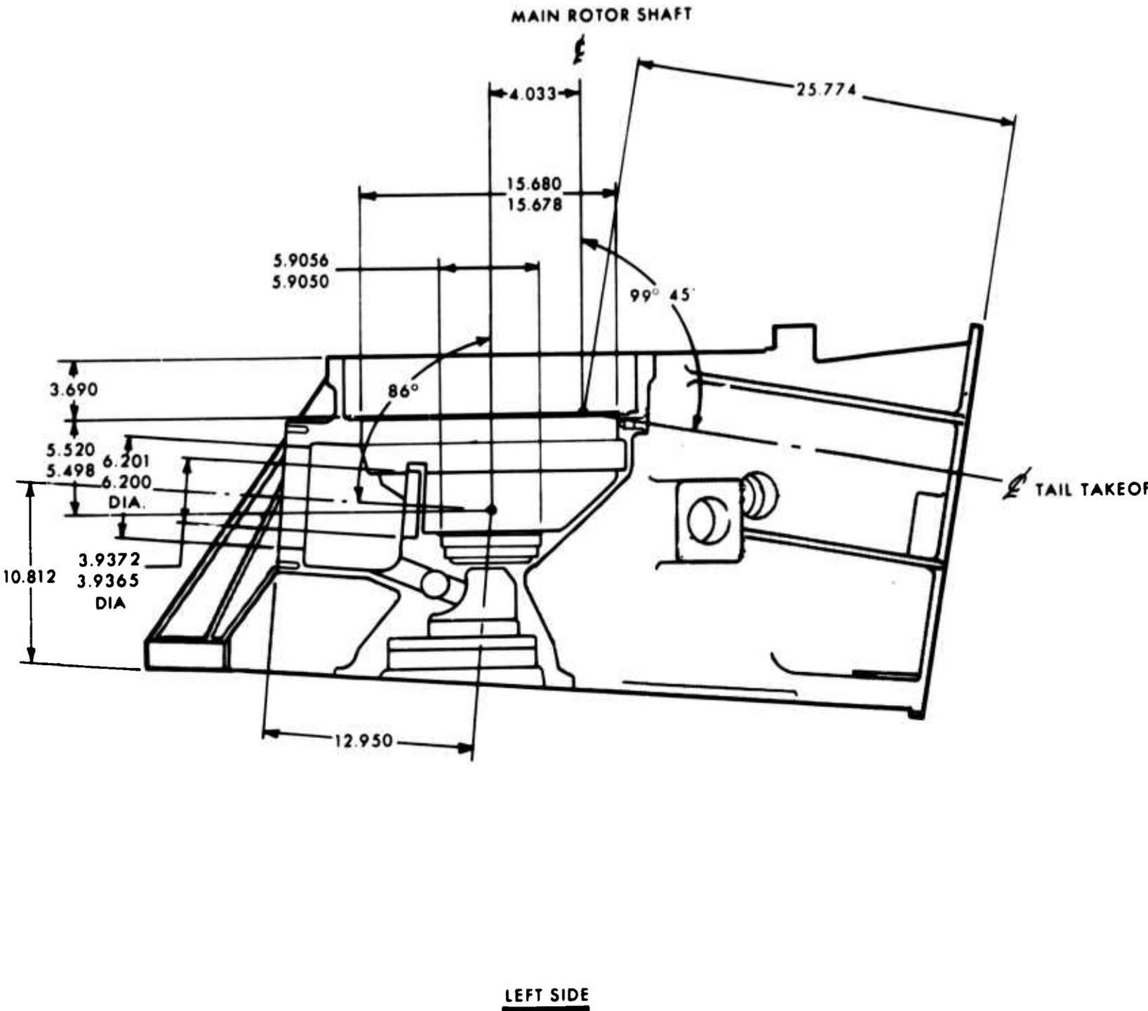
Figure 93. Main Housing, Critical Dimensions.
