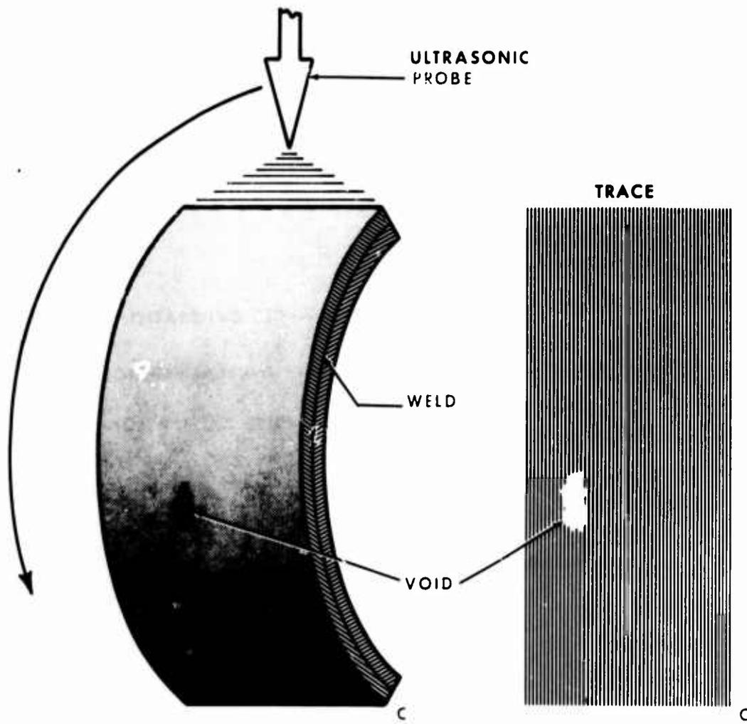
Figure 81. C-Scan Display of Inspection Trace.
