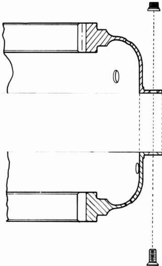
Figure 30. Ring Gear, Exploded View.
