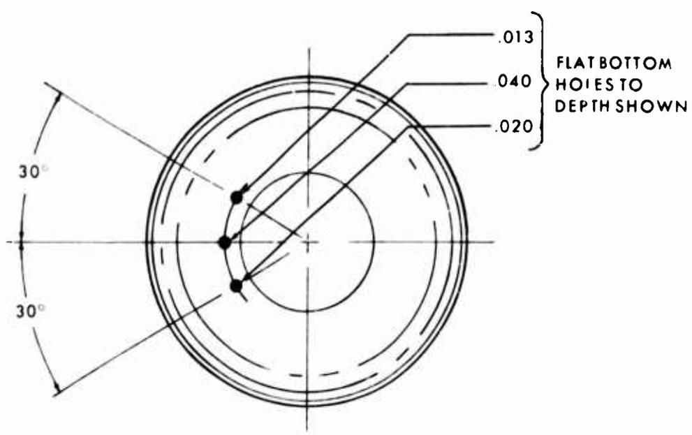
Figure A-2. Calibration Standard, Butt Weld.
