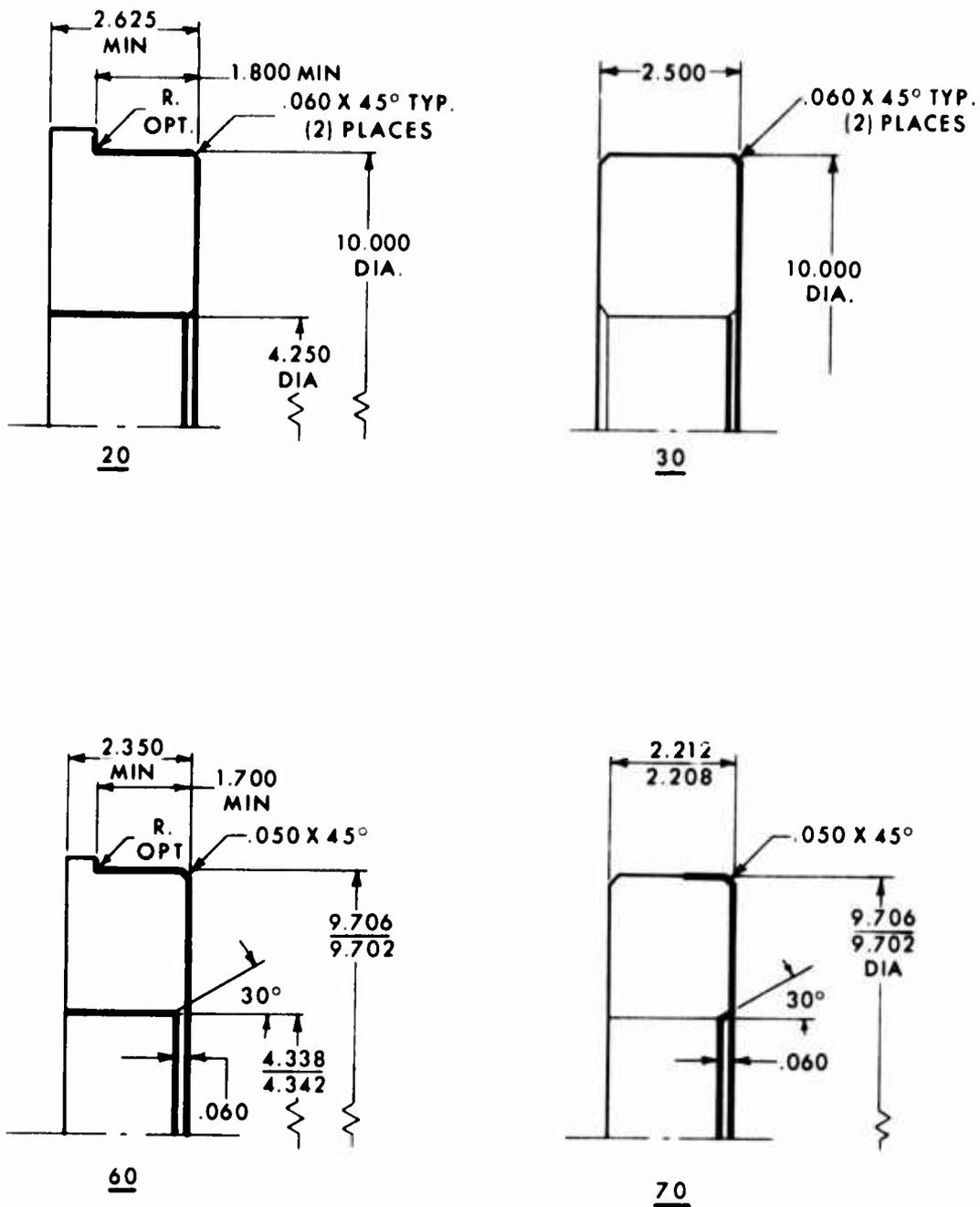
Figure D-5, RG351-11278-103: Machine Operation Drawing (Sheet 1 of 2).
