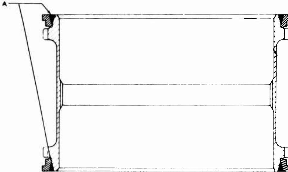
Figure 40. Assembled View of Sun Gear Showing Electron Beam Welds.
