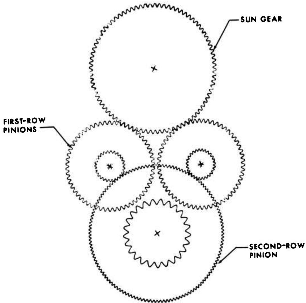
Figure 84. Roller Gear Unit Assembly, Step Two.
