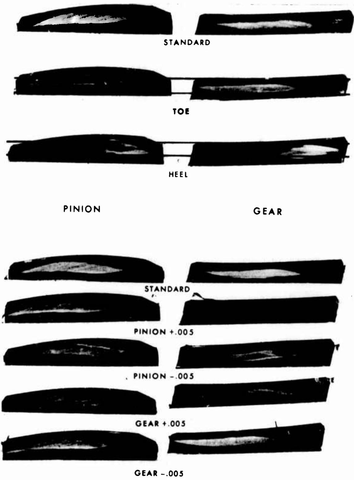
Figure 17. Bearing Patterns of Input Spiral Bevel Set.
