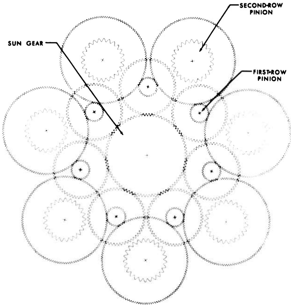
Figure 9. Roller Gear Component Arrangement.
