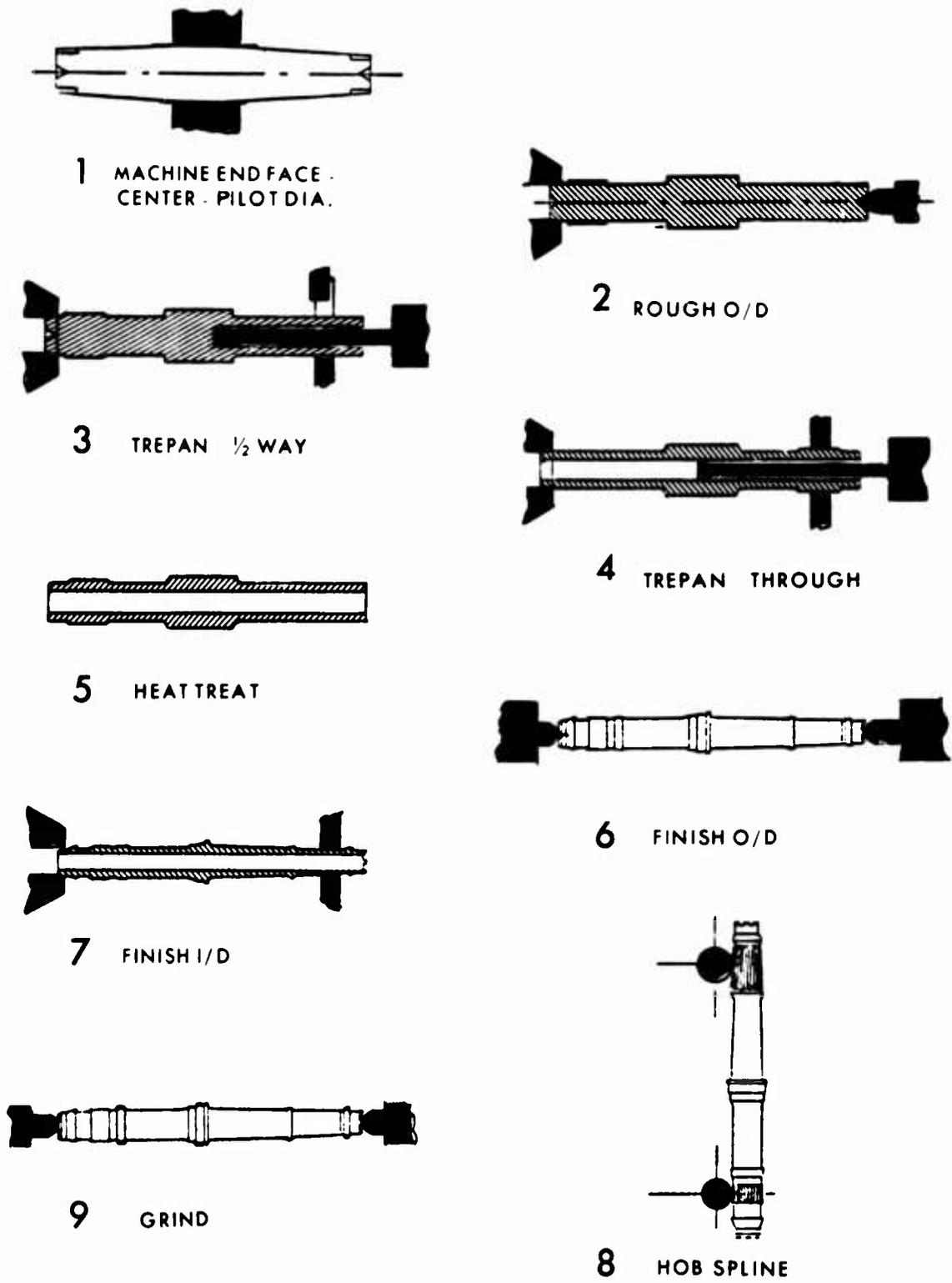
Figure 105. Main Rotor Shaft Manufacturing Process.
