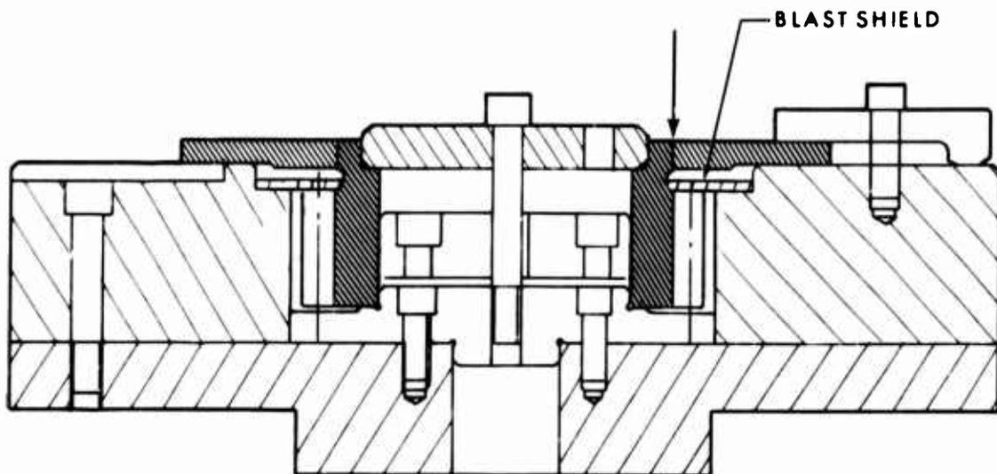
Figure 52. Welding Fixture for Second-Row Pinion Upper Gear to Plate Weld.
