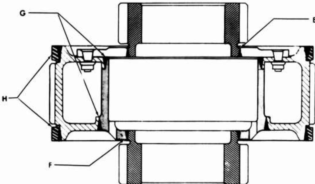
Figure 43. Assembled View of Second-Row Pinion Showing Electron Beam Welds.
