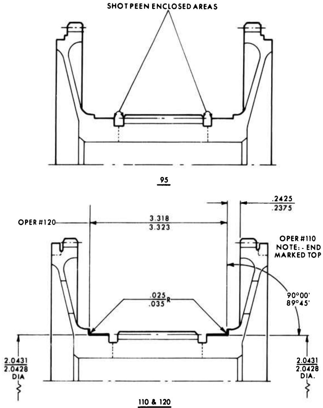
Figure E-6. RG351-11182-061, Machine Operation Drawing.
