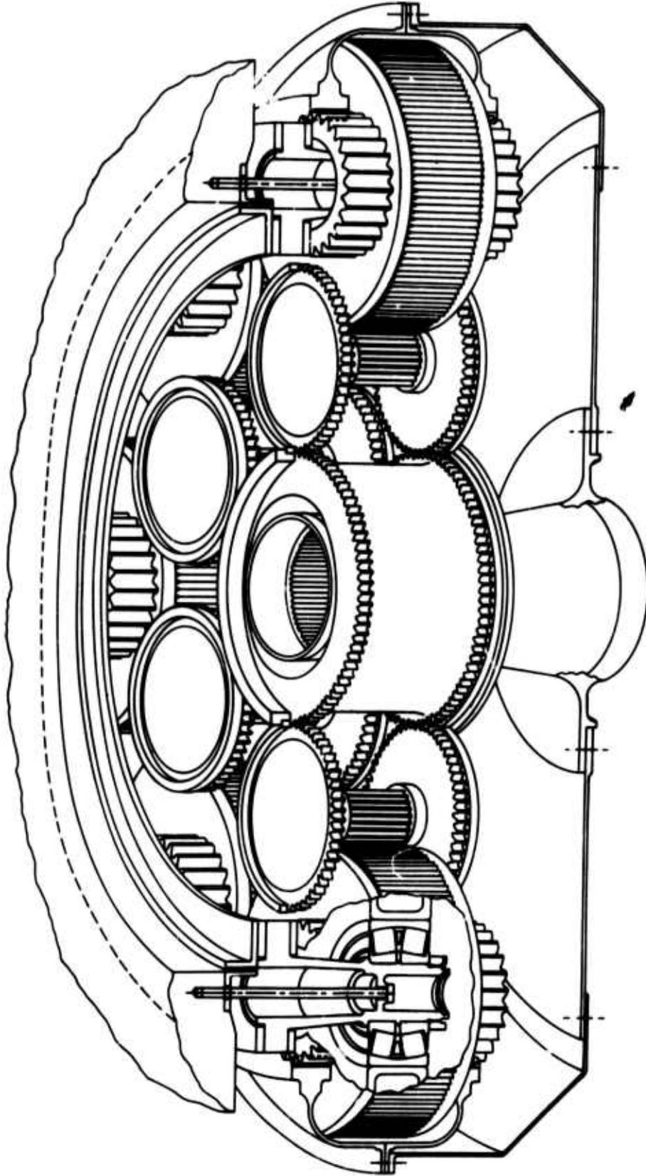
Figure 1. Sikorsky Roller Gear Drive.
