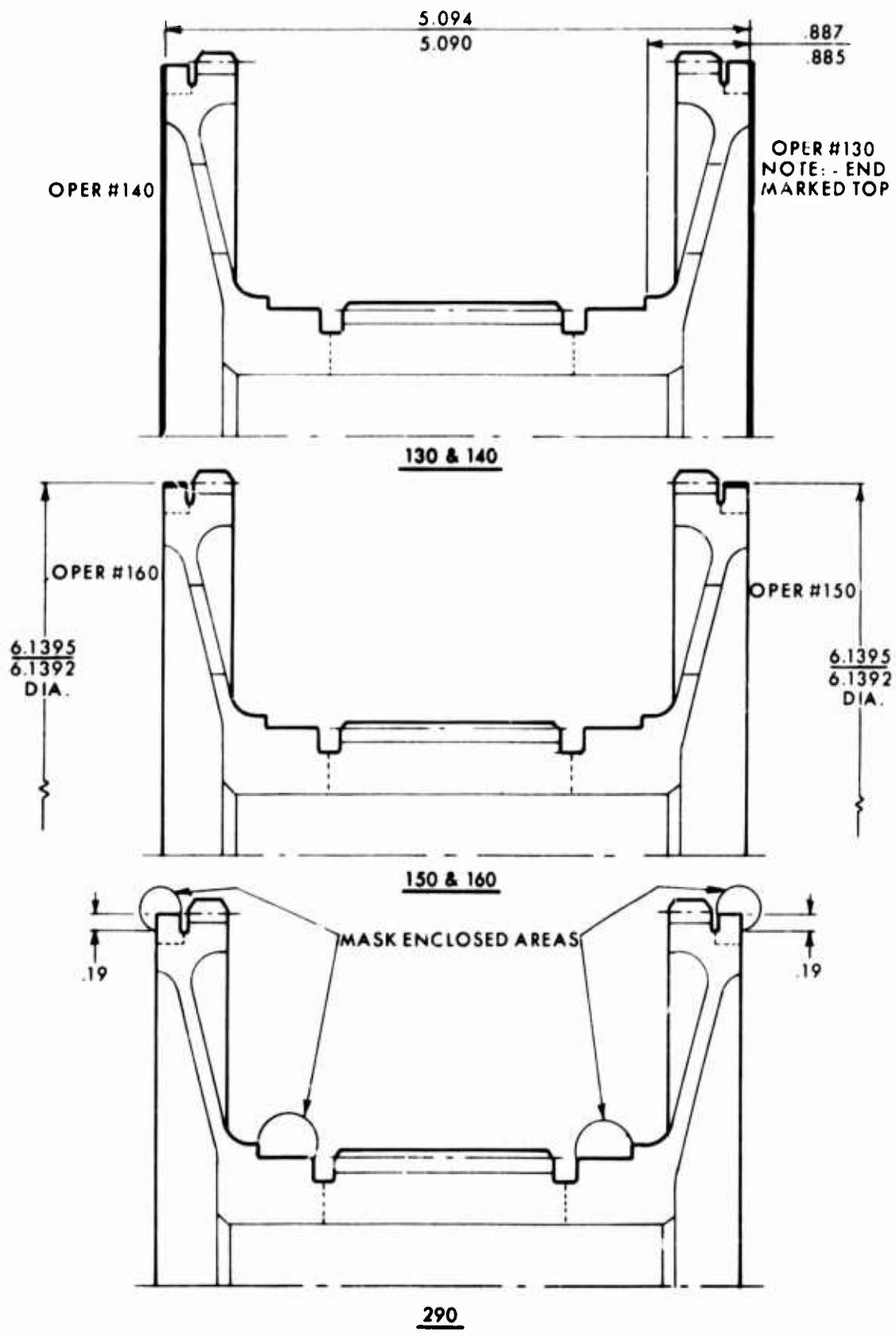
Figure E-6. RG351-11182-061, Machine Operation Drawing.
