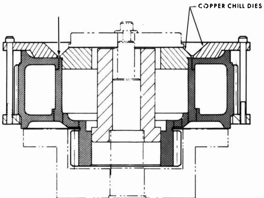
Figure 49. Welding Fixture for Second-Row Pinion Large Gear to Shaft Upper Weld.
