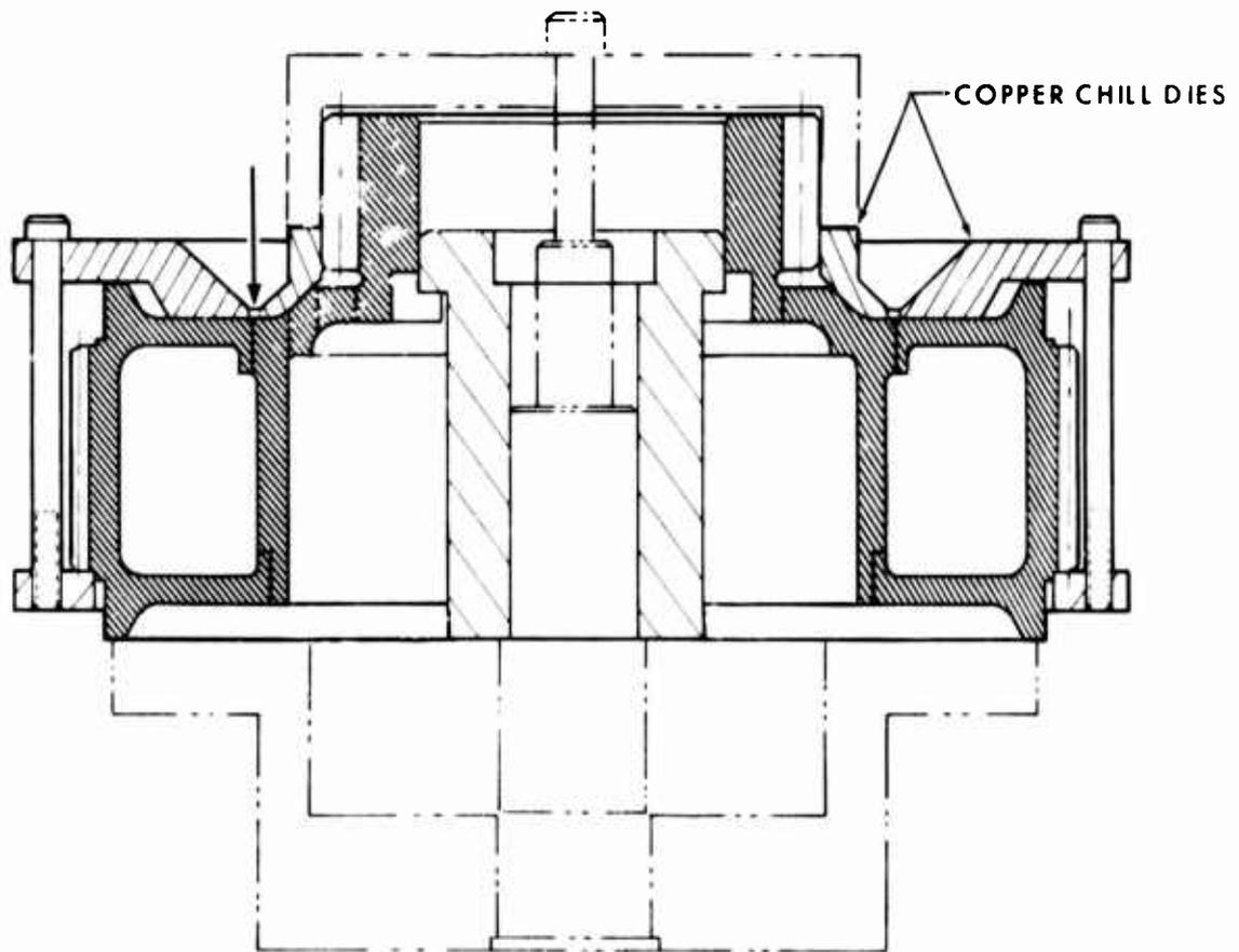
Figure 48. Welding Fixture for Second-Row Pinion
