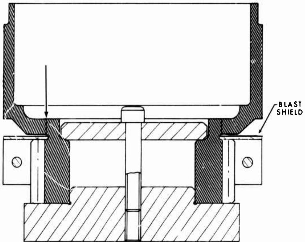
Figure 47. Welding Fixture for Second-Row Pinion Small Gear to Shaft Weld.
