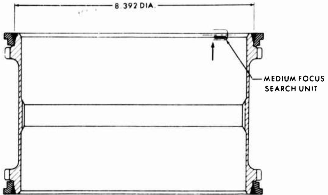
Figure A-3. Ultrasonic Inspection, Sun Gear.
