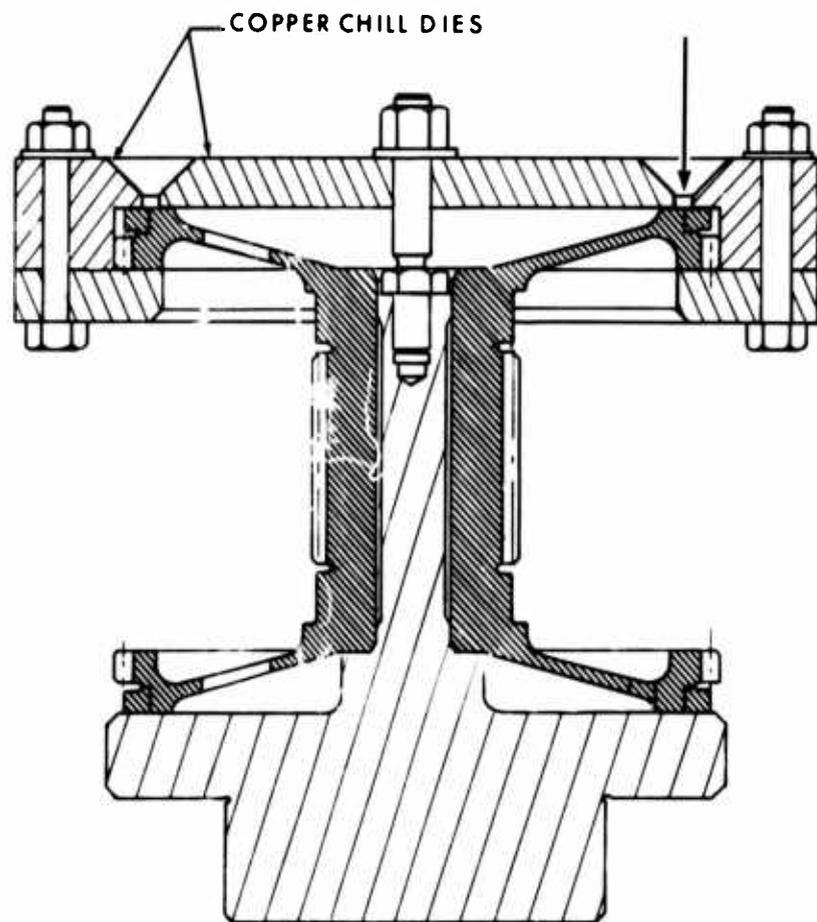
Figure 46. Welding Fixture for First-Row Pinion Roller Weld.
