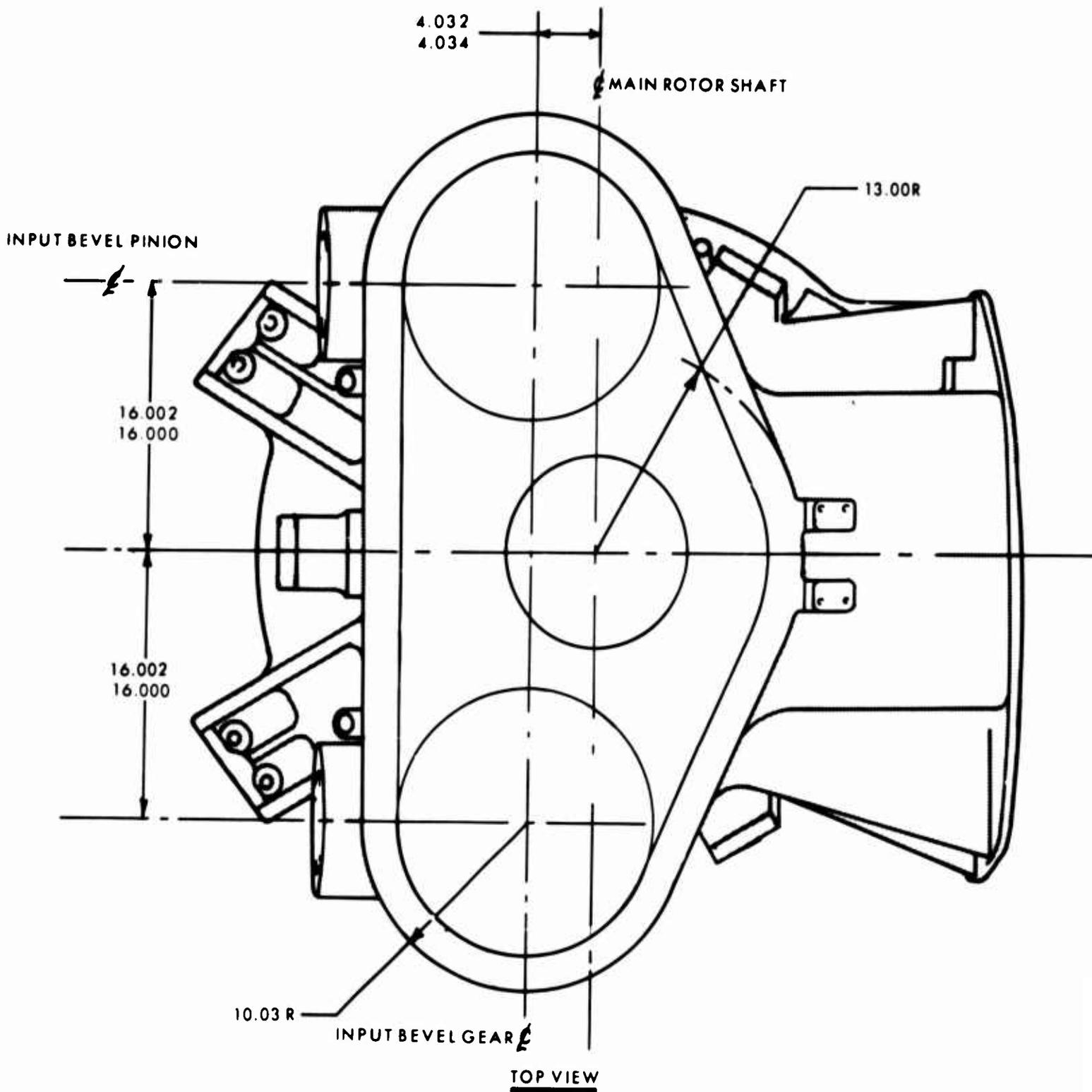
Figure 94. Main Housing, Critical Dimensions.
