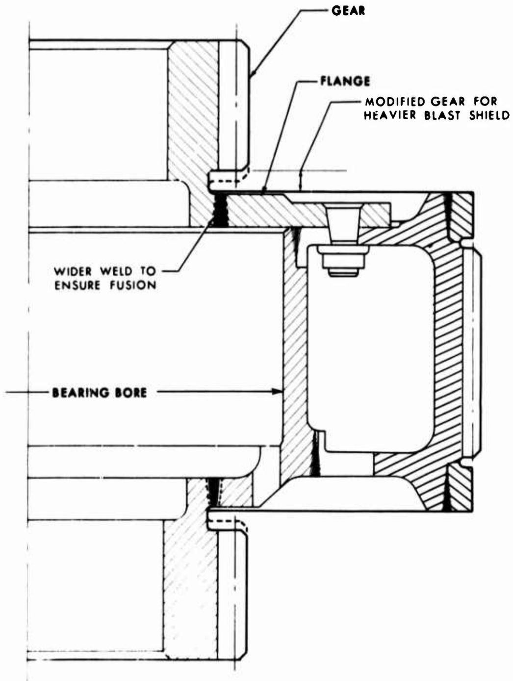
Figure 65. Second-Row Pinion Modification.
