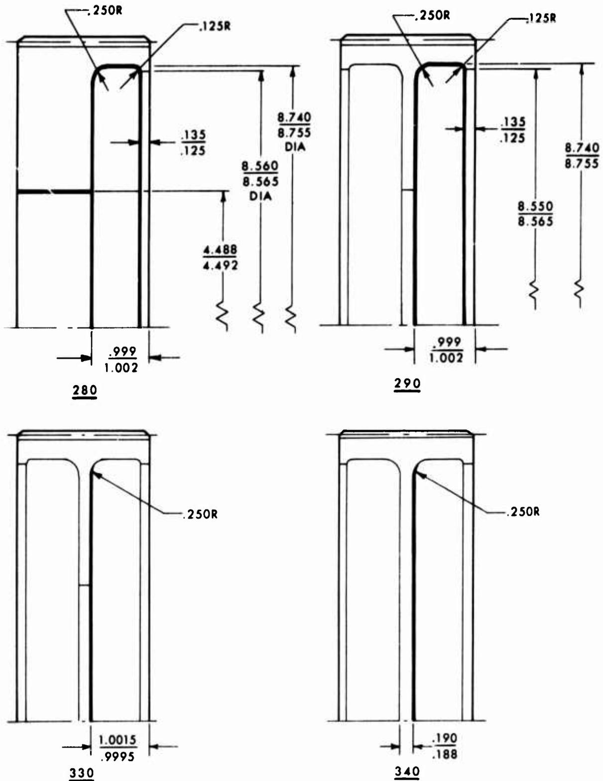
Figure D-5, RG351-11278-103: Machine Operation Drawing (Sheet 2 of 2).
