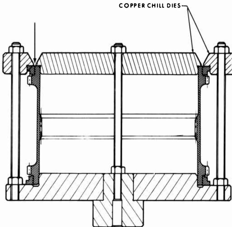
Figure 44. Welding Fixture for Sun Gear Roller Welds.
