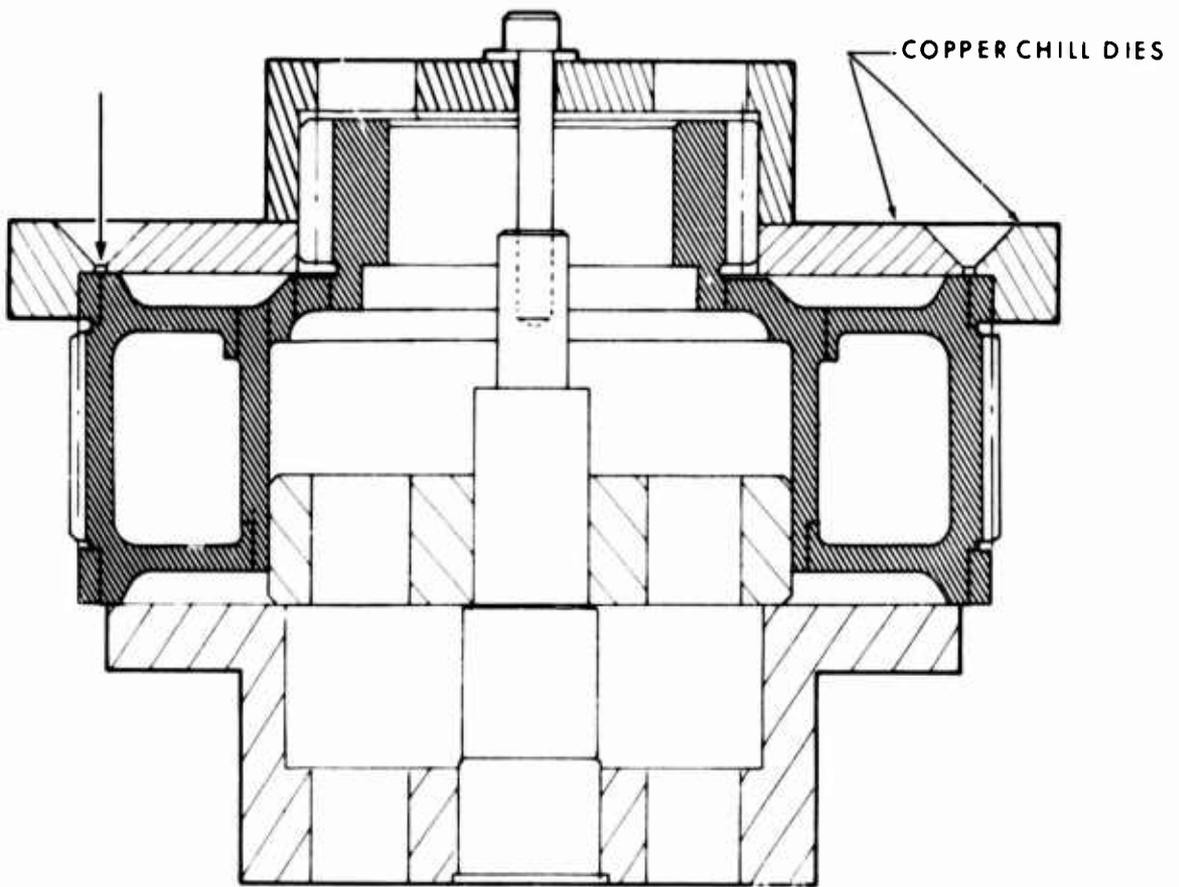
Figure 50. Welding Fixture for Second-Row Pinion Lower Roller Weld.
