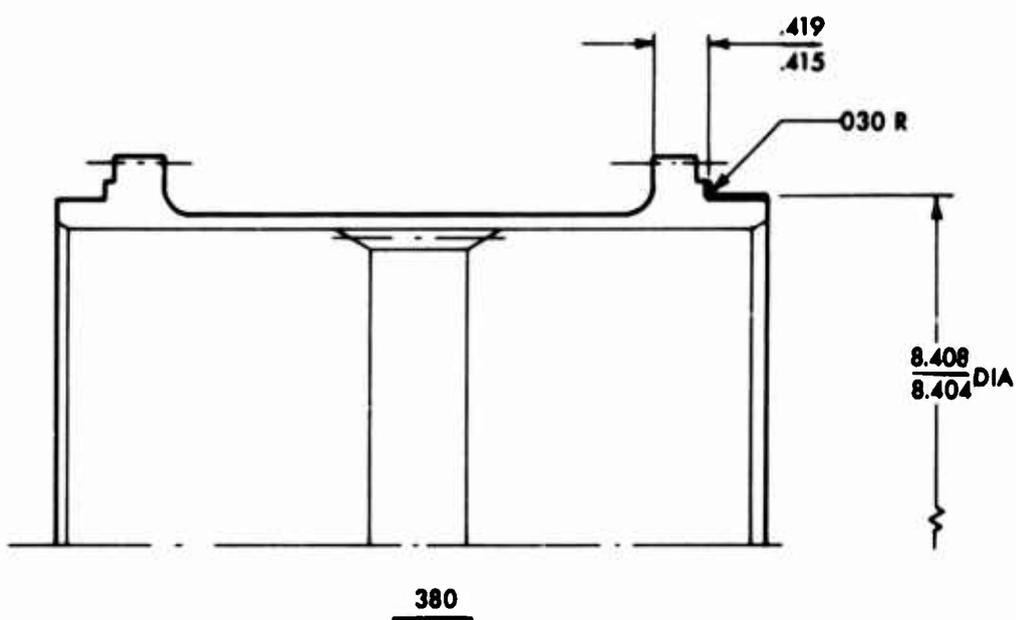
Figure F-3. RG351-11183-041, Machine Operation Drawing.
