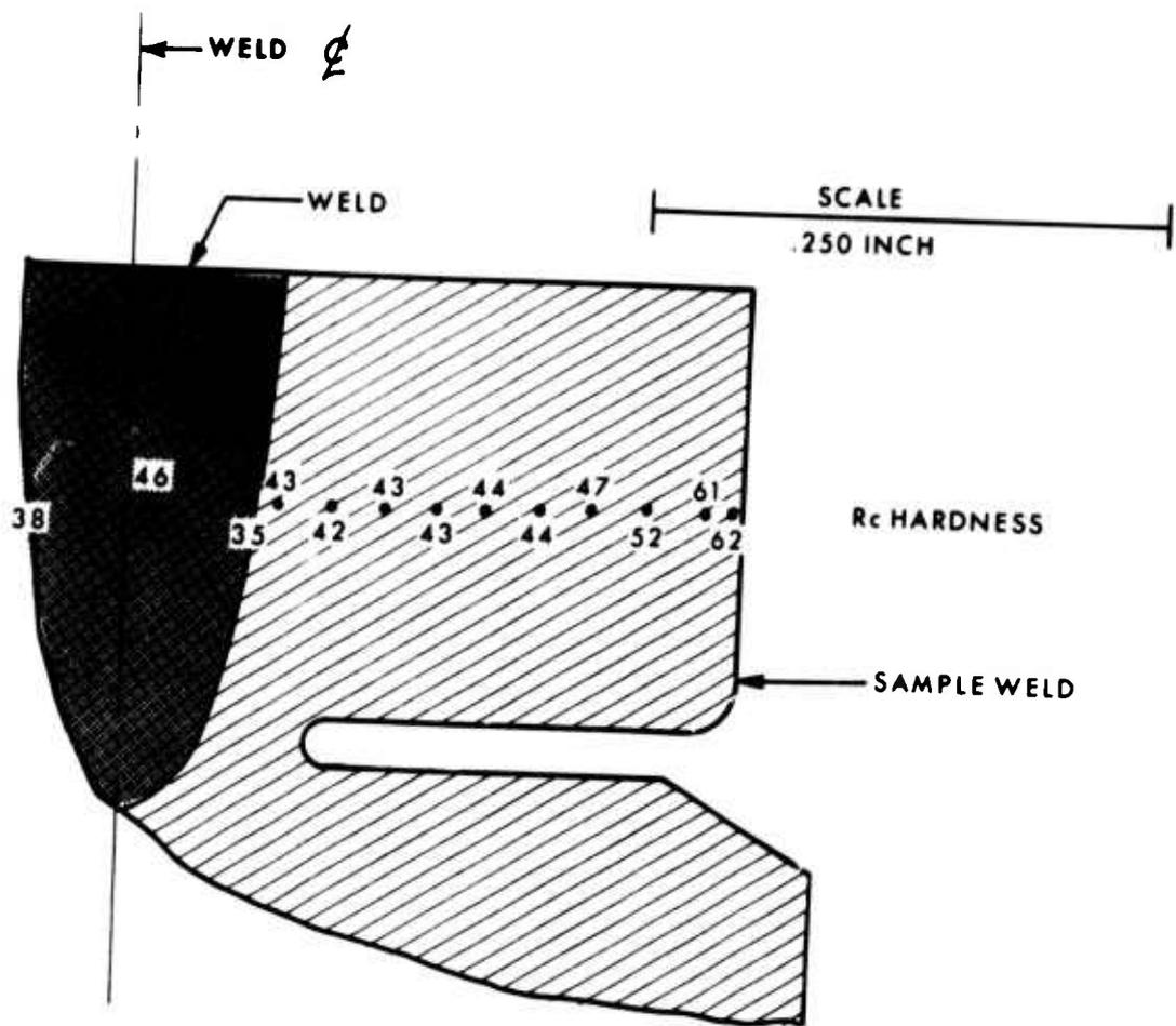
Figure 39. Typical Hardness Test of Electron Beam Weld Showing Effects of Heat on Steel hardness.
