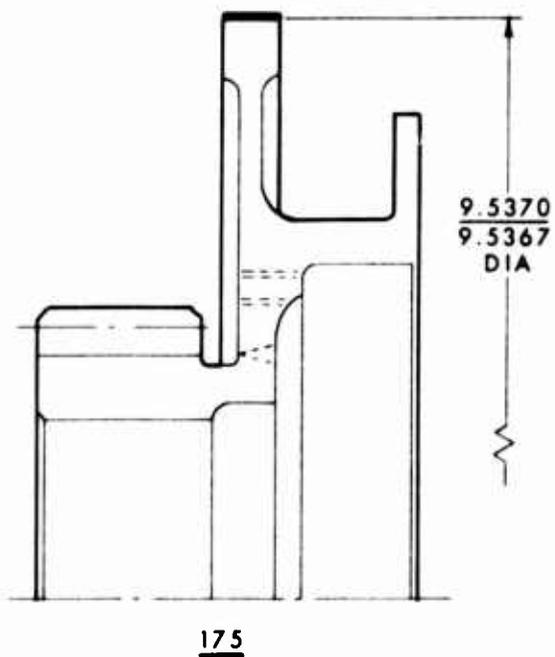
Figure D-7. RG351-11278-045: Machine Operation Drawing (Sheet 2 of 2).
