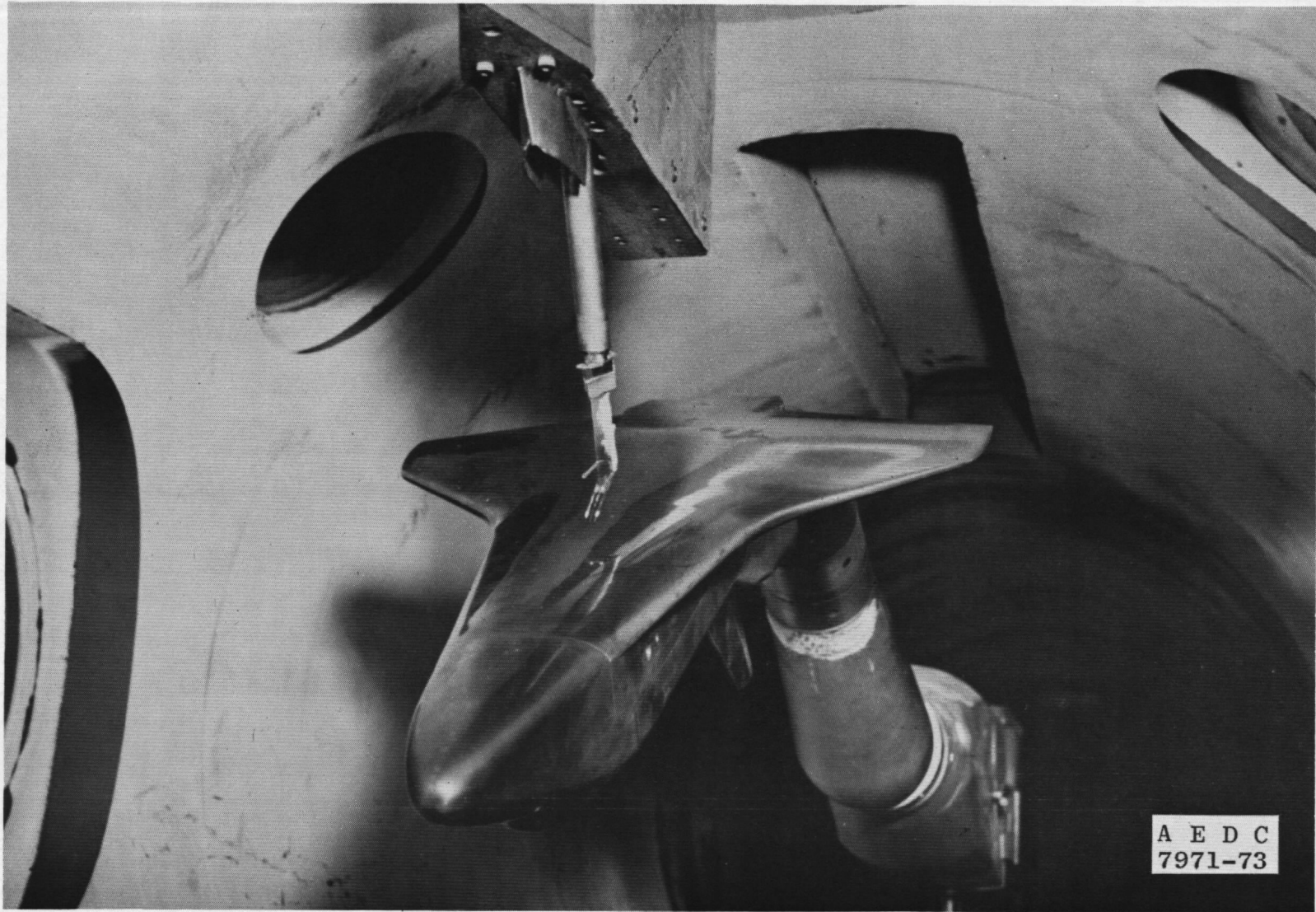
Figure 2. OH9 test installation photograph.
