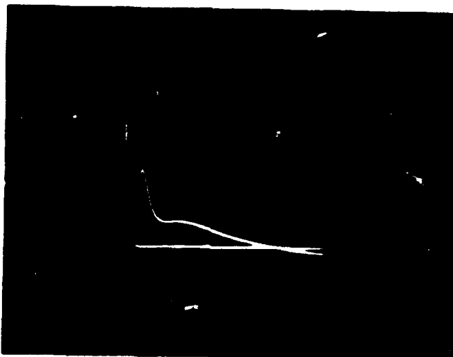
Figure 51. I_{sc} wave form--1 1/2-in. special design flexible conduit ( i = 10 \text{ mA/div} ; t = 0.5 \text{ msec/div} ).
