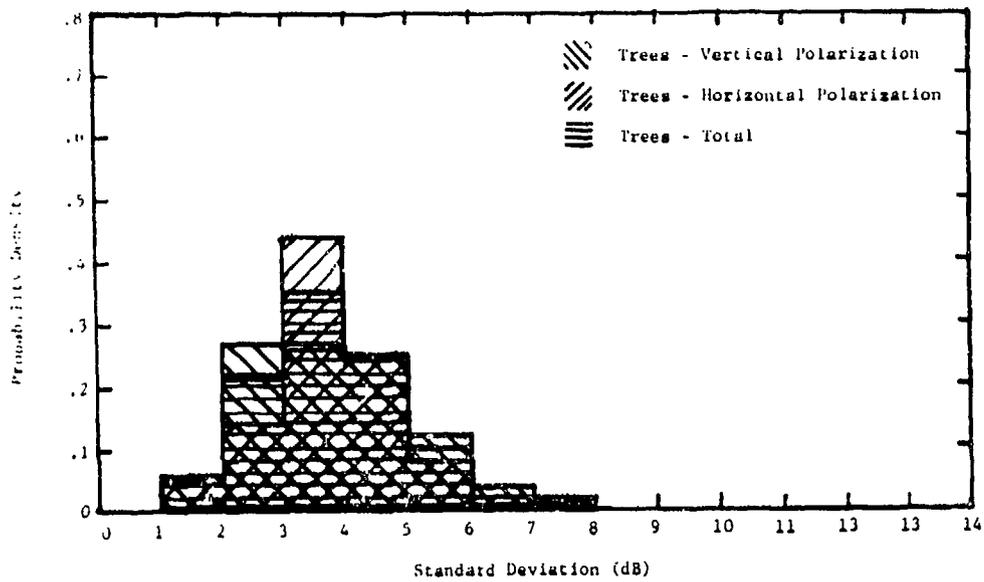
Figure 33. Probability density functions for the measured standard deviations of the amplitude distributions as a function of polarization; 9.5 GHz.
