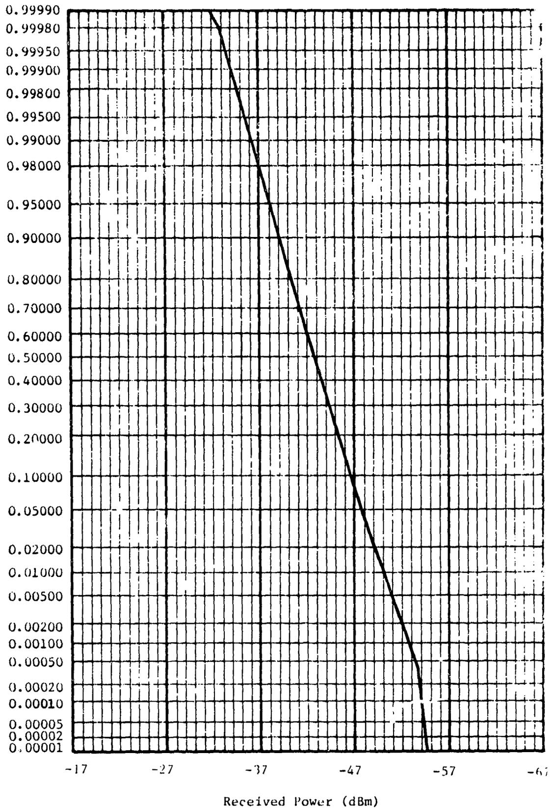
Figure 28. Cumulative probability distribution of the received power from deciduous trees; 95 GHz, horizontal polarization, and  $4.1^\circ$  depression angle.
