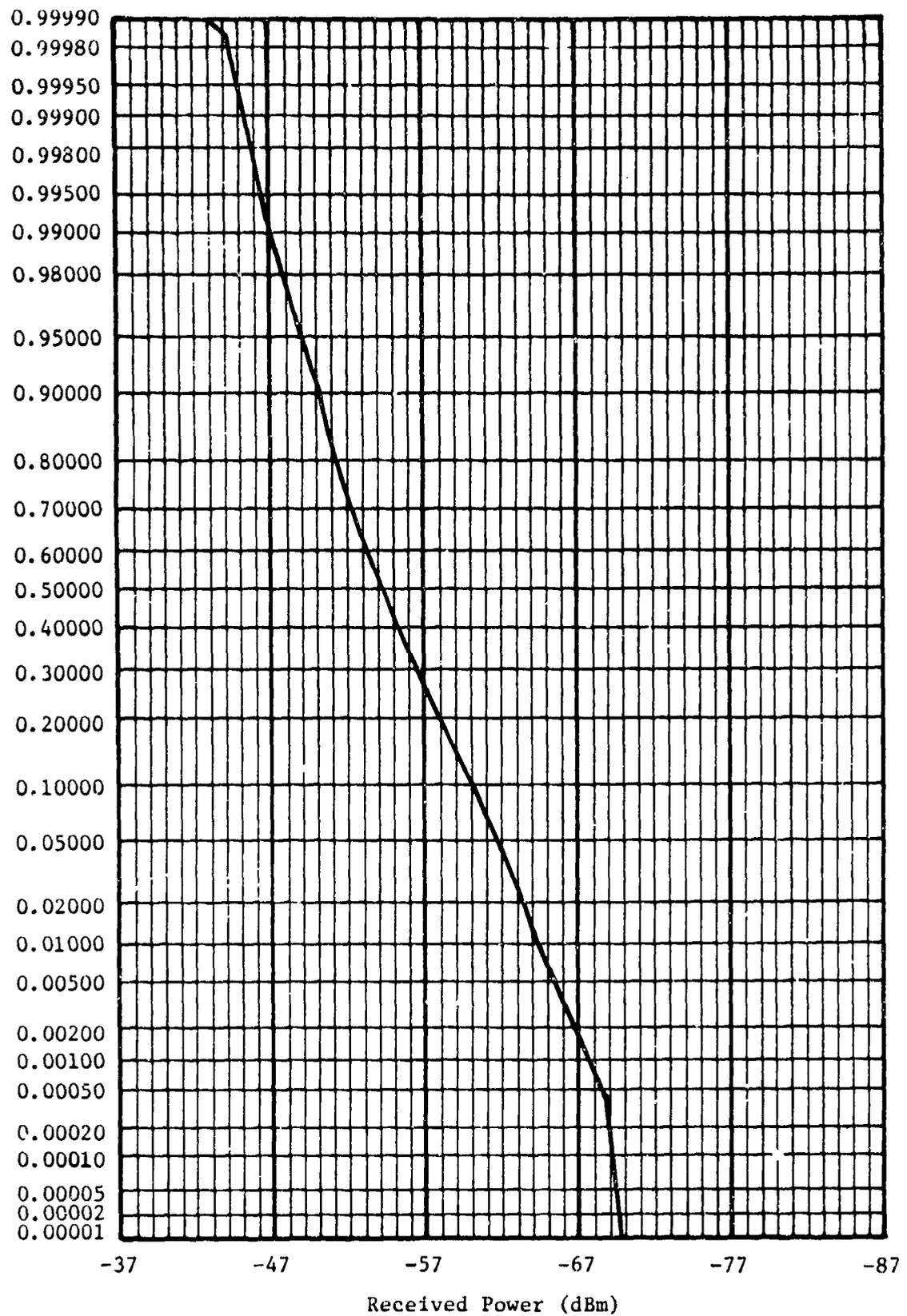
Figure 27. Cumulative probability distribution of the received power from deciduous trees; 35 GHz, horizontal polarization, and  $4.1^\circ$  depression angle.
