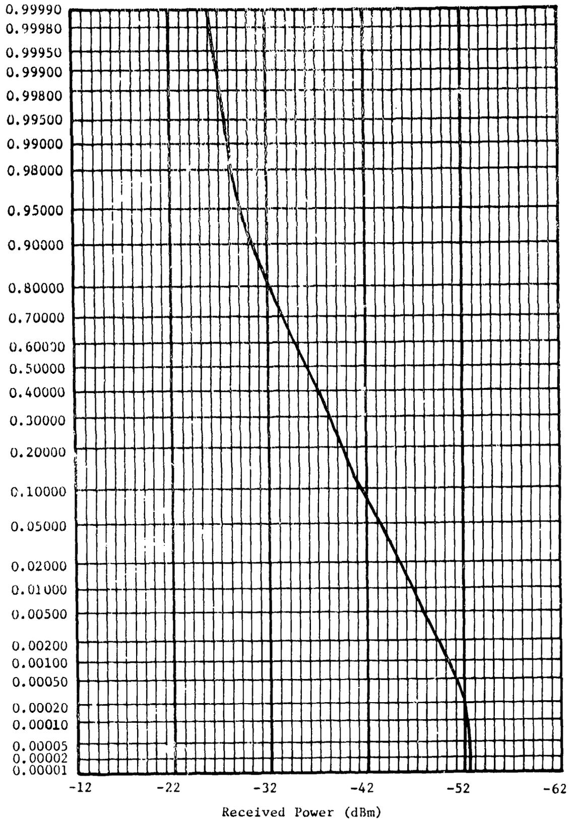
Figure 25. Cumulative probability distribution of the received power from deciduous trees; 9.5 GHz, horizontal polarization, and  $4.1^\circ$  depression angle.
