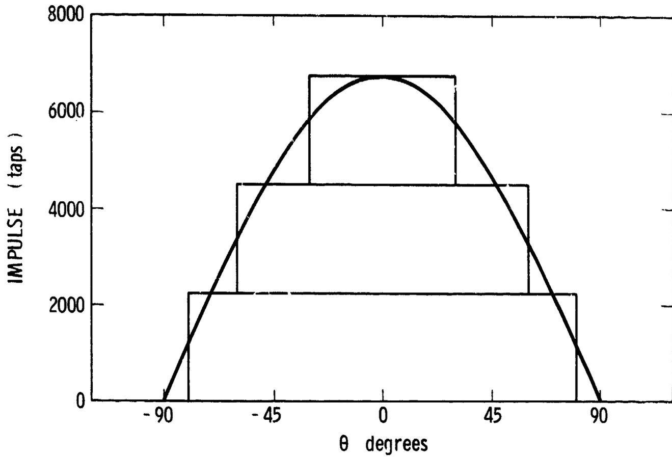
Figure 8. Cosine Load Approximated by Three Layers of Stripped SE. The cross-sectional area of the SE approximately equals the area under the cosine curve.
