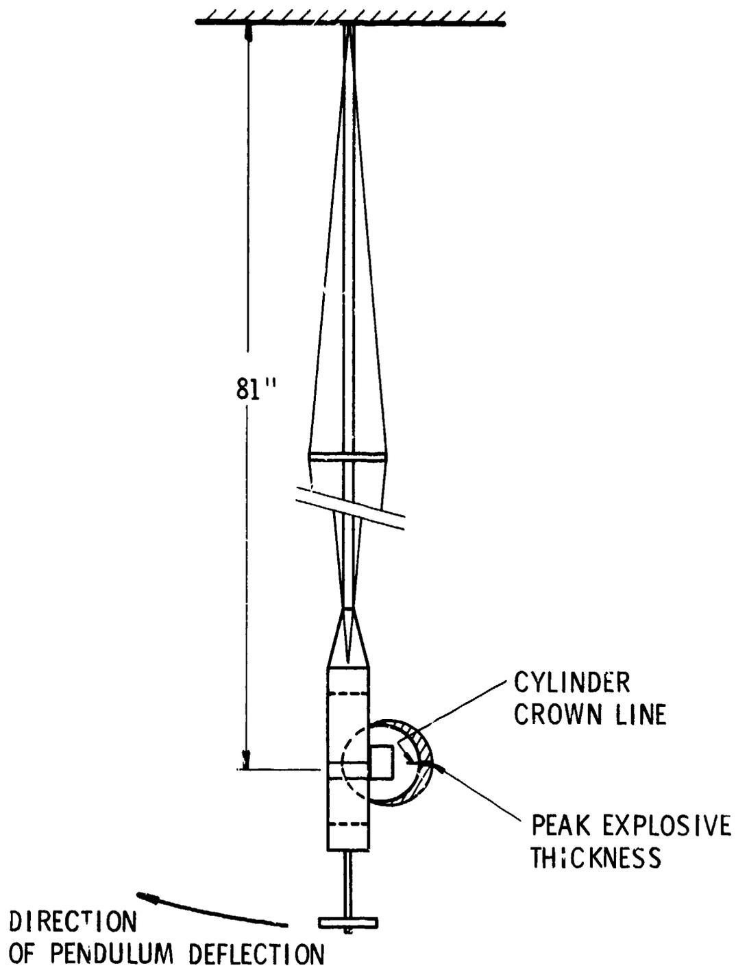
Figure 6. Ballistic Pendulum with Mounted Test Cylinder
