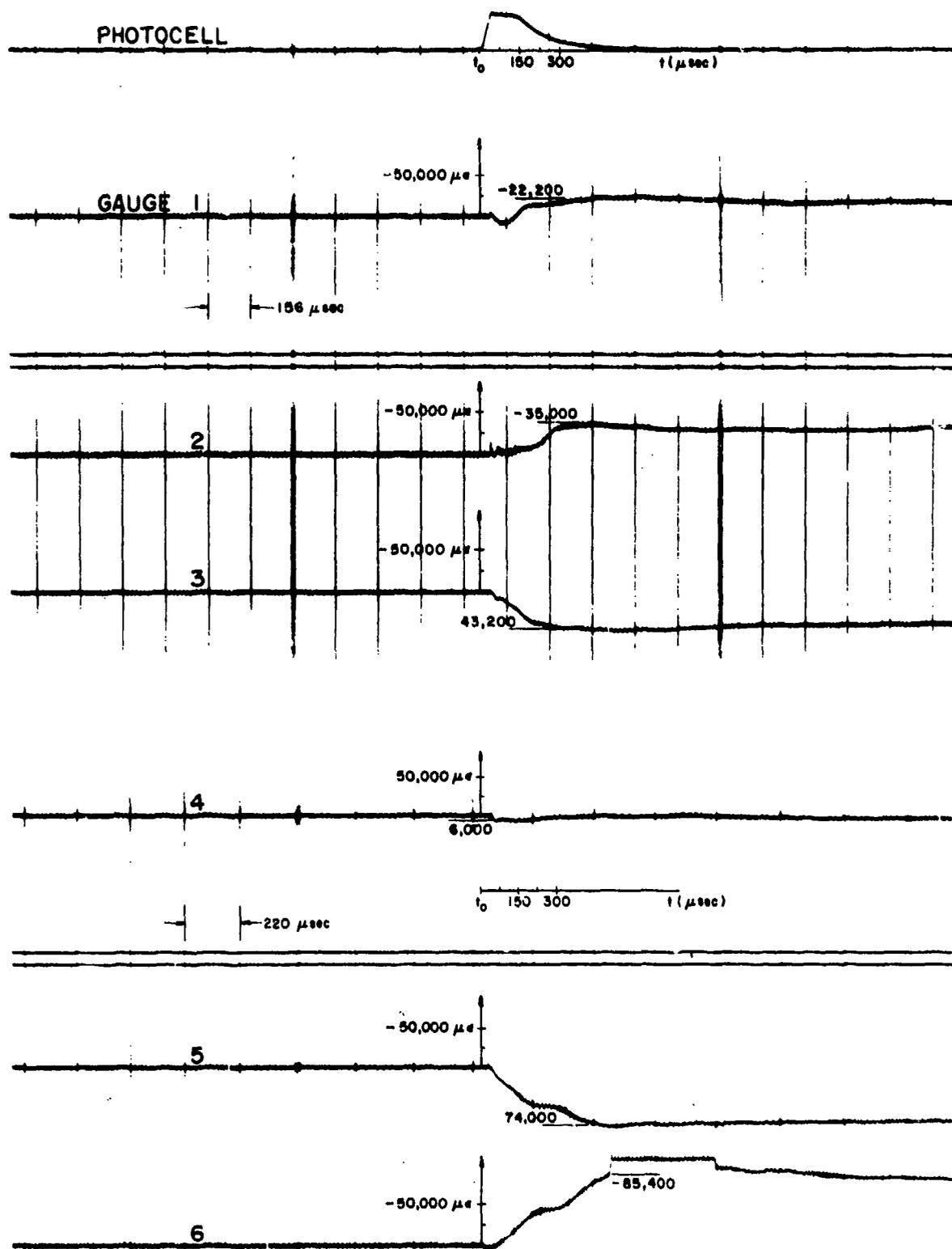
FIGURE B-7. TEST #21 - Pb CYLINDER, SE CIRCUMFERENTIAL RUNNING LOAD, PEAK SPECIFIC IMPULSE 4.5 KILOTAPS
