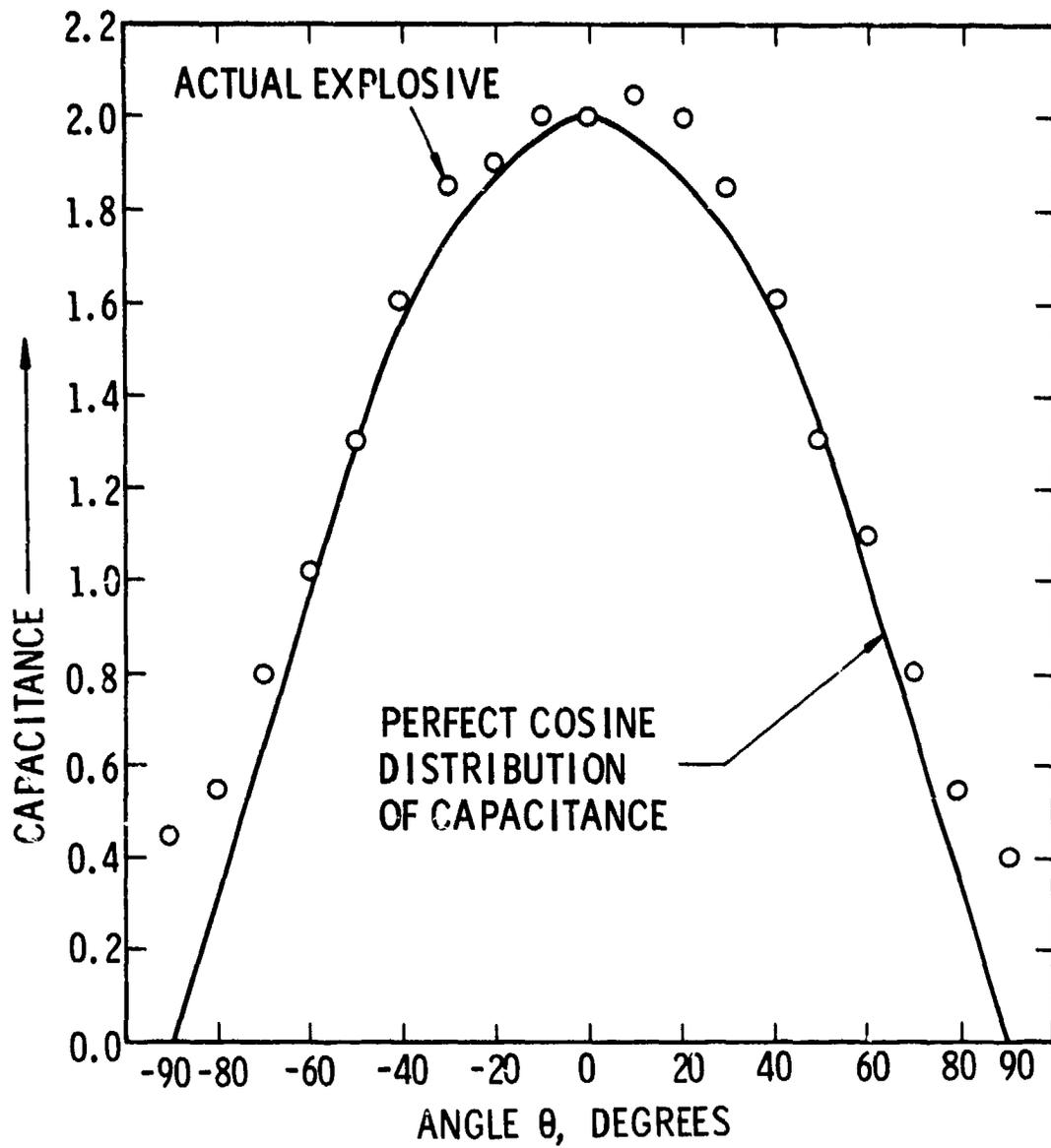
Figure 5. Cosine Distribution of SASN Explosive Used for Test #25
