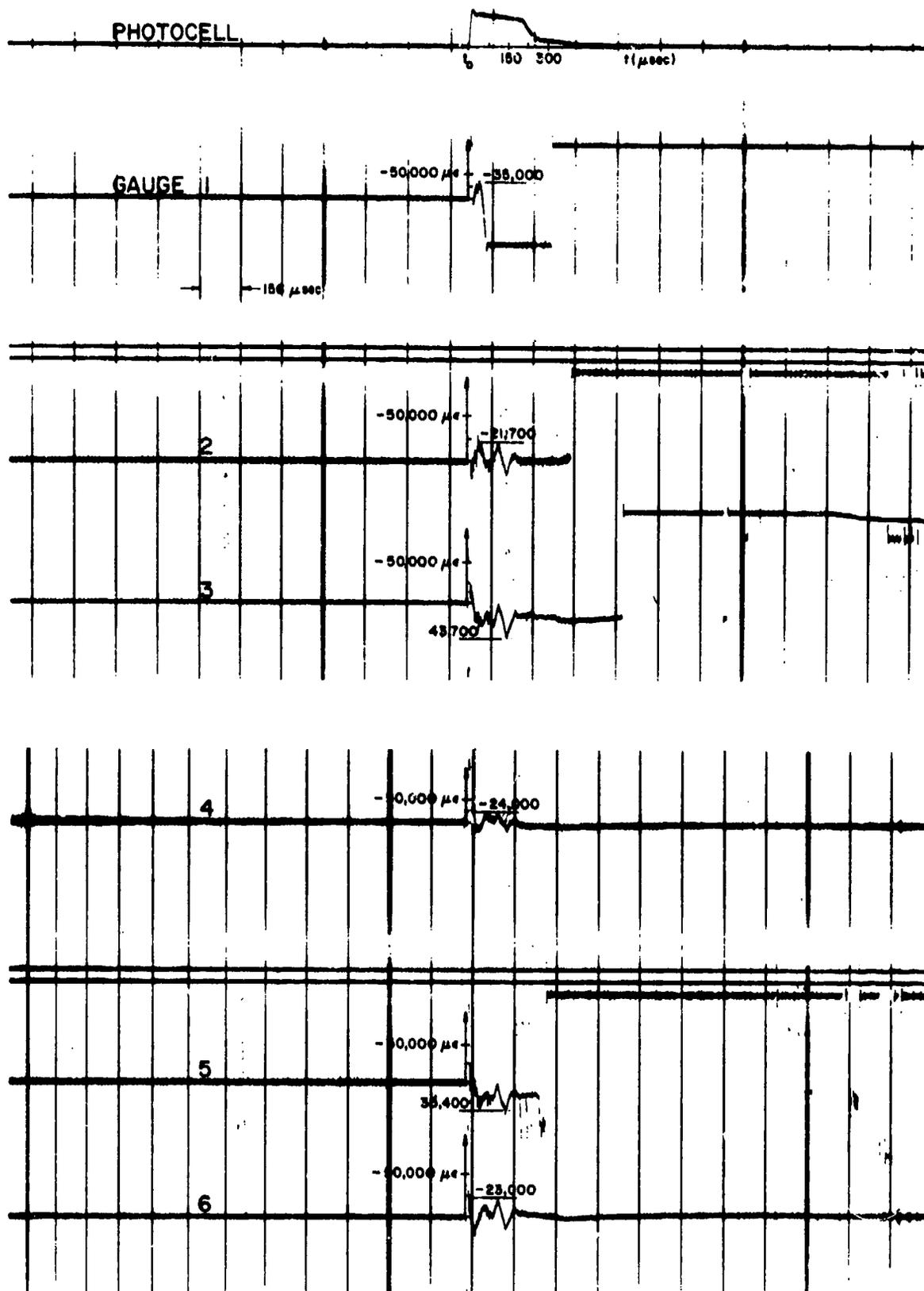
FIGURE B-15. TEST #27 - Al CYLINDER, SASN SIMULTANEOUS LOAD. PEAK SPECIFIC IMPULSE 4.44 KILOTAPS
