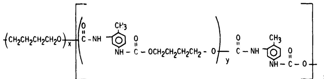
Figure 1. Idealized structure of PTMO/2,4-TDI/BD polyurethane block copolymer.
