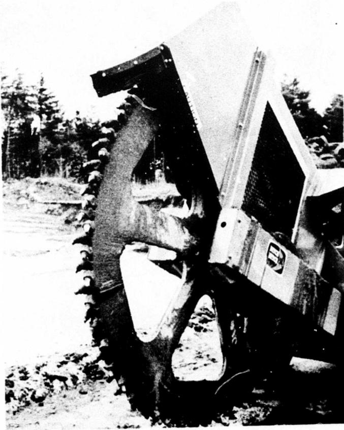
Figure 5. Cutter wheel of Ditch Witch ES30.
