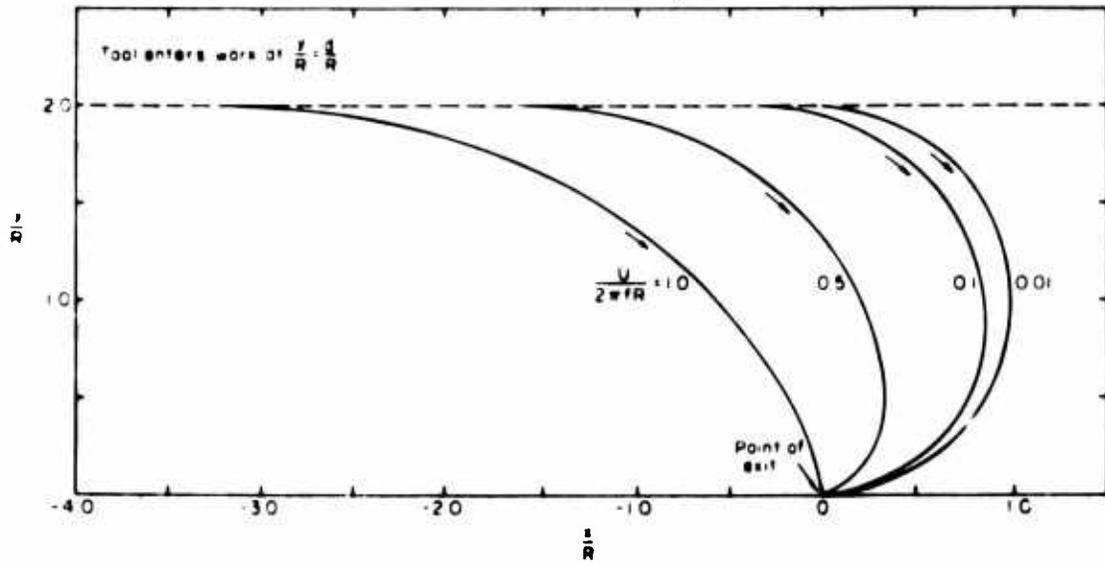
Figure 5. Tooth-tip trajectories for upmilling and climb milling rotors.
