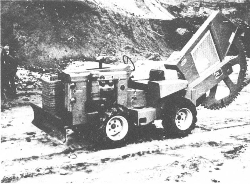
Figure 2. Ditch Witch ES30 Earth Saw on R60 Trencher.
