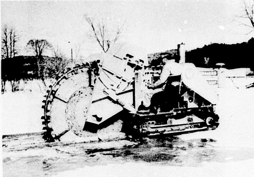
*Figure 10. Vermeer T-600B cutting floating ice. The machine was able to cut 18-in.-thick ice at maximum crawl speed (26 ft/min) with no perceptible effort. A contractor recently made long cuts in lake ice with a Ditch Witch saw, averaging 6.7 ft/min.*
