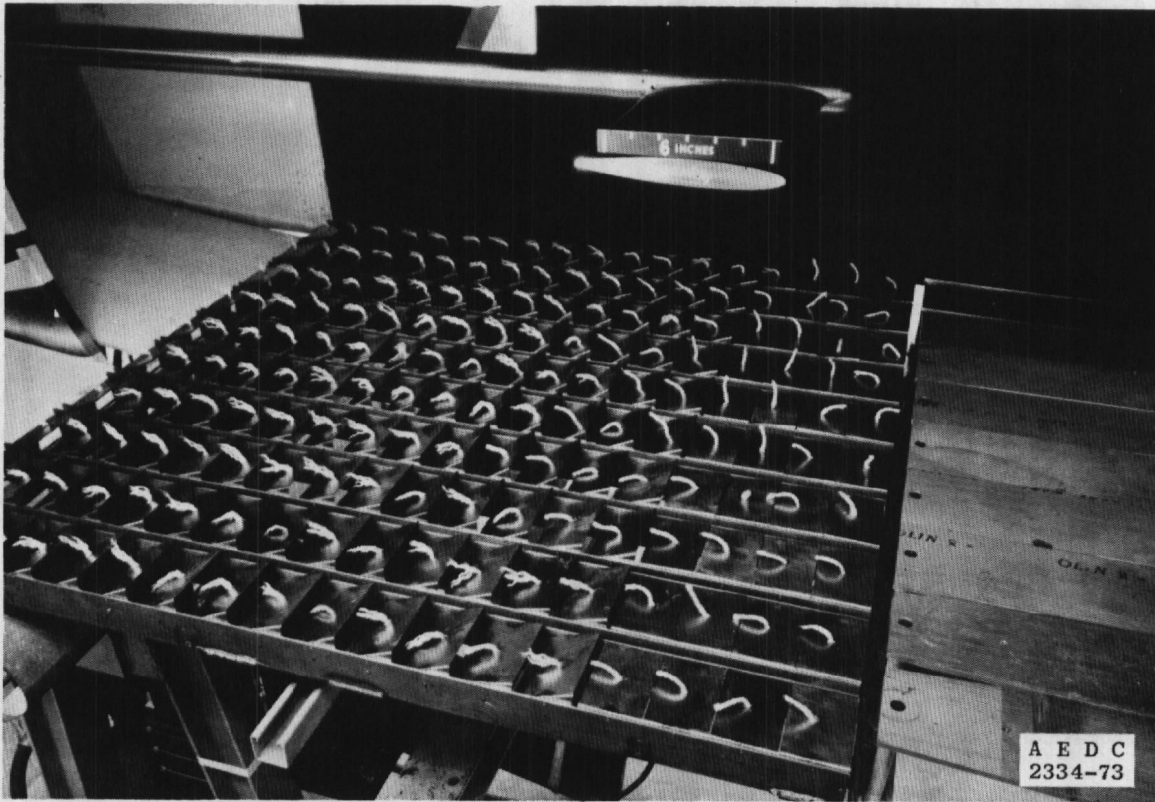
Figure 4. Louvered bottom test section wall.
