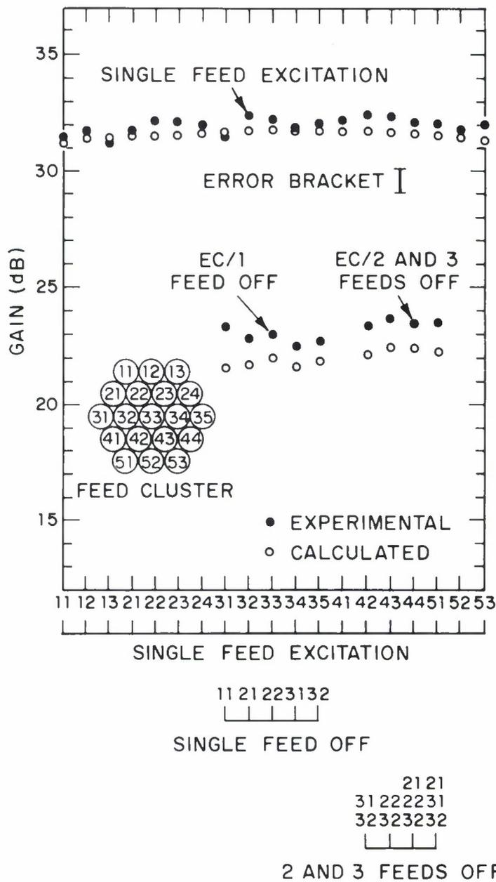
Fig. 14. Gain comparison for 30-inch diameter lens using variable power divider (VPD) feed network at  $f = 7.68$  GHz.
