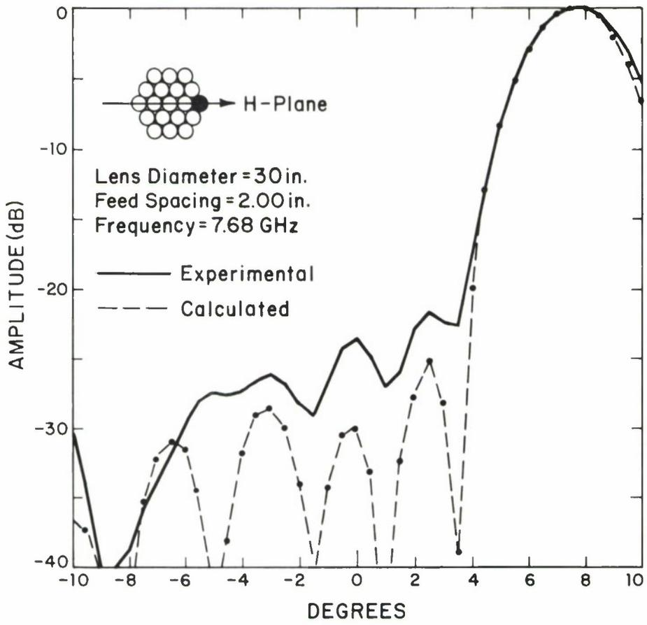
Fig. 3. Comparison of measured and calculated H-plane patterns, single feed on.
