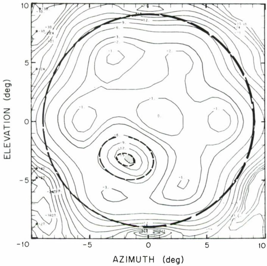
Fig. 12. Measured earth-coverage contour with feed 22 off.
