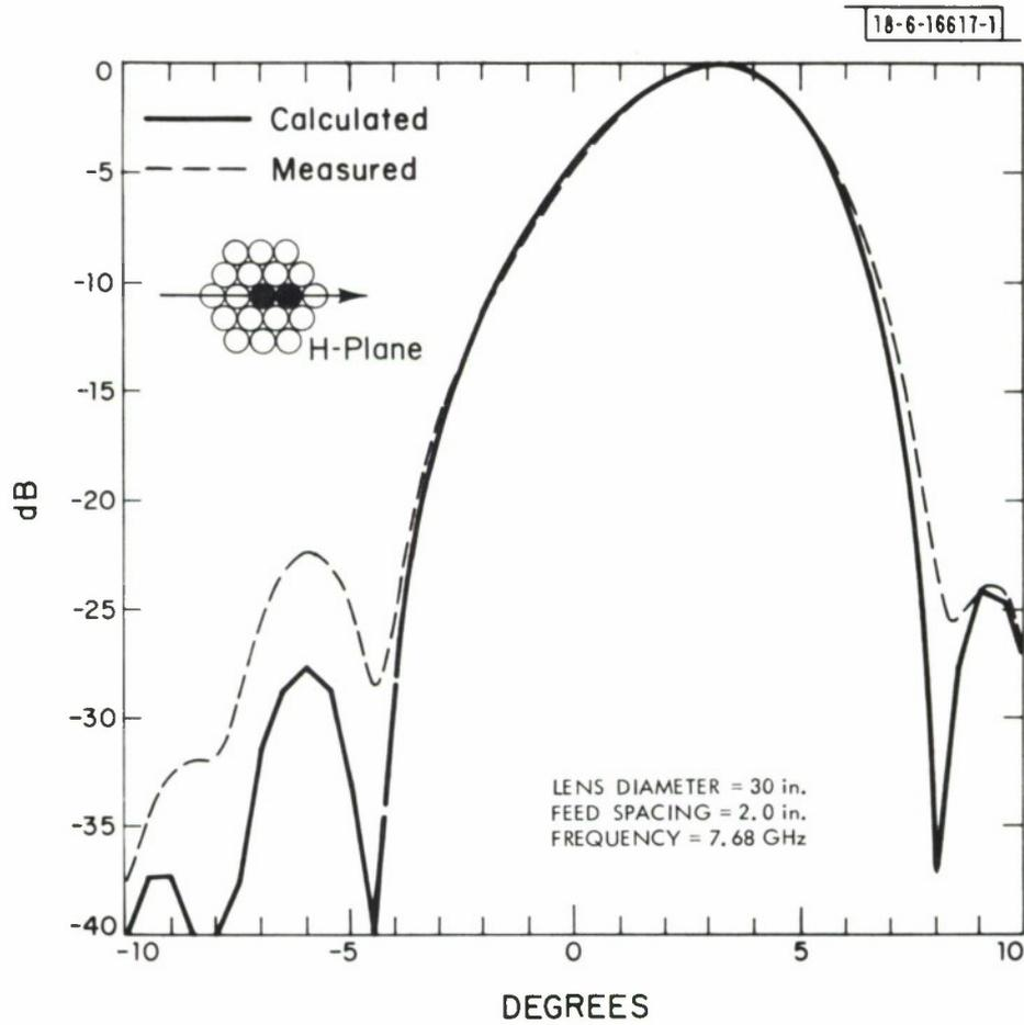
Fig. 8. Beam scanning characteristics for  $P_{33} = 0.25$ ,  $P_{34} = 0.75$ .
