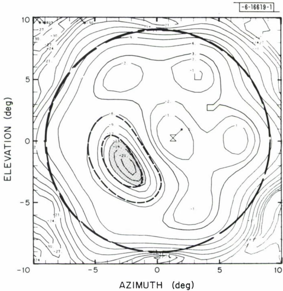
Fig. 13. Measured earth-coverage contour with feeds 22 and 32 off.
