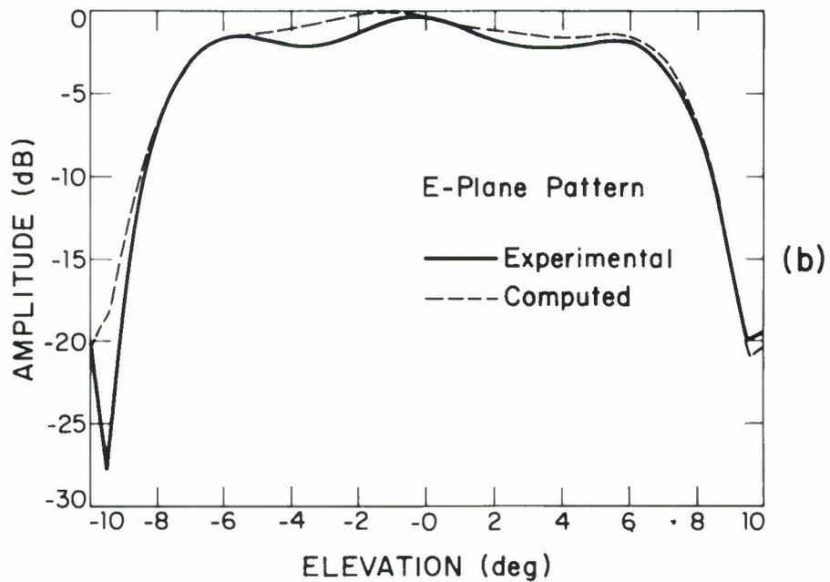
Fig. 11. Comparison of measured and computed earth-coverage patterns.
