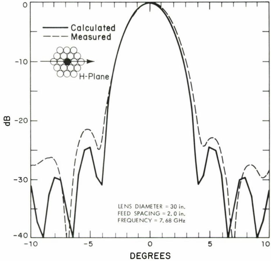
Fig. 5. Beam scanning characteristics for  $P_{33} = 1.0$ ,  $P_{34} = 0$ .
