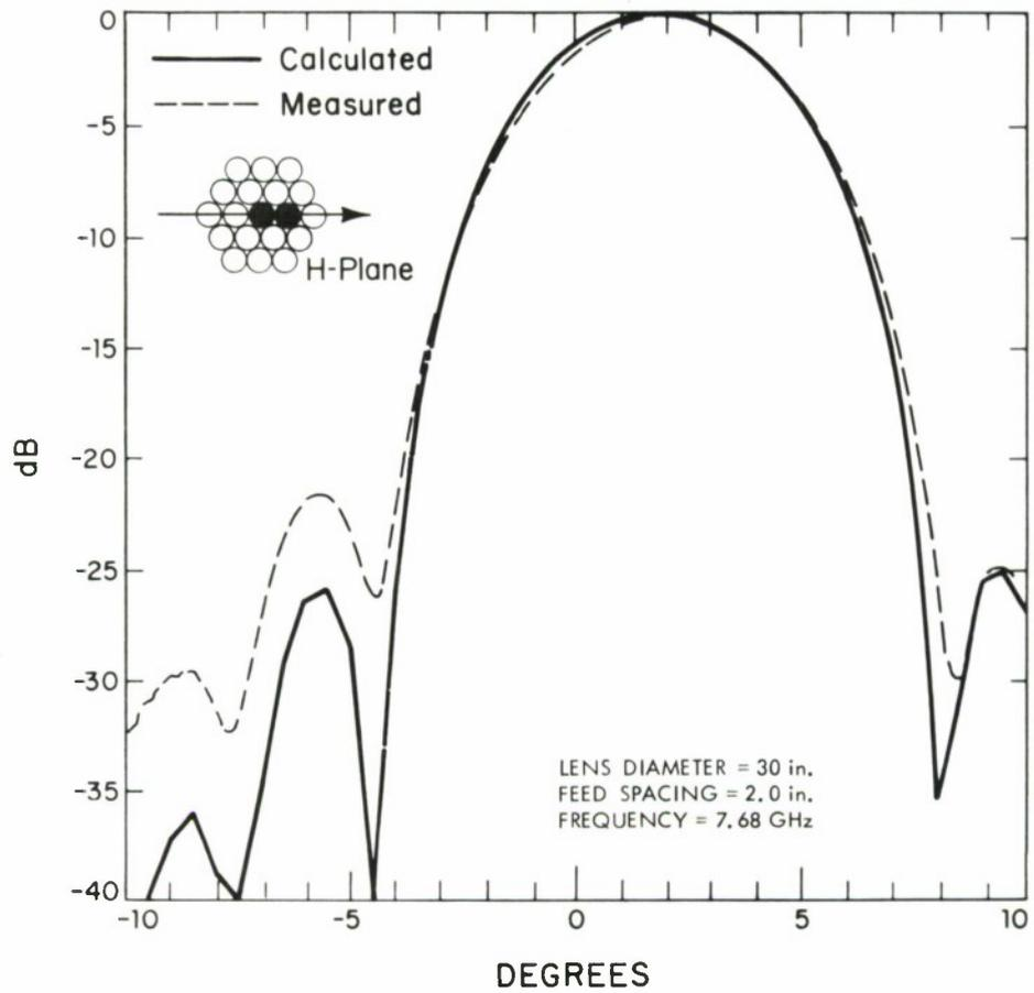
Fig. 7. Beam scanning characteristics for  $P_{33} = 0.50$ ,  $P_{34} = 0.50$ .
