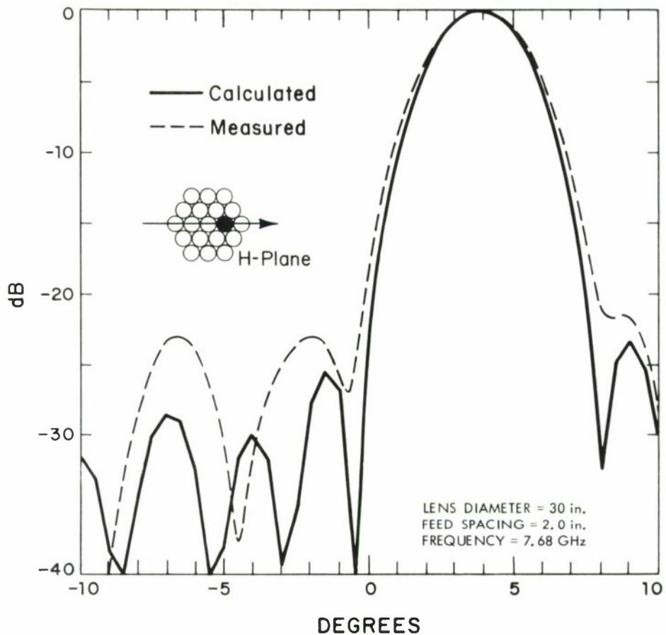
Fig. 9. Beam scanning characteristics for  $P_{33} = 0$ ,  $P_{34} = 1.0$ .
