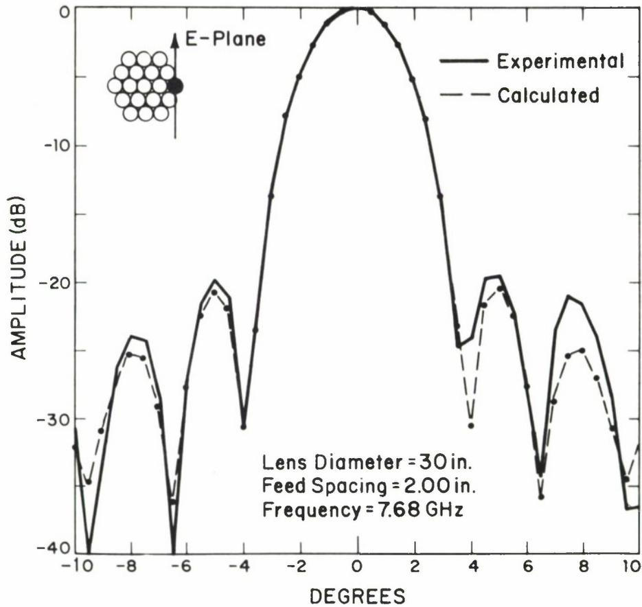
Fig. 4. Comparison of measured and calculated E-plane patterns, single feed on.
