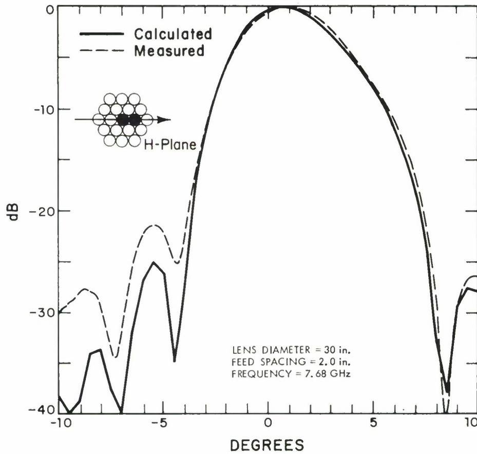
Fig. 6. Beam scanning characteristics for  $P_{33} = 0.75$ ,  $P_{34} = 0.25$ .
