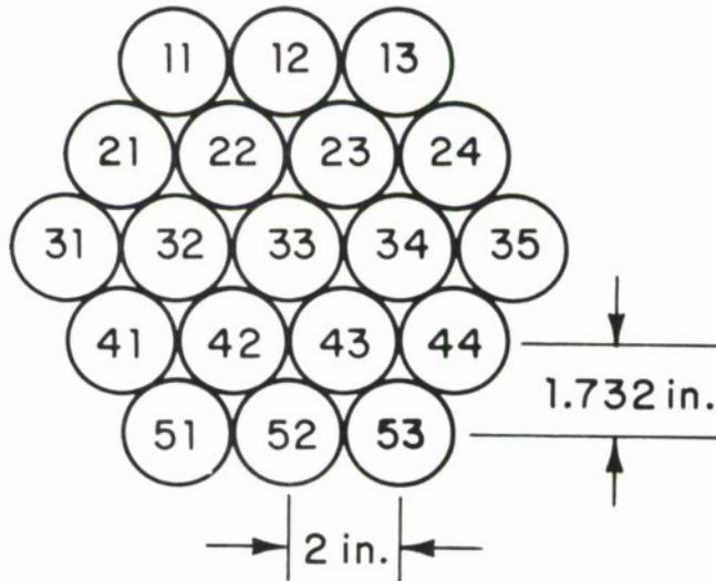
Fig. 2. Feed cluster geometry, indicating numbering scheme.
