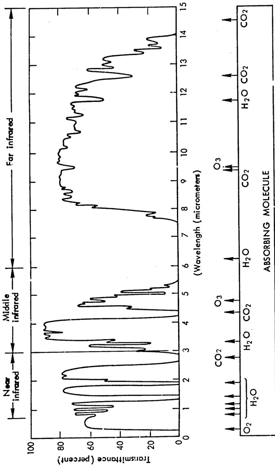
Fig. 1—Transmittance of the atmosphere for a 6000 ft horizontal path at sea level containing 17 mm of precipitable water
