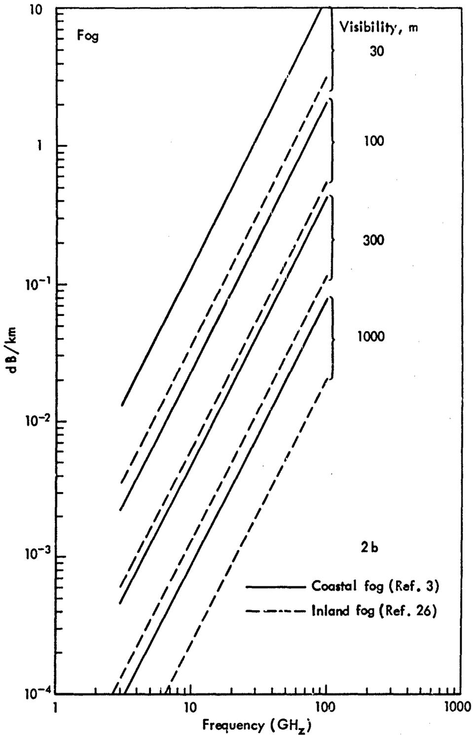
Fig. 12— Calculated attenuation by fog at 18° C
