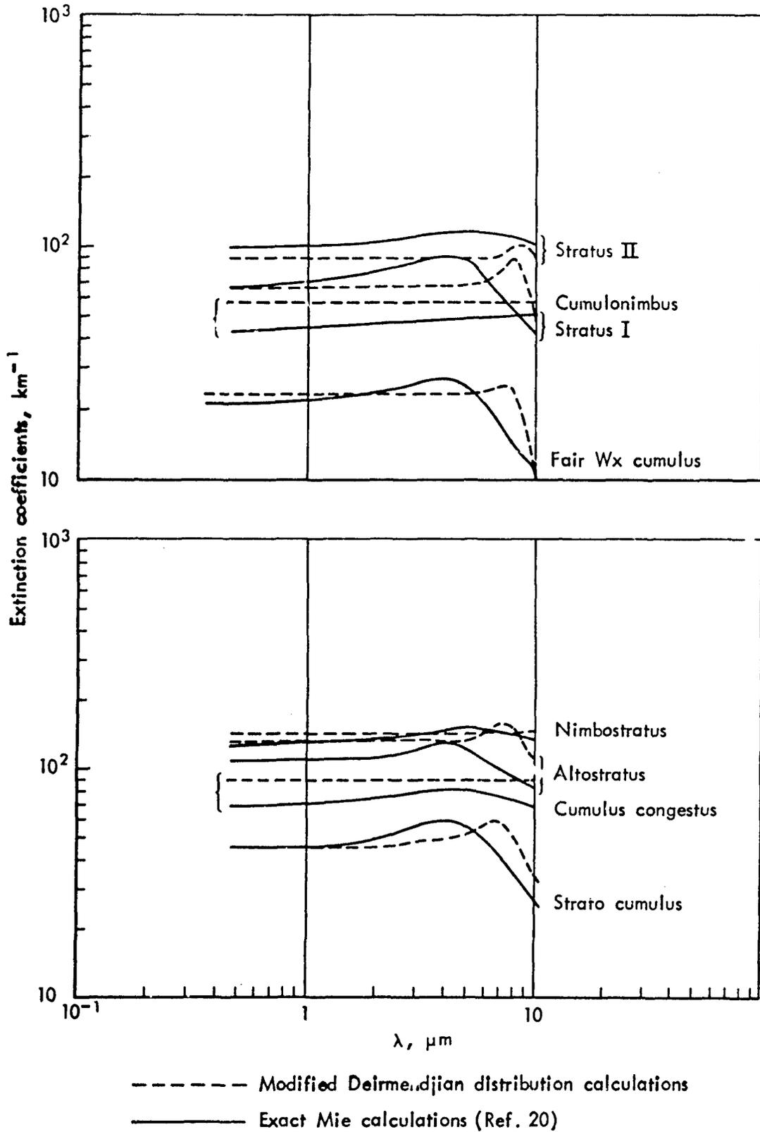
Fig. 6— Calculated visible/IR extinction coefficient due to clouds
