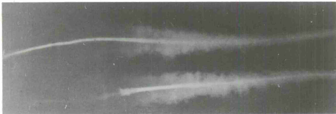
Figure 3.11 Trailing pair undergoing both vortex breakdown and Crow instability [56]
