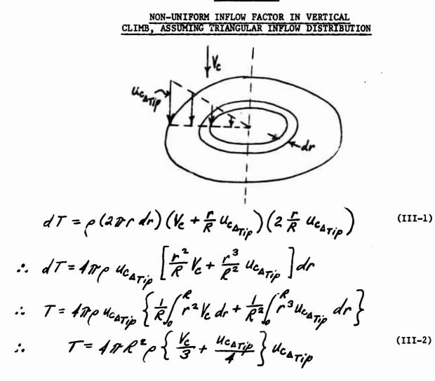
$u_{c_{A_{Tip}}}^{2} + \frac{4}{3} V_{c} u_{c_{A_{Tip}}}^{2} - \frac{1}{\mathcal{P}\mathcal{R}^{2}\rho} = 0$ Then  $\mathcal{U}_{C_{A_{Tip}}} = -\frac{2}{3}V_{C} + V(\frac{2}{3}V_{C})^{2} + \frac{T}{2R^{2}\rho}$ (III-3)  $dP = dT \left( Y_c + \frac{r}{R} u_{c_{A rip}} \right)$ Now
