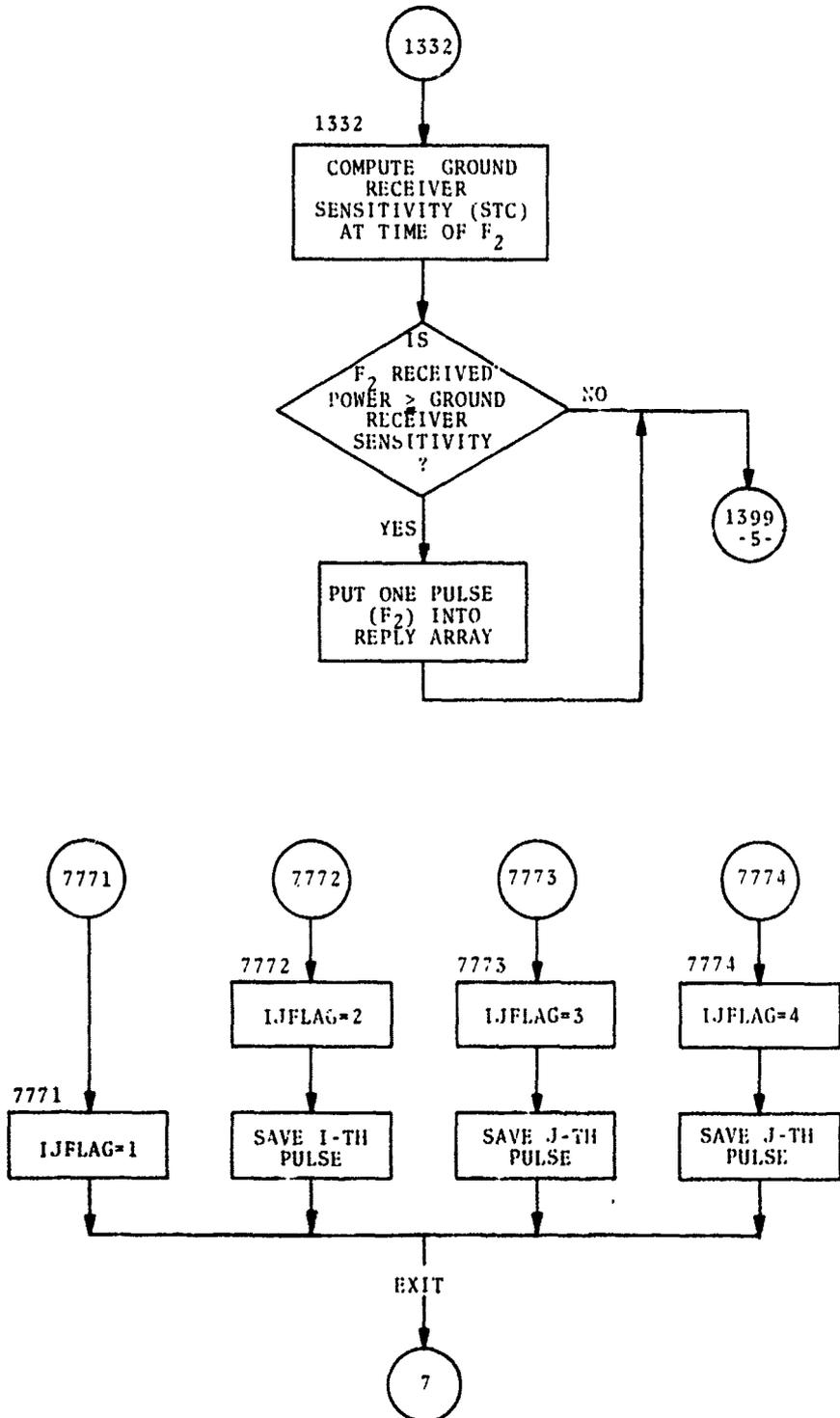
Figure 4-5. Flow Chart of ATCRBS Transponder Program Modifications to Provide DABS Operation Capability (Sheet 6 of 6)
