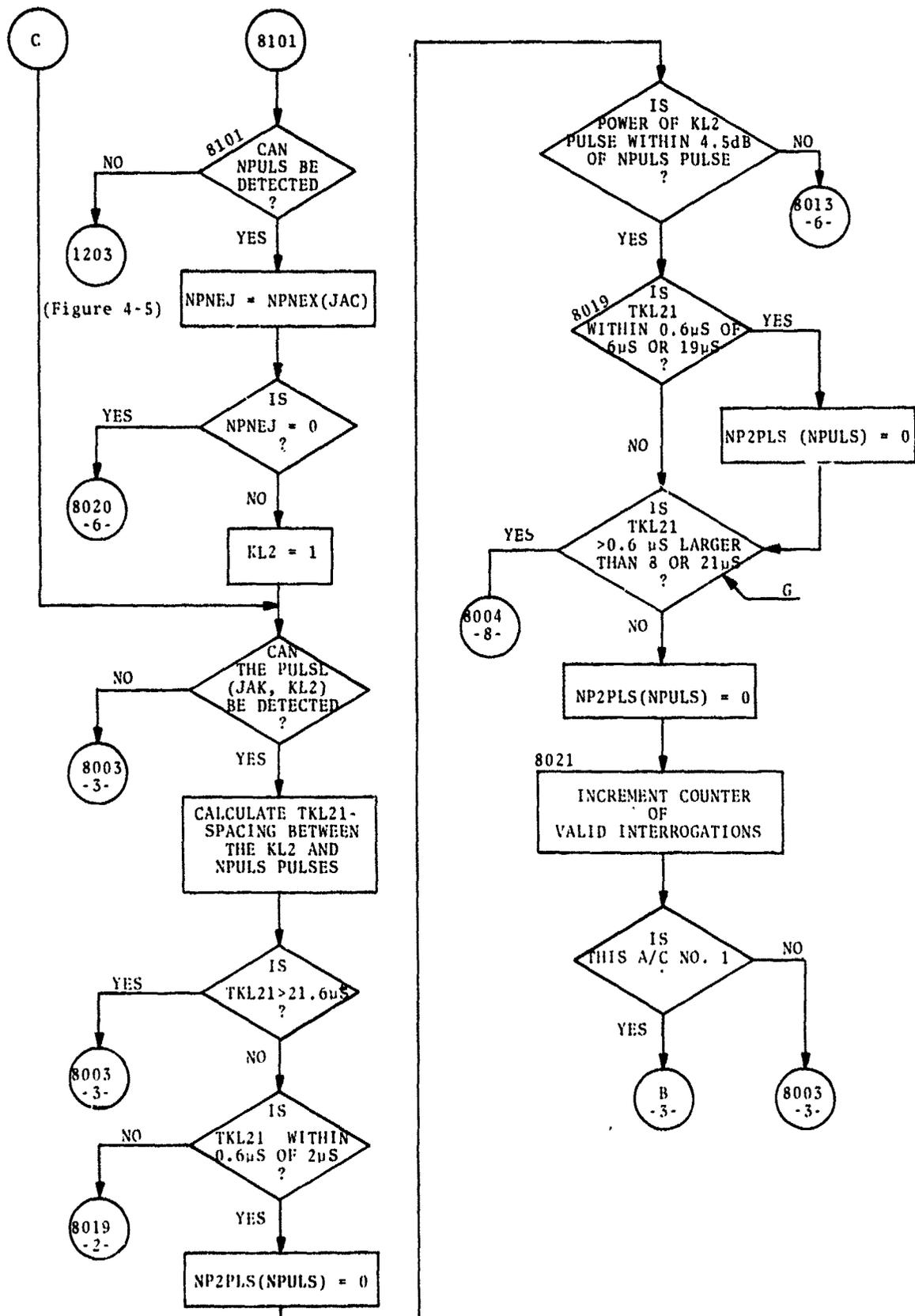
Figure 4-3. Flow Chart of ATRCBS Simulation Program Modifications Incidental to Performance of Task A (Sheet 2 of 8)
