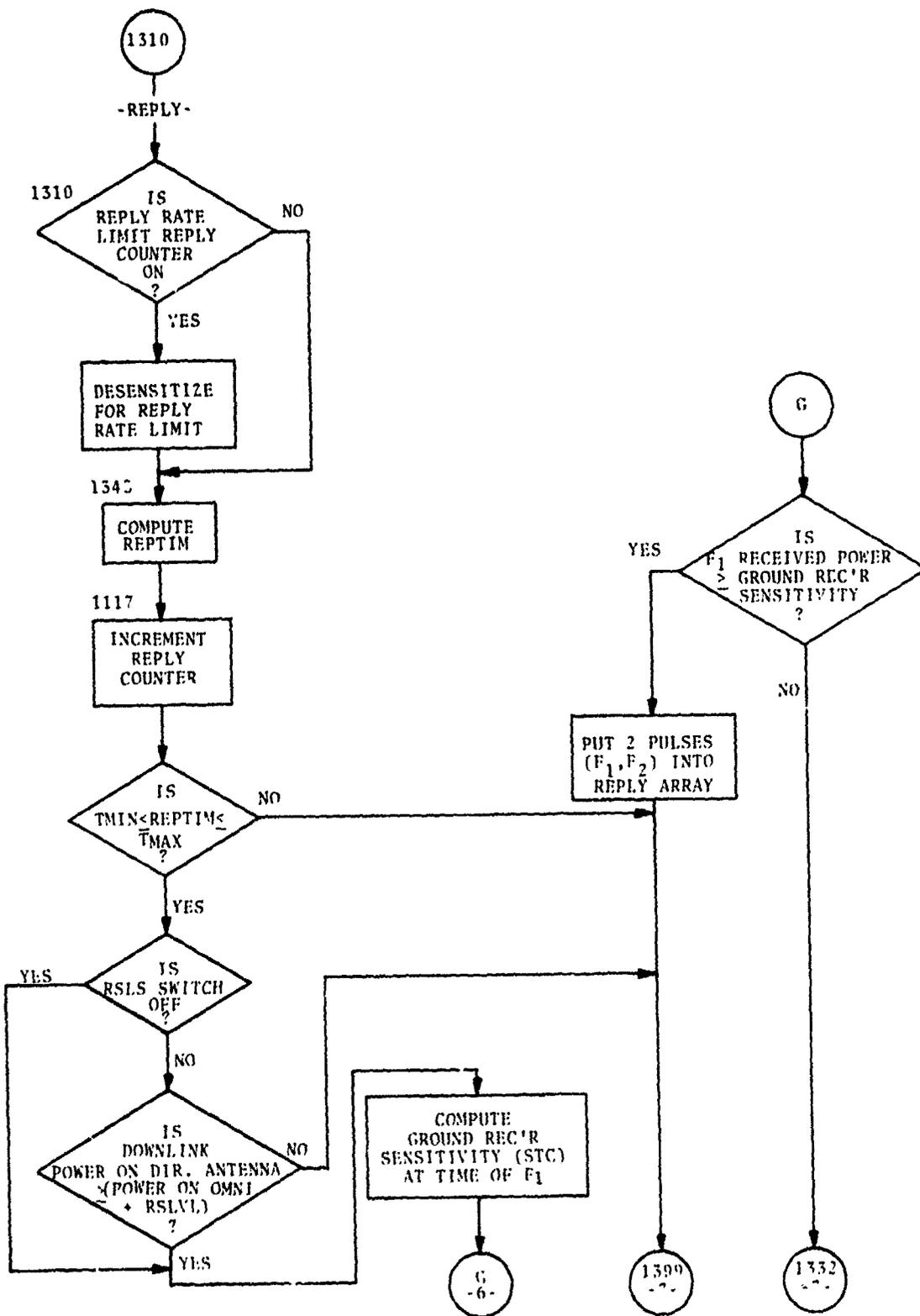
Figure 3-3. Flow Chart of ATRBS Transponder Simulation Routine (Sheet 6 of 7)
