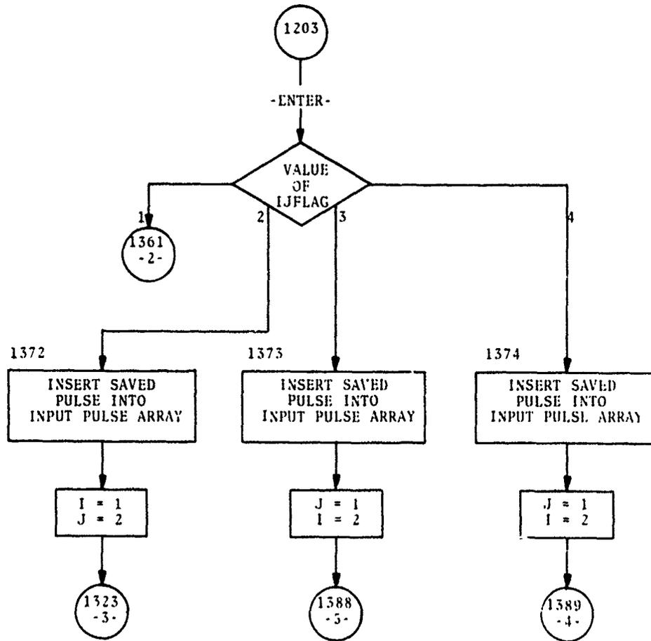
Figure 4-5. Flow Chart of ATRCBS Transponder Program Modifications to Provide DABS Operation Capability (Sheet 1 of 6)
