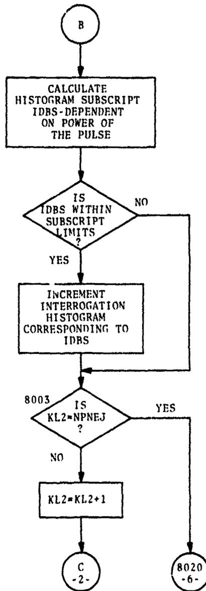
Figure 4-3. Flow Chart of ATRCBS Simulation Program Modifications Incidental to Performance of Task A (Sheet 3 of 8)
