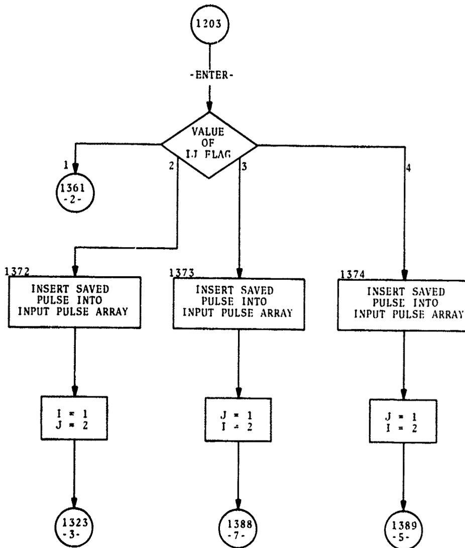
Figure 3-3. Flow Chart of ATCRBS Transponder Simulation Routine (Sheet 1 of 7)
