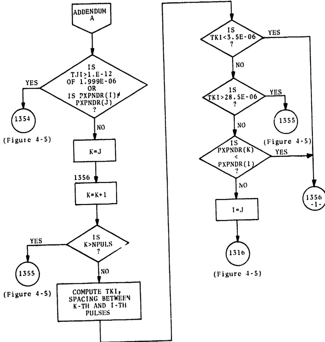
Figure 4-6. Flow Chart of Addenda to Modified ATCRBS Transponder Program (Sheet 1 of 5)
