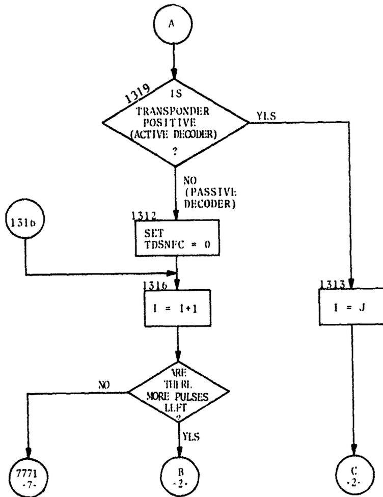
Figure 3-3. Flow Chart of ATRBS Transponder Simulation Routine
