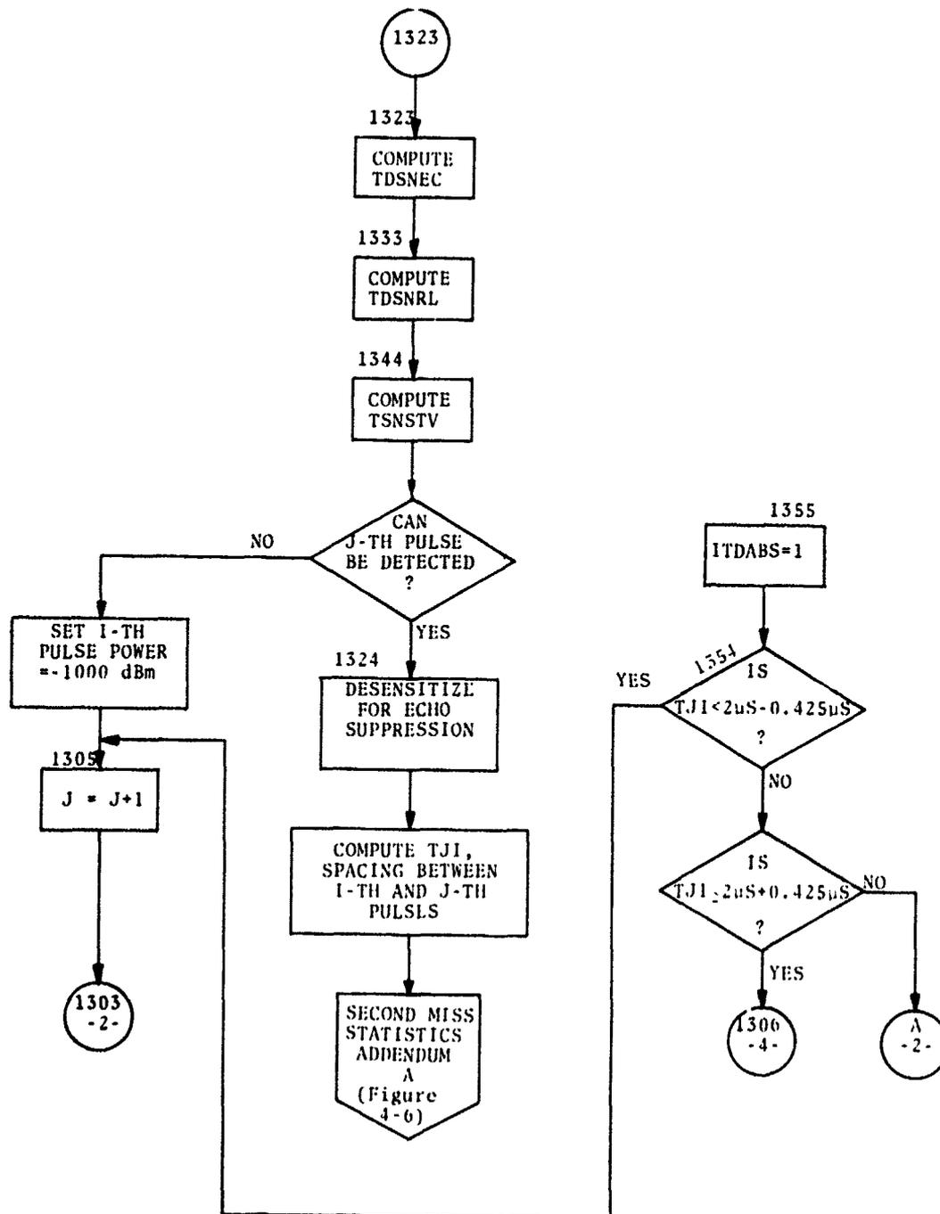
Figure 4-5. Flow Chart of ATCRBS Transponder Program Modifications to Provide DABS Operation Capability (Sheet 3 of 6)
