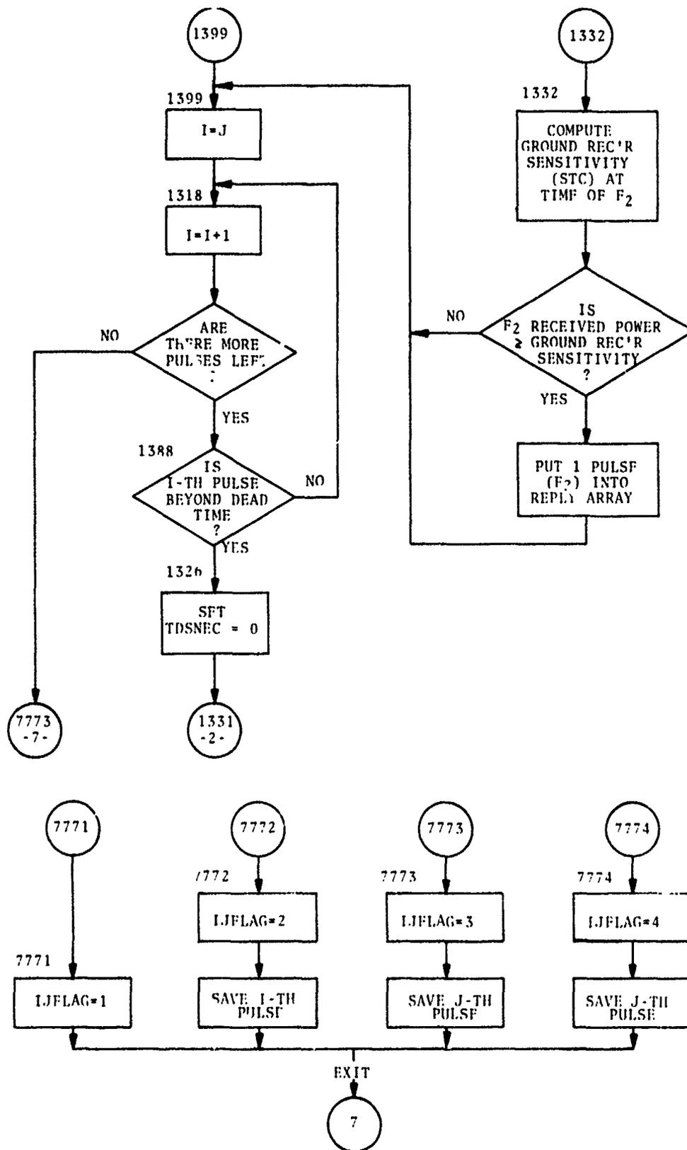
Figure 3-3. Flow Chart of ATRBS Transponder Simulation Routine (Sheet 7 of 7)
