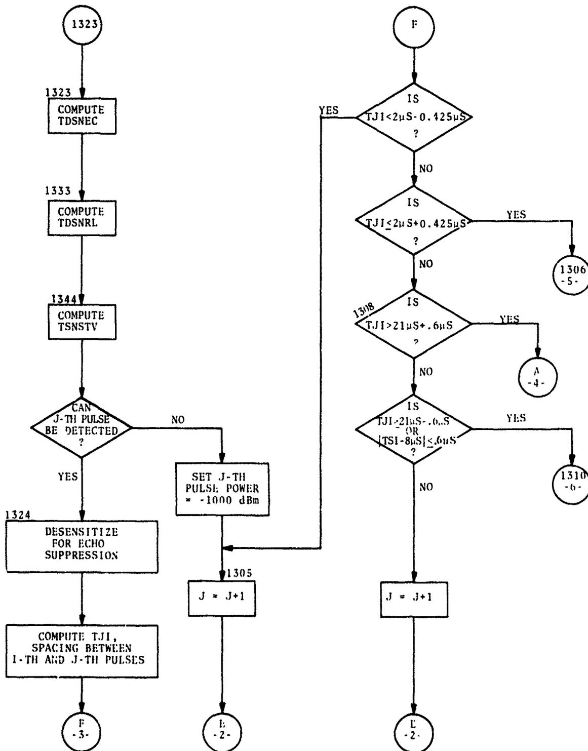
Figure 3-3. Flow Chart of ATRBS Transponder Simulation Routine (Sheet 3 of 7)
