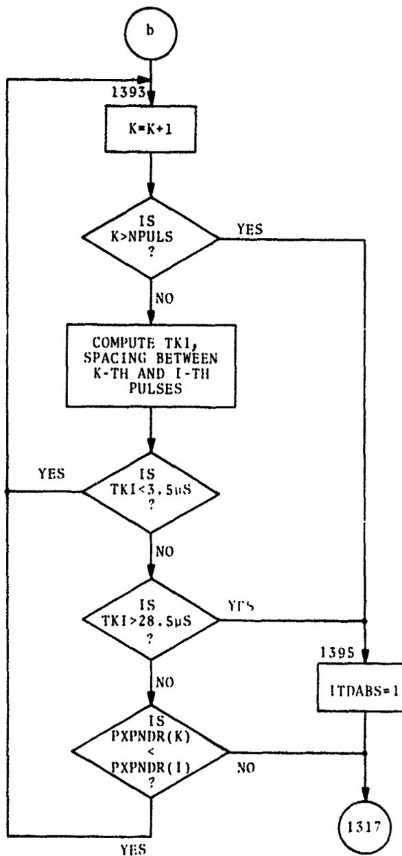
Figure 4-6. Flow Chart of Addenda to Modified ATRBS Transponder Program (Sheet 5 of 5)
