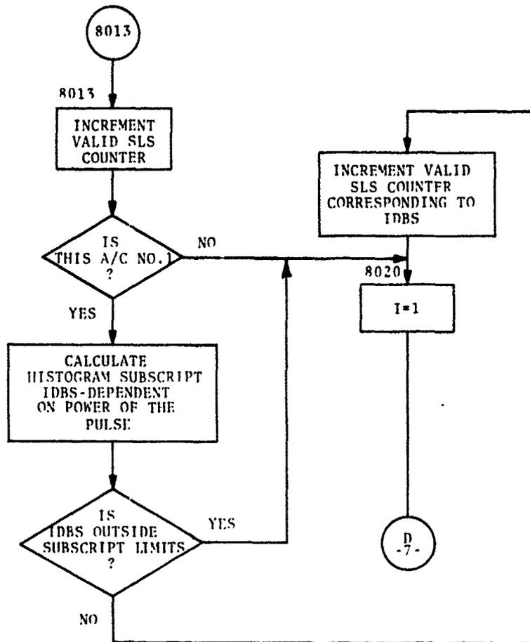
Figure 4-3. Flow Chart of ATRBS Simulation Program Modifications Incidental to Performance of Task A (Sheet 6 of 8)
