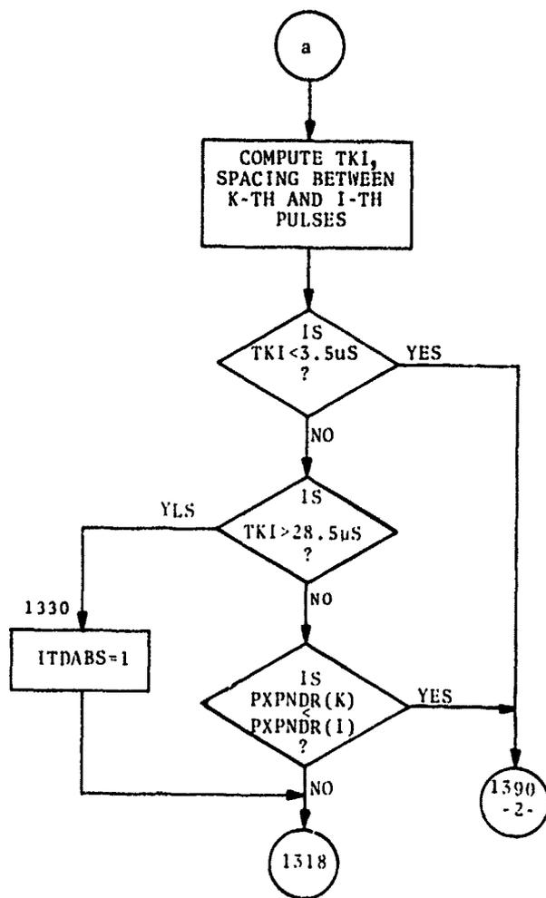
Figure 4-6. Flow Chart of Addenda to Modified ATRBS Transponder Program (Sheet 3 of 5)
