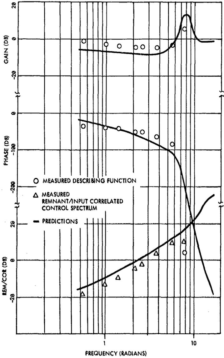
FIGURE 3-10. FREQUENCY-DOMAIN MEASURES FOR TACTILE TRACKING, 1-Axis PITCH WITH SMALLER INPUT (AVERAGE OF 4 SUBJECTS).
