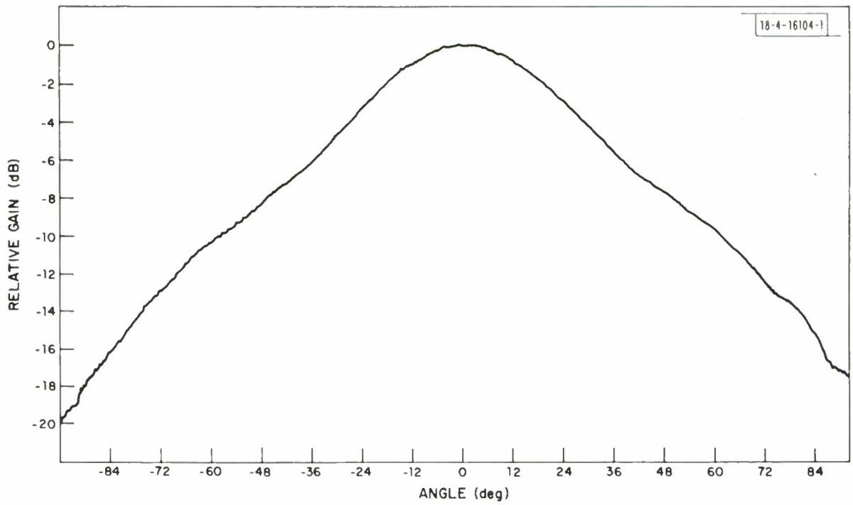
Fig. 21. Measured azimuth pattern for PALM antenna.
