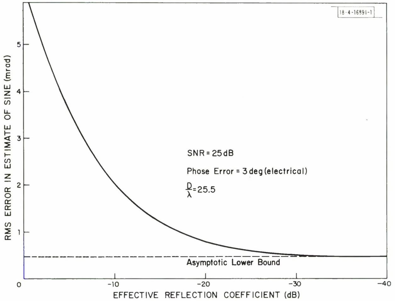
Fig. 3. Theoretical error performance of PALM interferometer.
