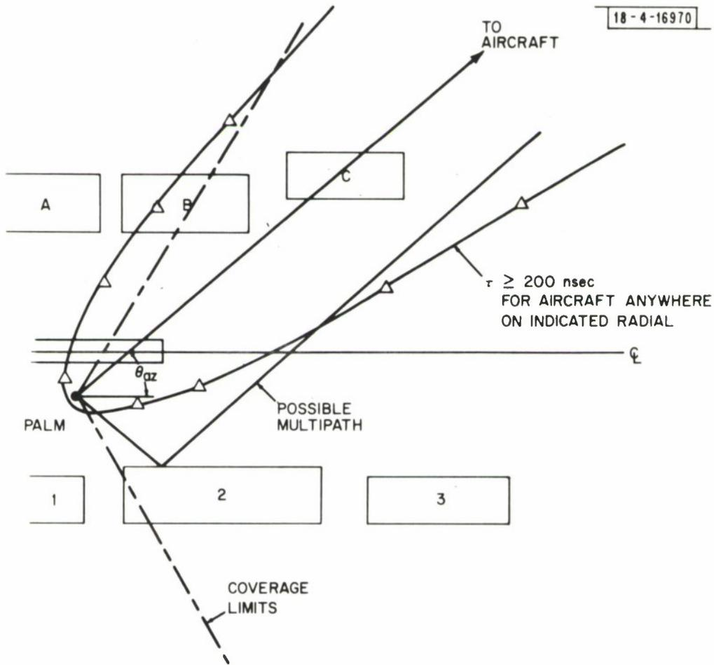
NOTE: WALLS OF BUILDINGS A-C ARE NOT ORIENTED TO YIELD MULTIPATH FOR INDICATED AZIMUTH (although they could yield shadowing.)
