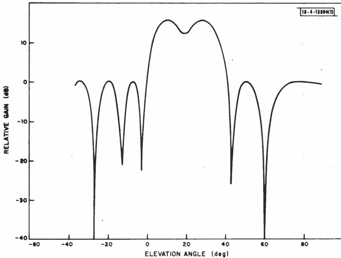
Fig. 22. Elevation pattern through azimuth boresight.
