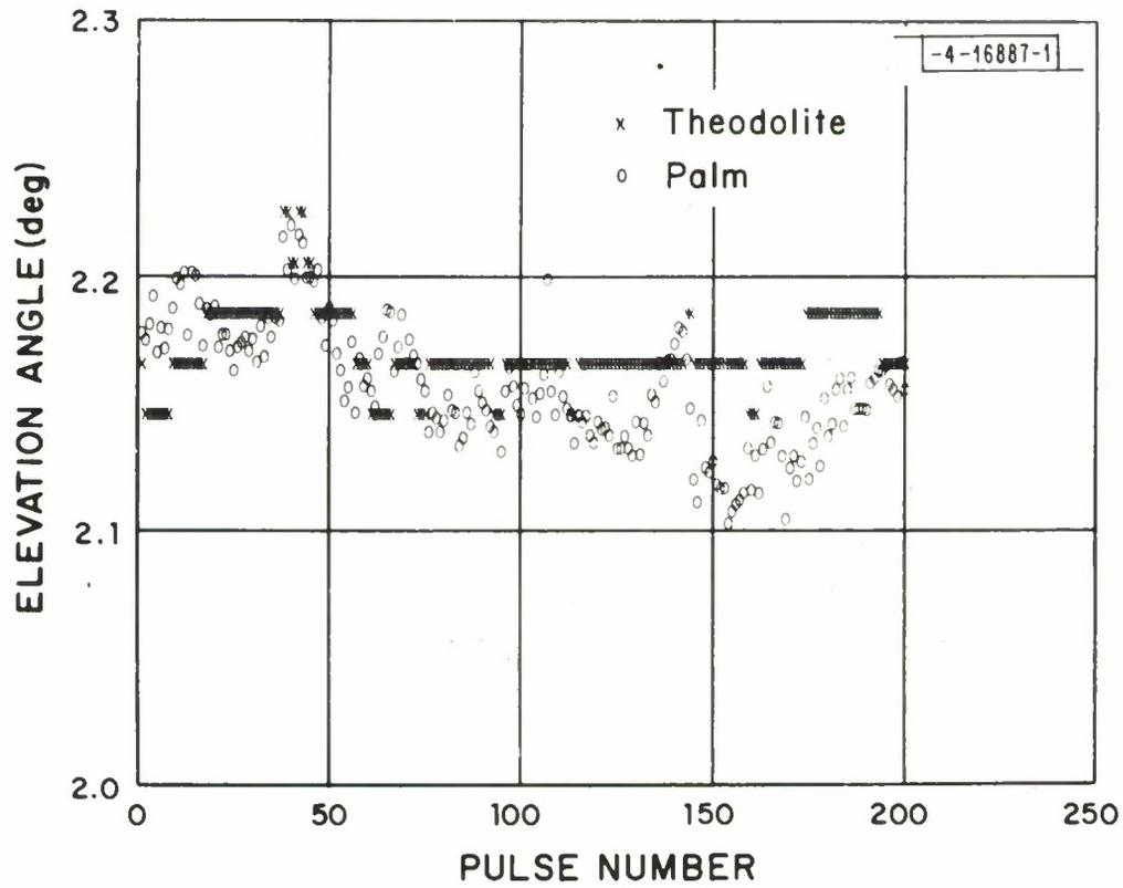
Fig. 34. Elevation angle estimates versus pulse number (time).
