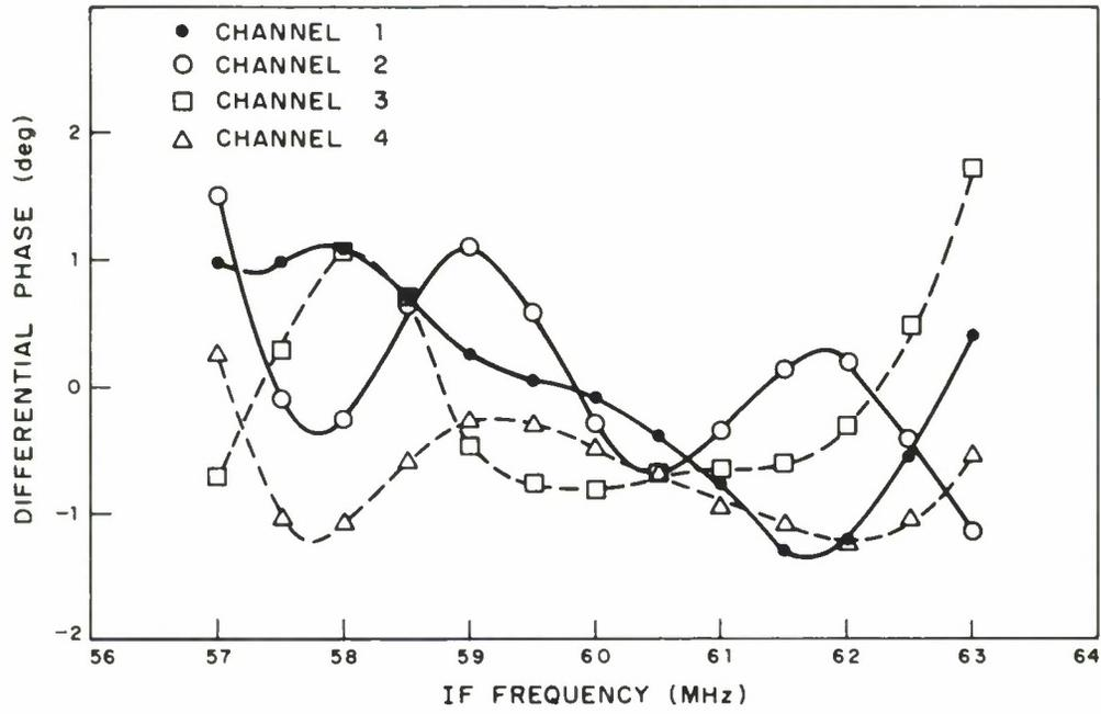
Fig. 26. Channel differential amplitude and phase response.
