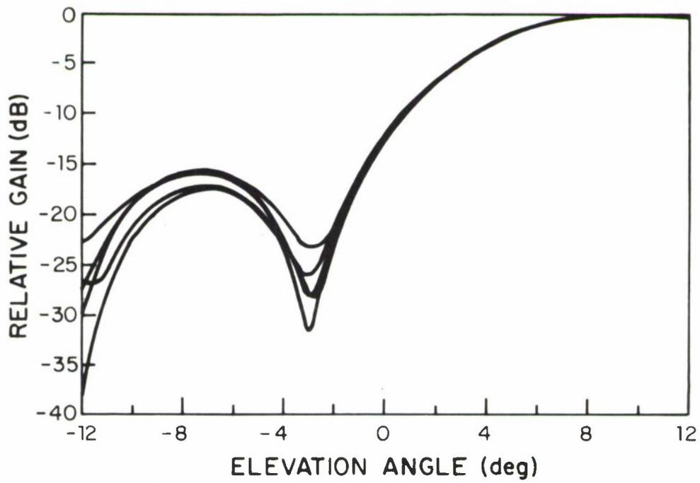
Fig. 23. Elevation patterns for the five PALM antennas.
