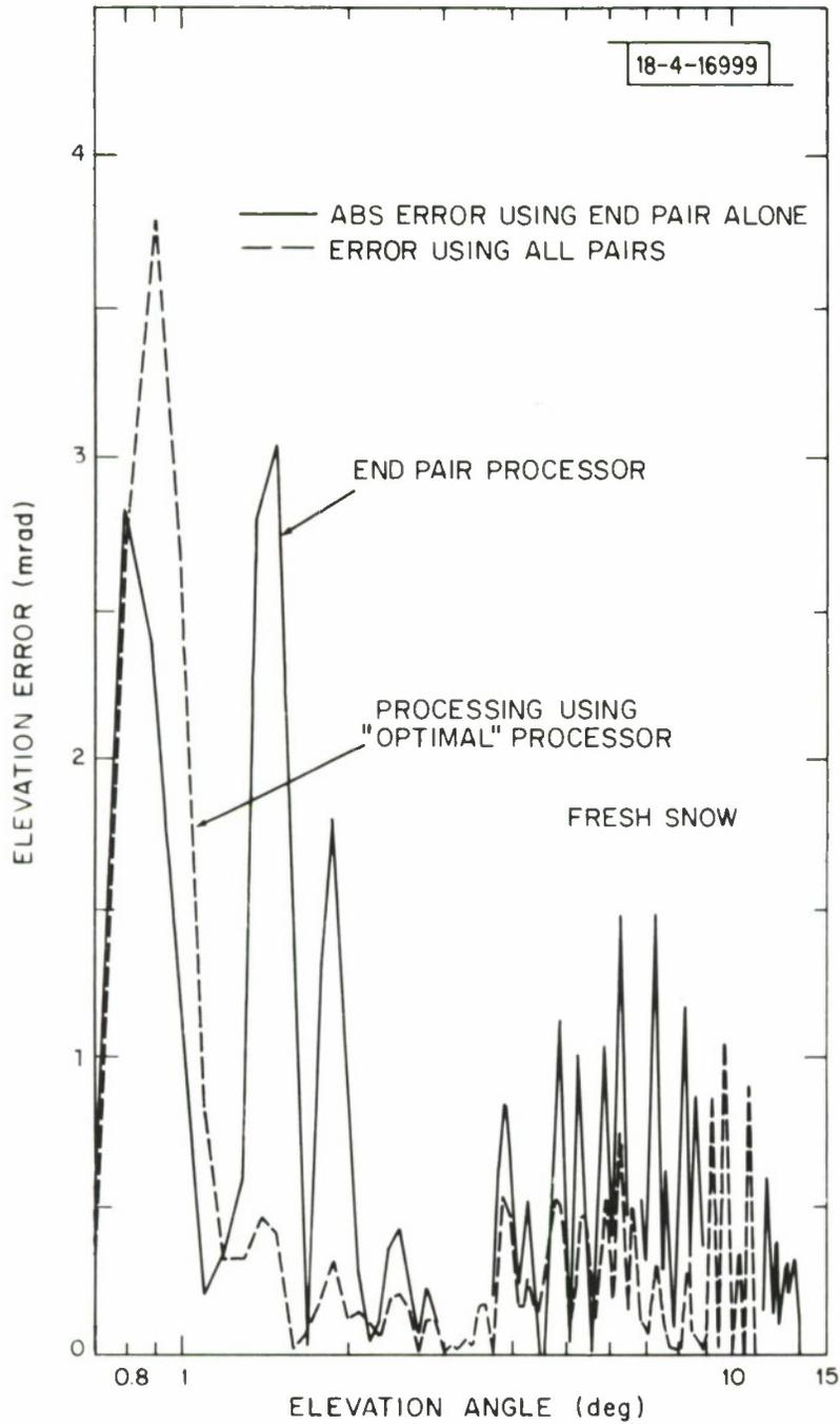
Fig. 18. Simulation of PALM error over flat, fresh snow surface.
