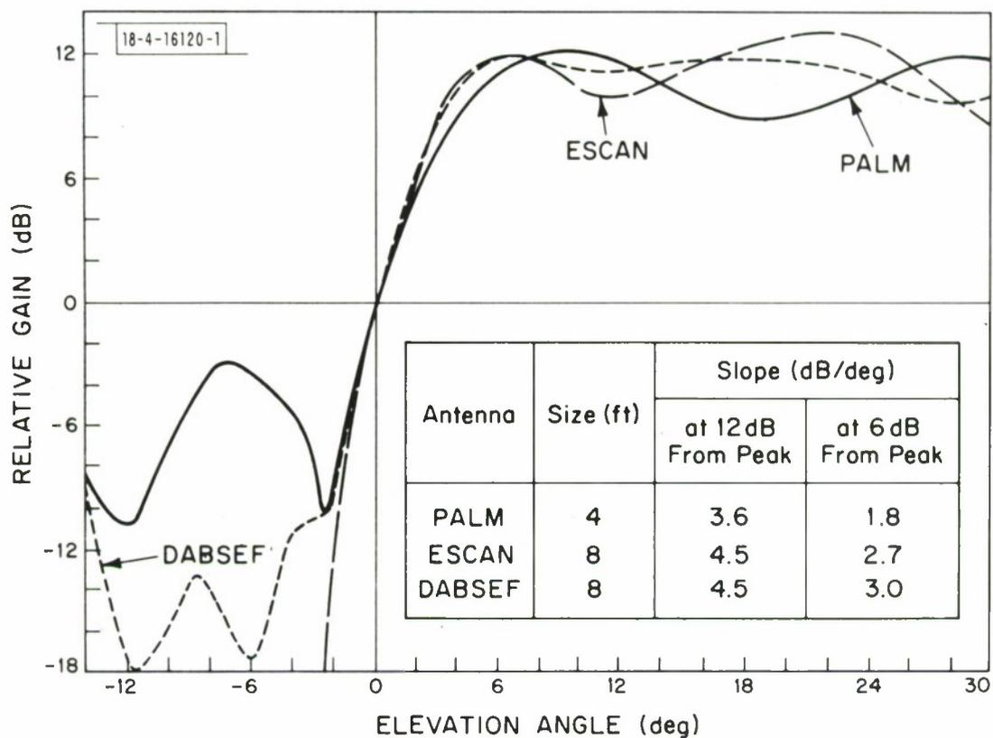
Fig. 6. Measured antenna patterns at 1090 MHz.
