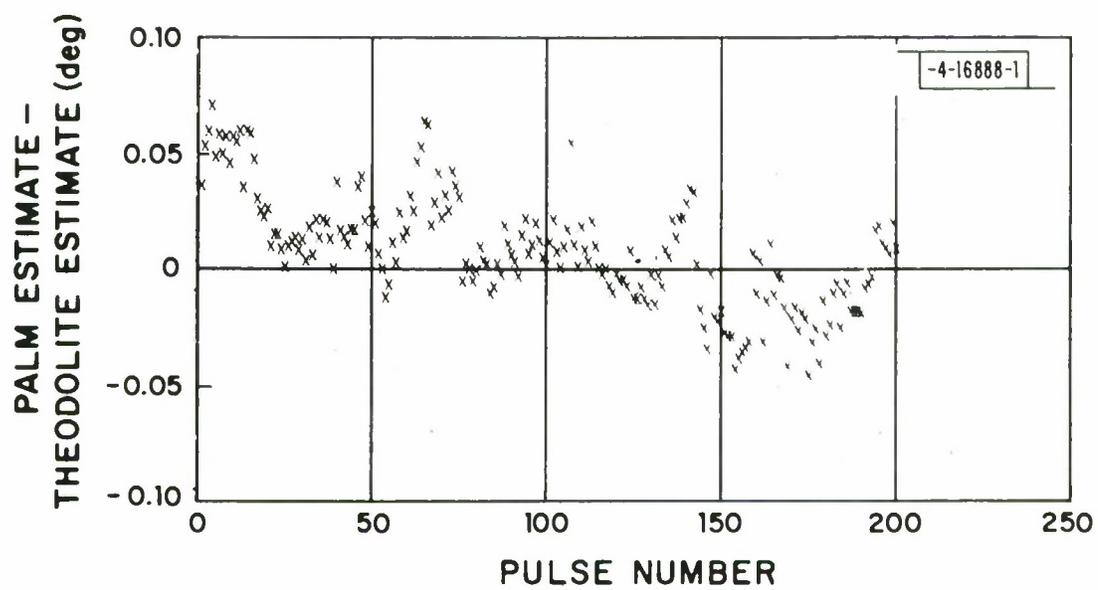
Fig. 35. PALM estimate error versus pulse number (time).
