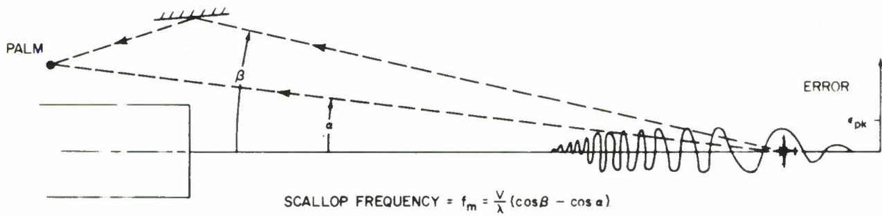
$\alpha, \beta$  ARE MEASURED WRT AIRCRAFT GROUND VELOCITY VECTOR
