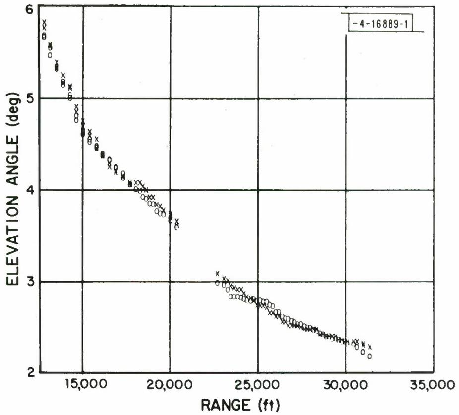
Fig. 38. Elevation angle estimates versus range (time).
