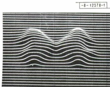
Fig. I-3. CO<sub>2</sub> laser raster scan sensitivity profile of HgCdTe quadrantal array with two of the four elements connected to 50-ohm load.
