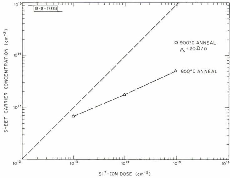
Fig. I-5. Sheet carrier concentration of GaAs layers implanted with 400-keV Si ions at room temperature through 700 Å of  $\text{Si}_3\text{N}_4$ . Straight line represents 100-percent electrical activity.
