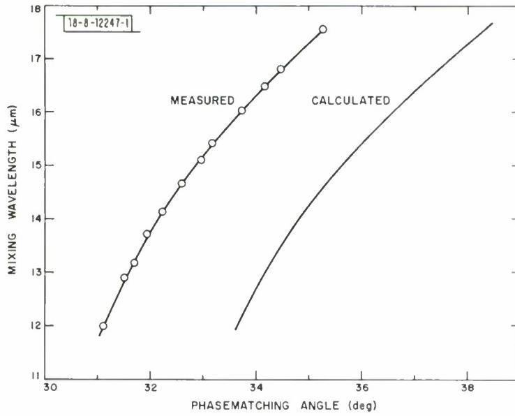
Fig. II-11. Difference mixing wavelength vs measured and calculated phase-matching angles for type I phase-matching in CdGeAs<sub>2</sub>. CO<sub>2</sub> laser is fixed at 9.59 μm, while CO laser is tuned from 5.33 to 6.20 μm.
