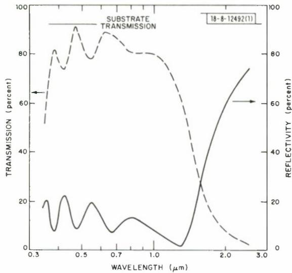
Fig. III-9. Variation of transmission and reflectivity with wavelength for Sn-doped  $\text{In}_2\text{O}_3$  films deposited by RF sputtering on glass substrate heated to  $550^\circ\text{C}$ . Structure below  $1\ \mu\text{m}$  is due to interference effects.
