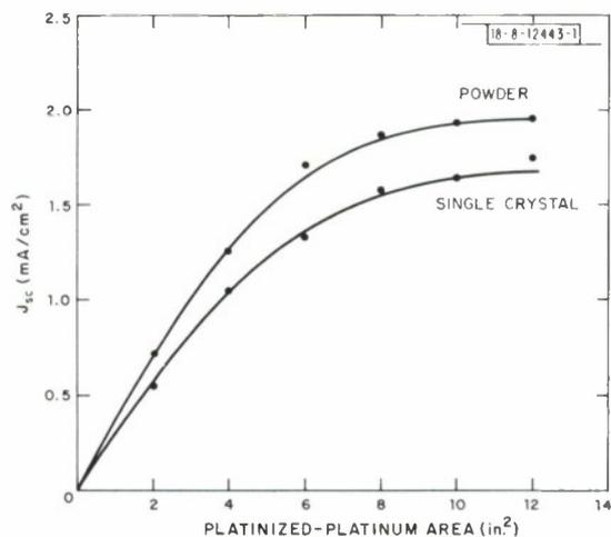
Fig. III-2. Short-circuit current density ( $J_{sc}$ ) as a function of cathode area for photoelectrolysis cell at pH = 0. Area of TiO<sub>2</sub> anode was 1 cm<sup>2</sup>.
