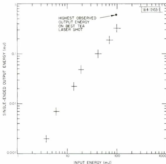
Fig. II-15. Input-output energy dependence of 10.6- $\mu\text{m}$  spin-flip laser ( $n = 1 \times 10^{16} \text{ cm}^{-3}$ ,  $l = 1.5 \text{ cm}$ ,  $T = 2 \text{ K}$ , input pulse-width  $\sim 2 \mu\text{sec}$ ,  $H = 45 \text{ kG}$ ).
