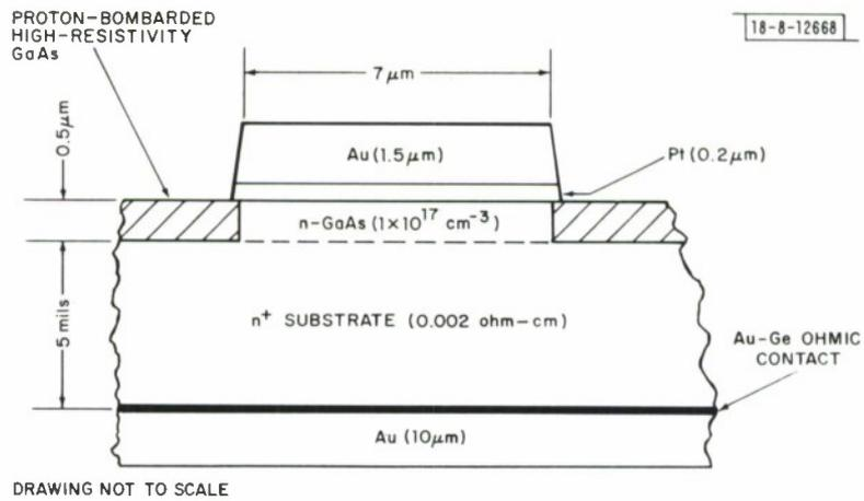
Fig. I-12. GaAs Schottky-barrier varactor diode.
