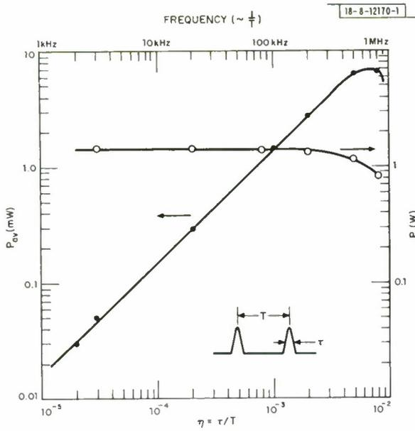
Fig. I-11. Measured peak ( $P_0$ ) and average ( $P_{av}$ ) output powers obtained using external cavity and high-duty-cycle pulser shown in Fig. I-10.
