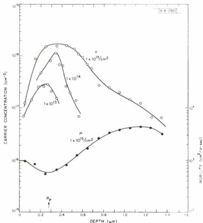
Fig. I-7. Carrier concentration and mobility vs depth measured in GaAs implanted with 400-keV Si ions at room temperature through 700 Å of Si<sub>3</sub>N<sub>4</sub> and annealed at 850°C.
