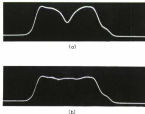
Fig. I-4. Response of HgCdTe quadrantal array to CO<sub>2</sub> laser beam scanned across center with (a) two opposite photodiodes connected, and (b) all four photodiodes connected to 50-ohm load.
