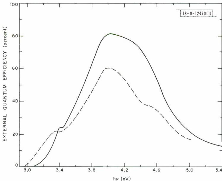
Fig. III-3. Variation of external quantum efficiency with photon energy ( $h\nu$ ) for photoelectrolysis cell with single-crystal (solid line) or hot-pressed (dashed line) TiO<sub>2</sub> anode.
