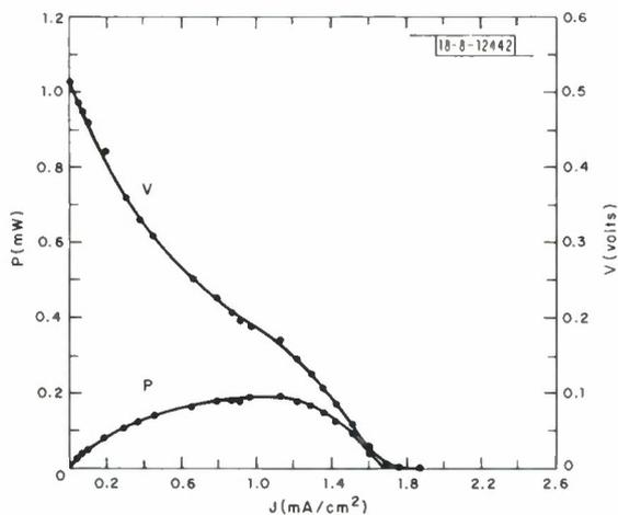
Fig. III-1. Operating characteristics of TiO<sub>2</sub>/Pt photoelectrolysis cell at pH = 0. Output voltage  $V$  and power to external load  $P$  are plotted against current density  $J$ .
