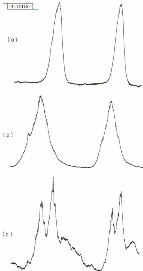
Fig. II-17. Fabry-Perot traces of spin-flip and pump laser outputs: (a)  $\text{CO}_2$  pump laser output, (b) single-mode spin-flip laser output, (c) multi-longitudinal bounce-mode spin-flip laser output.
