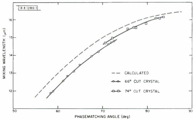
Fig. II-12. Difference mixing wavelength vs measured and calculated phase-matching angles for type I phase-matching in AgGaSe<sub>2</sub>. CO<sub>2</sub> laser is fixed at 9.57 μm, while CO laser is tuned from 5.29 to 6.01 μm.
