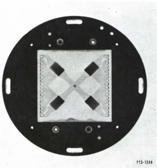
Fig. IV-1. Front view of completed VERS-11. Four 8-element silicon photodiode arrays are shown mounted on metalized aluminum substrate which is epoxied to anodized aluminum plate.
