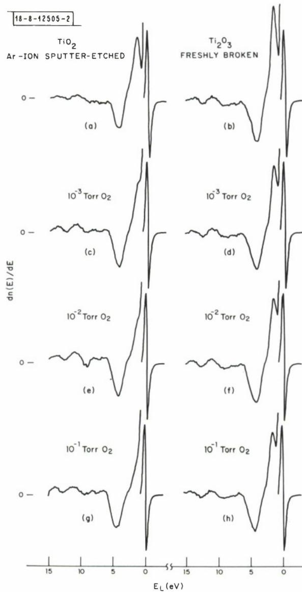
Fig. III-6. Electron energy-loss spectra,  $dn(E)/dE$  vs  $E_L$ , for  $\text{TiO}_2$  and  $\text{Ti}_2\text{O}_3$ , both before [(a) and (b)] and after [(c) through (h)] exposure for 10 minutes to  $\text{O}_2$  at pressures specified. Incident-beam energy was 30 eV.
