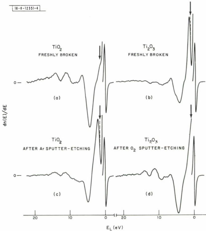
Fig. III-5. Electron energy-loss spectra,  $dn(E)/dE$  vs  $E_L$ , for (a) freshly broken  $\text{TiO}_2$ , (b) freshly broken  $\text{Ti}_2\text{O}_3$ , (c) Ar-ion sputter-etched  $\text{TiO}_2$ , and (d) O-ion sputter-etched  $\text{Ti}_2\text{O}_3$ . Arrows indicate  $E_L = 1.5$  eV. Incident-beam energy was 30 eV.
