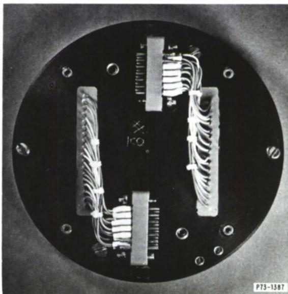
Fig. IV-2. Back view of completed VERS-11 shown in Fig. IV-1. In this view, connectors which mate with external circuitry may be seen.
