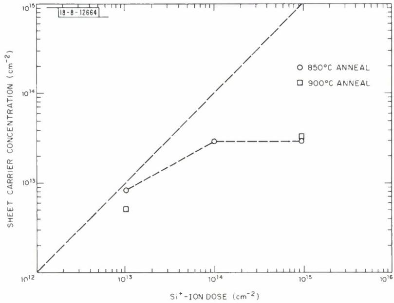
Fig. I-6. Sheet carrier concentration of GaAs layers implanted with 400-keV Si ions at 400°C through 700 Å of  $\text{Si}_3\text{N}_4$ .
