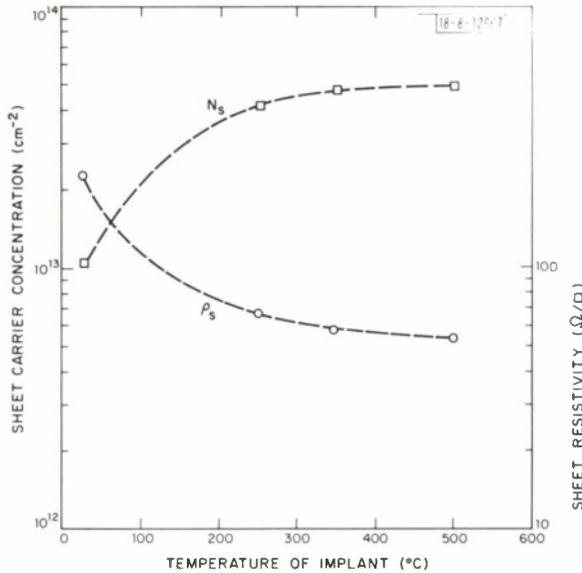
Fig. I-9. Sheet carrier concentration and sheet resistivity vs temperature of implant for 400-keV Se<sup>+</sup> ion-implanted GaAs annealed at 900 °C. Implant dose was constant at  $1 \times 10^{14} \text{ cm}^{-2}$ , and implants were made through 700 Å of Si<sub>3</sub>N<sub>4</sub>.
