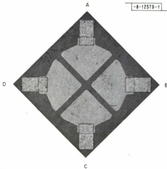
Fig. I-1. Photograph of HgCdTe quadrantal photodiode array.
