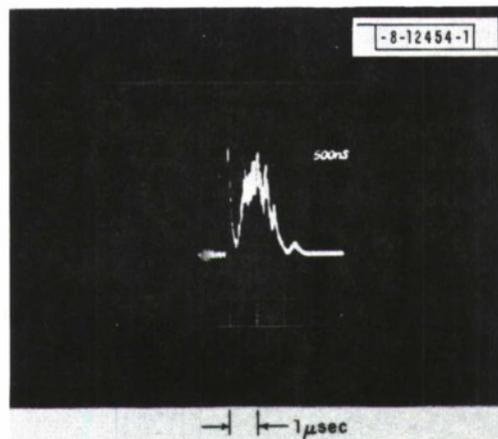
Fig. II-16. Spin-flip laser output pulse ( $n = 1 \times 10^{16} \text{ cm}^{-3}$ ,  $l = 1.5 \text{ cm}$ ,  $T = 2 \text{ K}$ , input pulsewidth  $\sim 2 \mu\text{sec}$ ,  $H = 45 \text{ kG}$ ).
