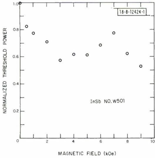
Fig. II-6. Magnetic-field dependence of CW InSb threshold.
