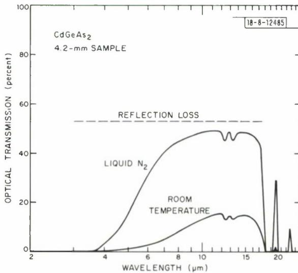
Fig. II-9. Optical transmission through 4.2-mm-thick  $\text{CdGeAs}_2$  sample.
