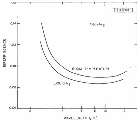
Fig. II-10. Birefringence of  $\text{CdGeAs}_2$  vs wavelength at room temperature and at liquid nitrogen temperature.
