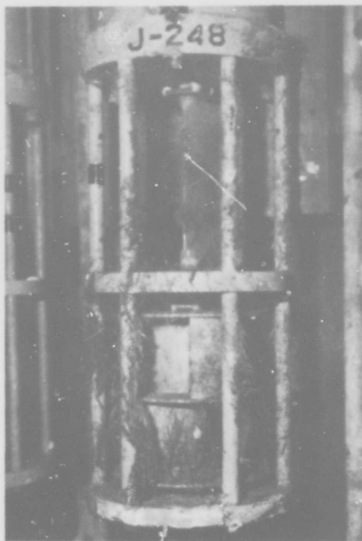
Figure 4.7.2. Rotor of current meter, showing fouling by hydroids and barnacles at depth of 50 feet.
