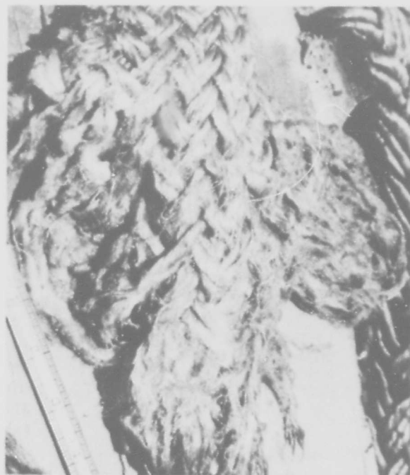
Figure 3.3.10. Lower end of parted nylon rope.
