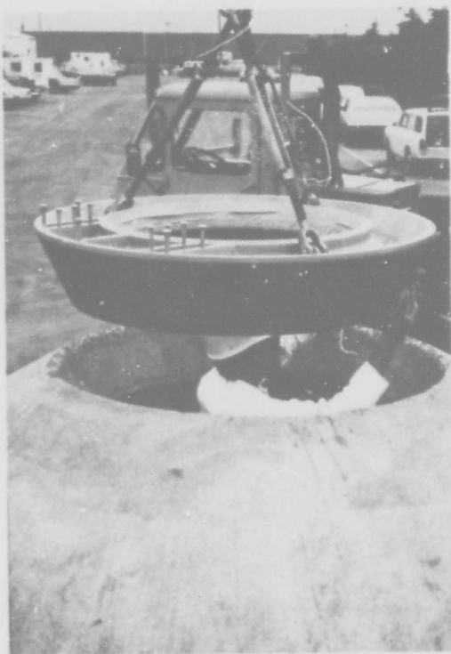
Figure 4.3.3. Hatch penetrator (top) and hull penetrator in hemisphere.
