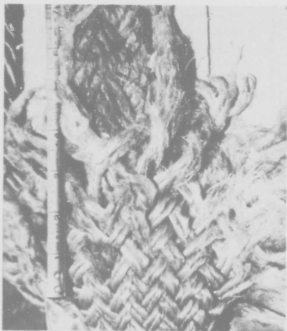
Figure 3.3.9. Upper end of parted nylon rope showing exposed core braid.
