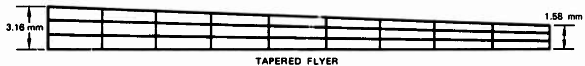
(a) 1145 ALUMINUM FLYER AND TARGET
