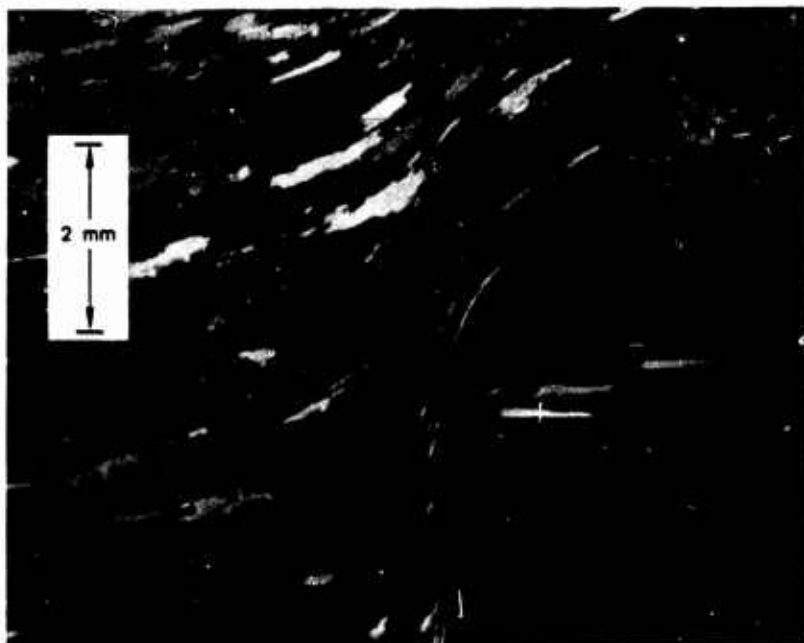
FIGURE D-1 POLISHED CROSS SECTION OF 1145 ALUMINUM PARTIALLY PENETRATED BY A ROD-LIKE PROJECTILE
